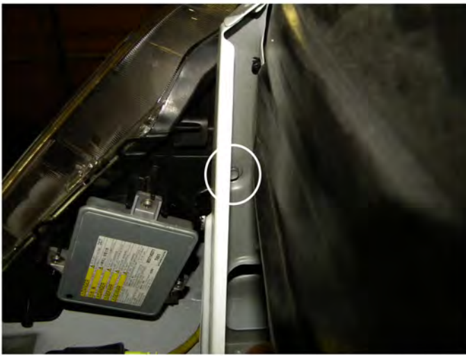
17. The location of the 10mm bolt is under the headlight housing
