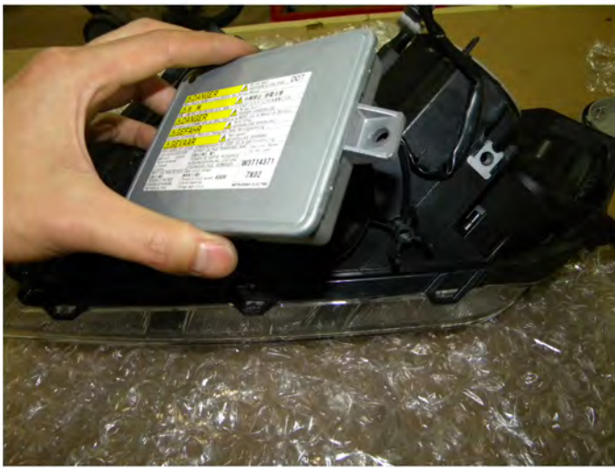
23. Remove the ballast from housing
