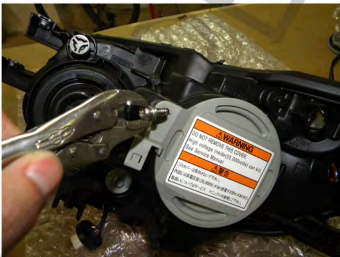
27. Remove security screw that is securing lightbulb to access the hole cover
