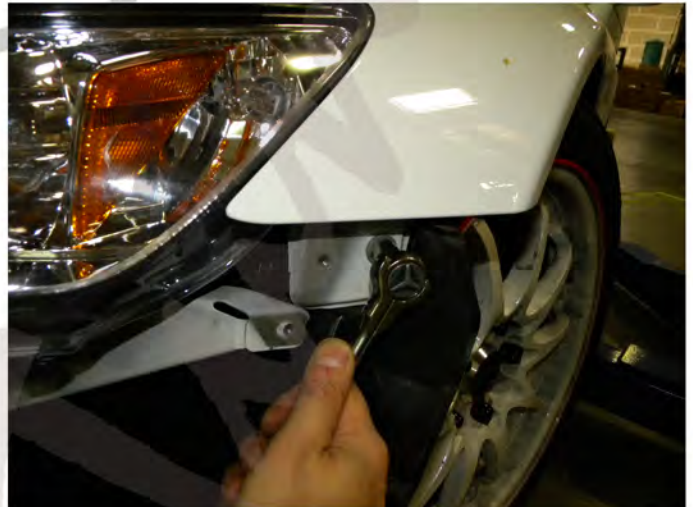
56. Replace and tighten 10mm bolts to the side of the housing
