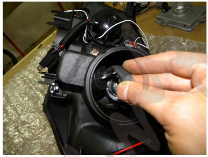
42. Run the cable or harness through the housing
