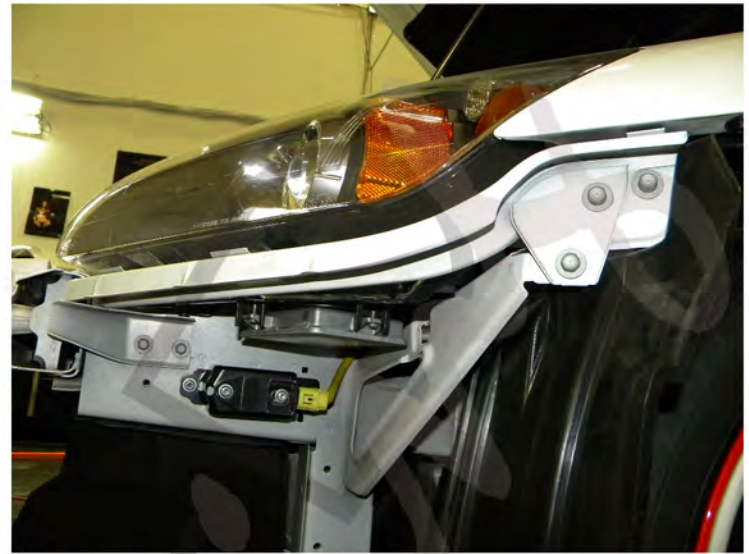
12. Bracket bolt locations (4 bolts)
