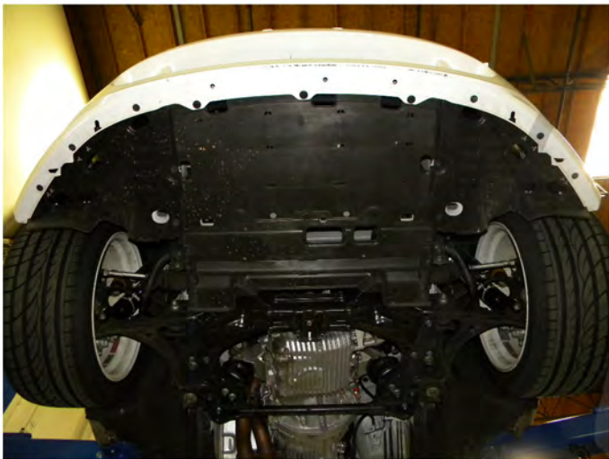
67. Replace the (3) clips and the (6) 10mm bolts located on the bottom of the front bumper
