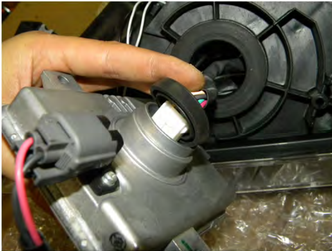
49. Reconnect the ballast and replace the rubber cover
