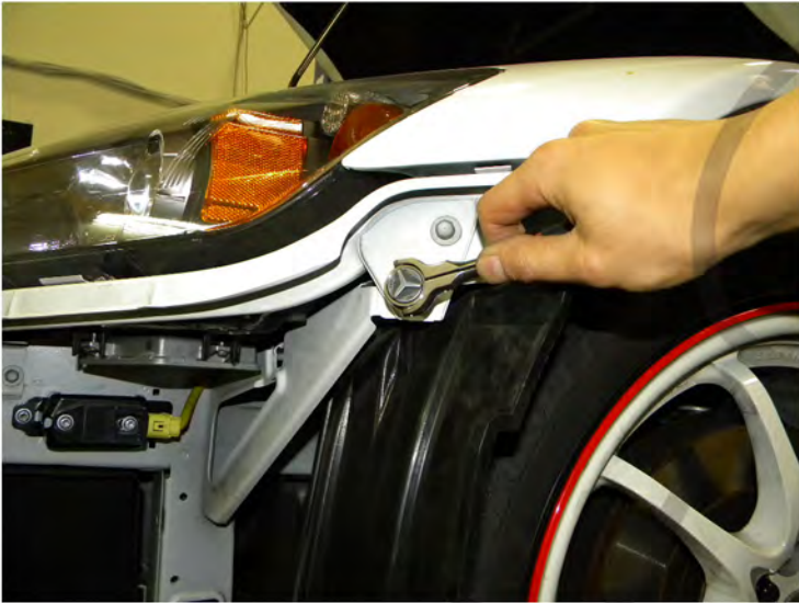
13. Unscrew the 10mm bolt
