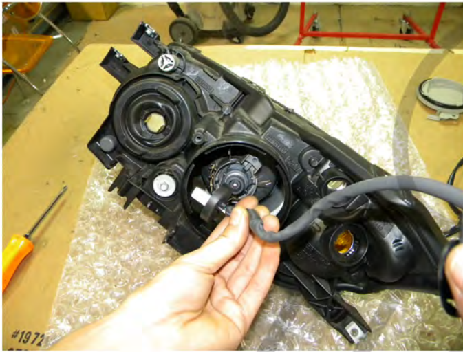
31. Remove the cable from its housing
