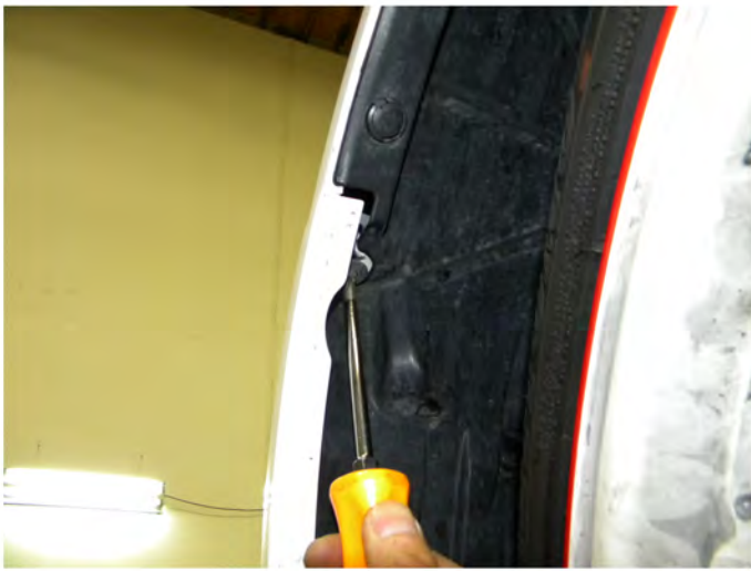
65. Replace and tighten phillip head screw in the wheelwell
