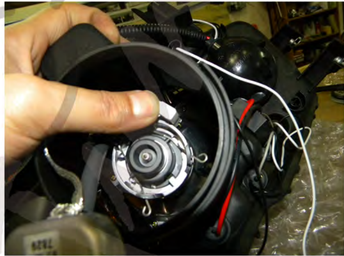
44. Connect the ground connector onto the cable or harness
