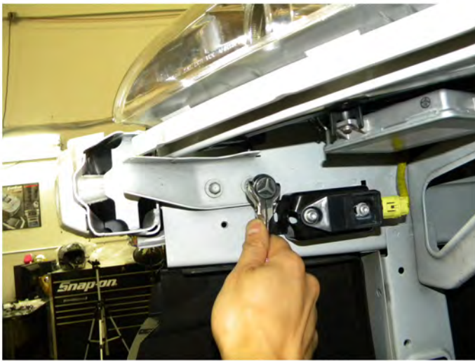
59. Replace bracket under the headlight and tighten (4) 10mm bolts
