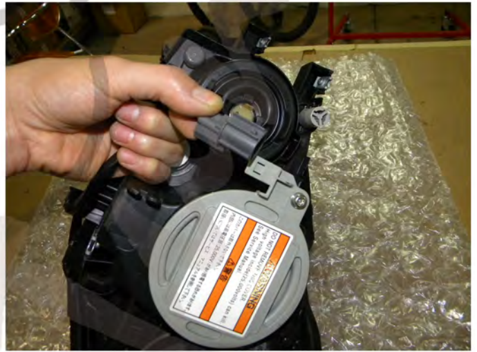
26. Unclip the connector
