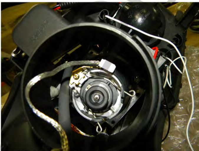
39. Connect the ground connector onto the cable or harness
