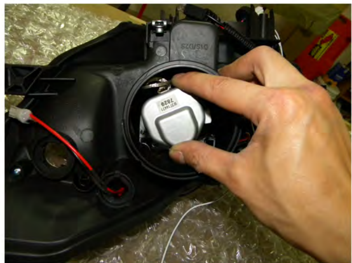
46. Reattach the harness to the HID bulb
