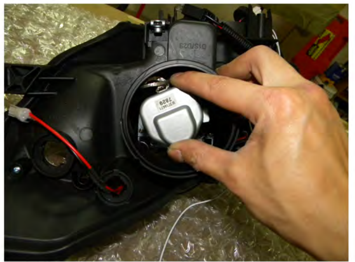
40. Reattach the harness to the HID bulb
