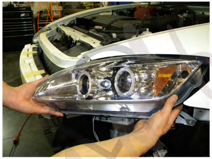
54. Place the new light into the proper location
