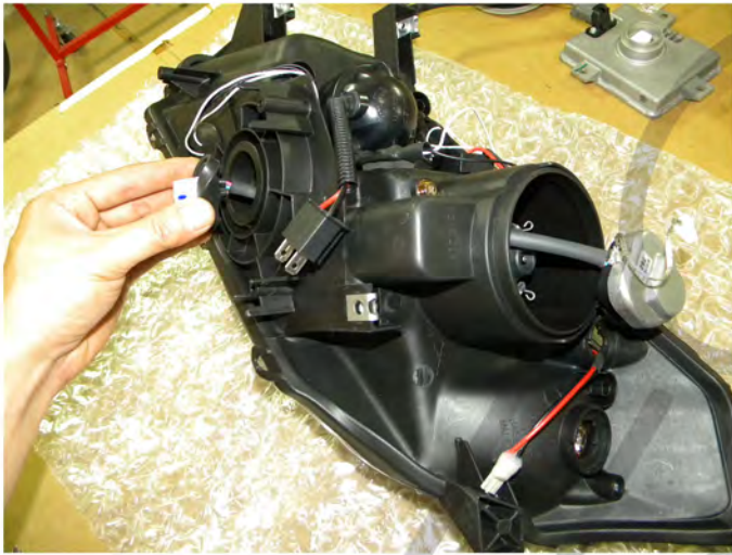
43. Run the cable through the inside of the housing
