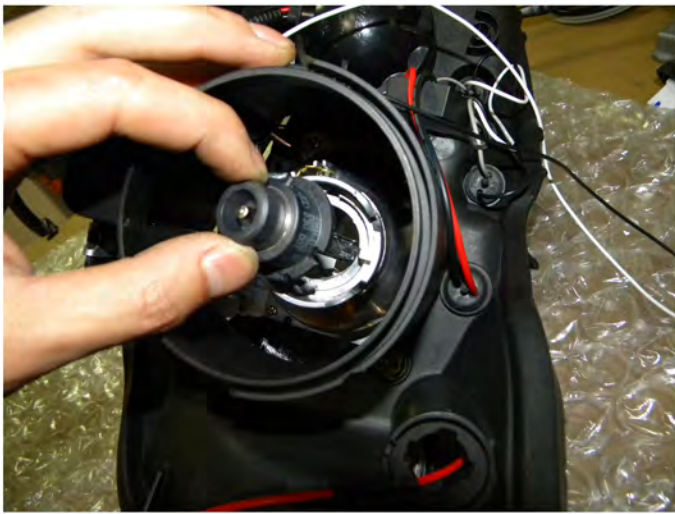
35. Place and secure the HID bulb inside the housing
