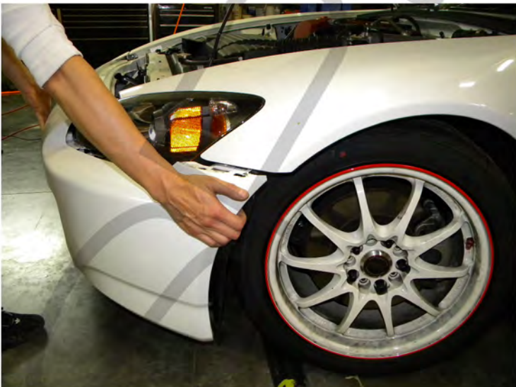
9. Unlatch the sides of bumper
