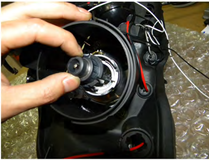
41. Place and secure the HID bulb inside the housing
