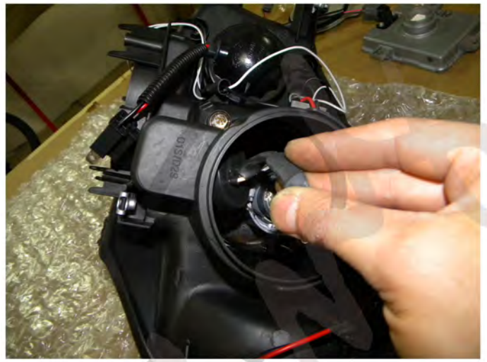
36. Run the cable or harness through the housing
