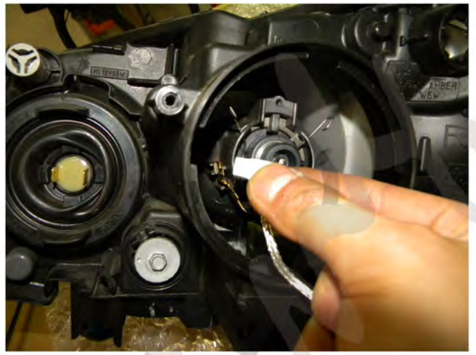
30. Unplug the ground connection
