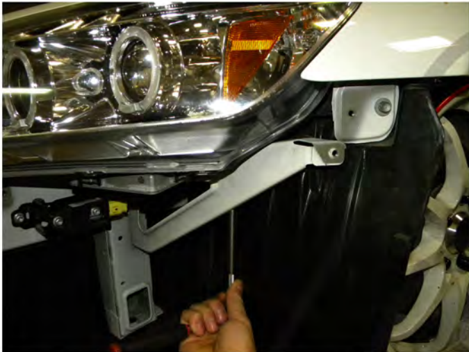
55. Replace and tighten 10mm bolts located underneath the headlight housing
