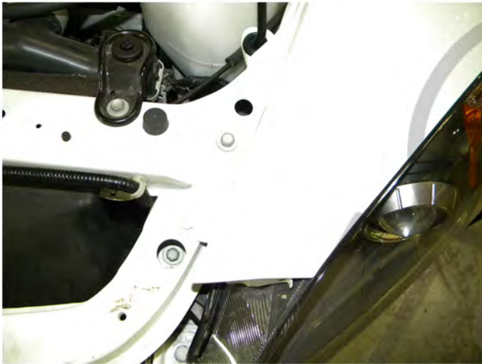
19. Remove (2) 10mm bolts located toward the top side of the headlight
