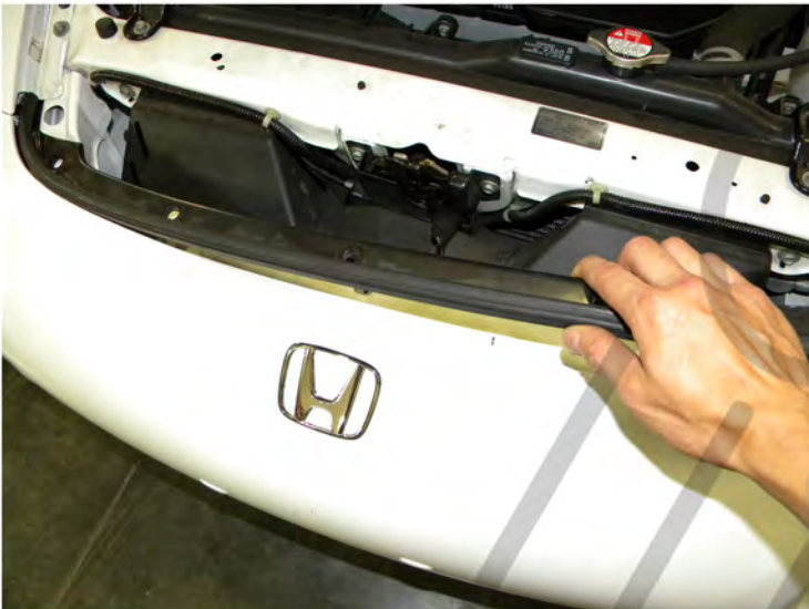
7. Remove the bracket
