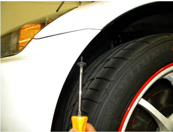
5. Remove the phillip head screw
