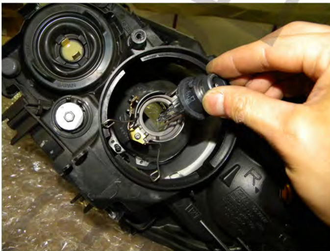
33. Remove the HID bulb
