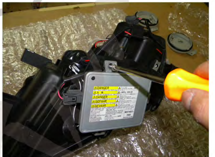
50. Secure the ballast onto the housing ( 3 phillips head screws)
