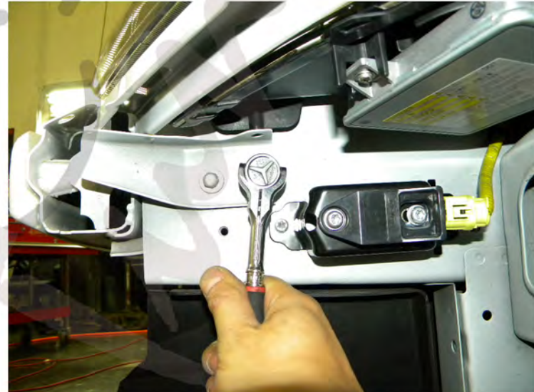
14. Unscrew the 10mm bolt
