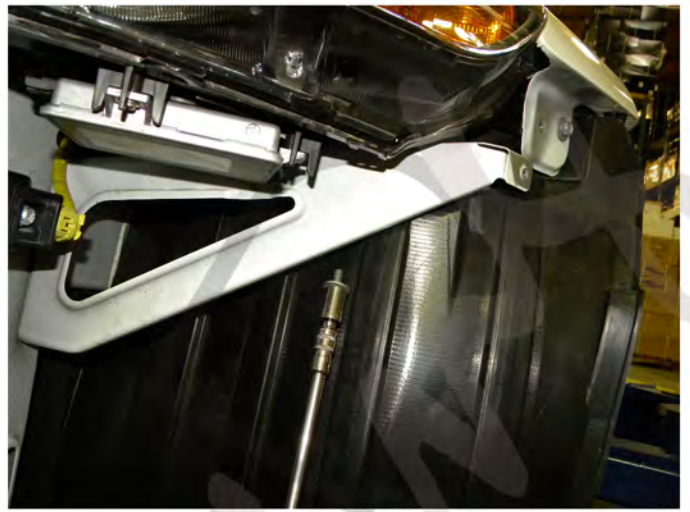
18. Remove the 10mm bolt located under the headlight housing
