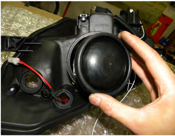
47. Replace the rubber cover
