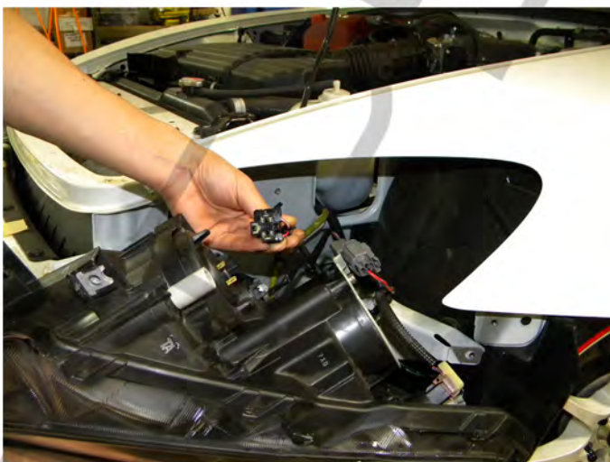
21. Remove all wiring harnesses and sockets from the headlight housing
