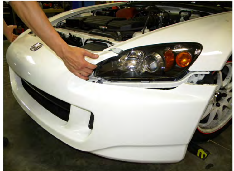
10. Remove the front bumper
