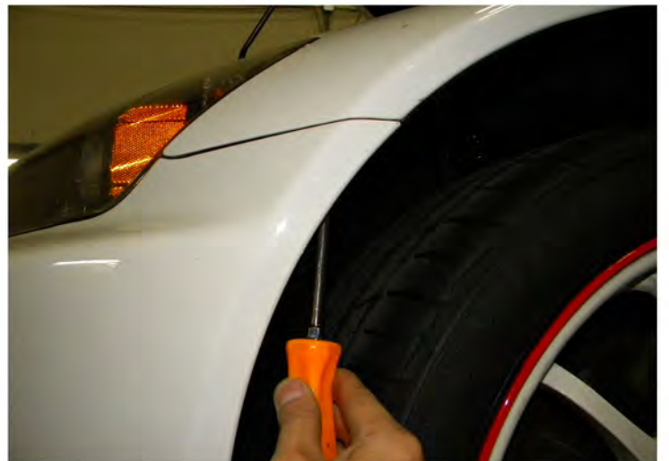
4. Remove the phillips head screw from the wheel well
