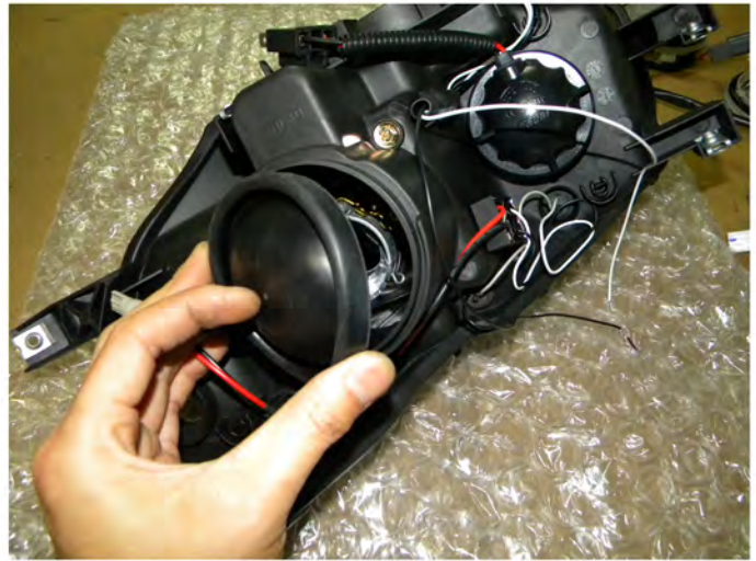
34. Remove the rubber cover
