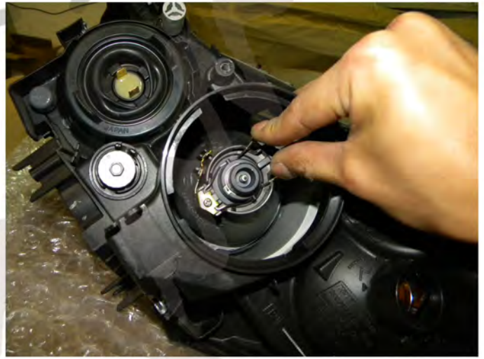
32. Remove the HID bulb
