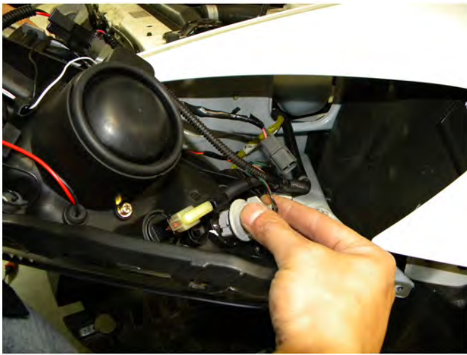
53. Reconnect all harnesses and sockets onto the new headlight
