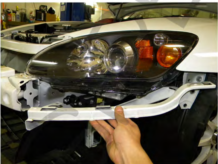
15. Remove the bracket
