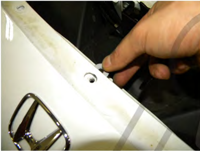
61. Replace (5) washers located under the top mounting points of the bumper
