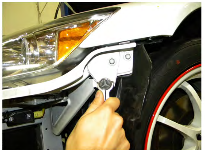
58. Replace bracket under the headlight and tighten (4) 10mm bolts
