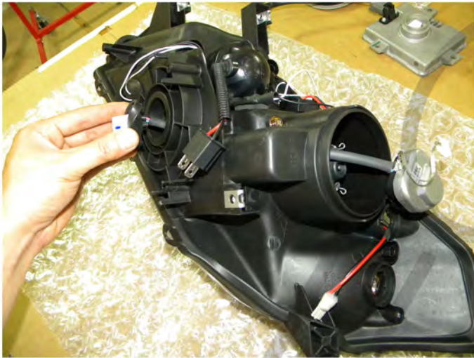
37. Run the cable through the inside of the housing
