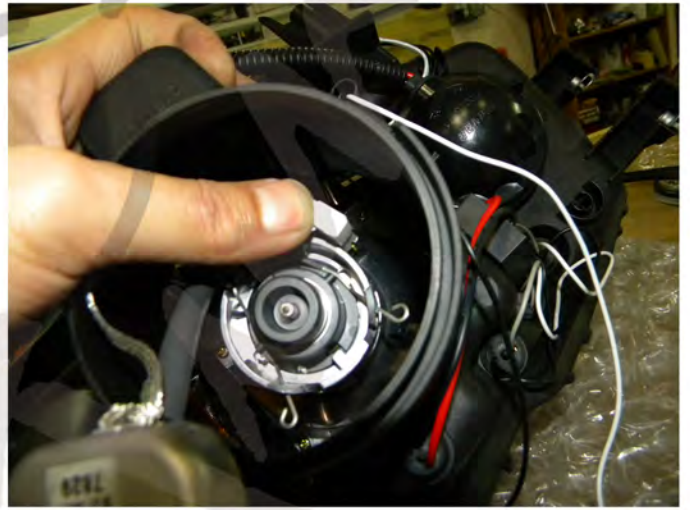
38. Connect the ground connector onto the cable or harness
