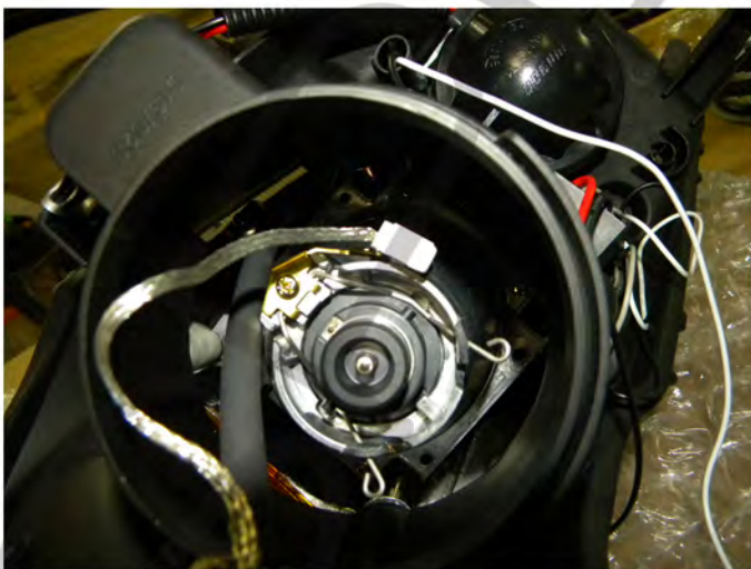
45. Connect the ground connector onto the cable or harness
