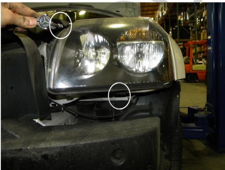
9. Install two 8mm headlight bolts
