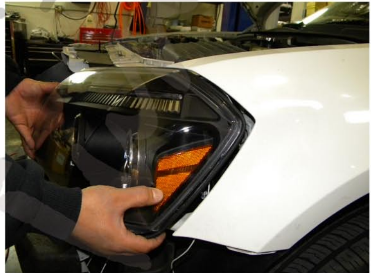
8. Install the new projector headlight
