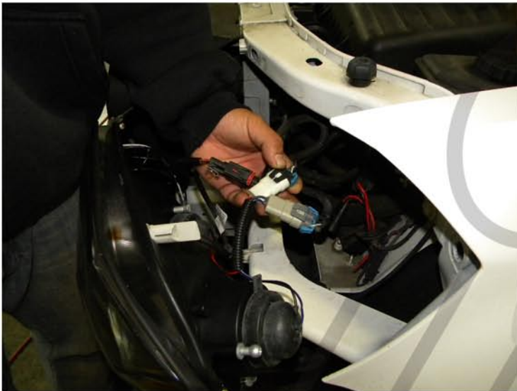
7. Disconnect all the connectors from the headlight
