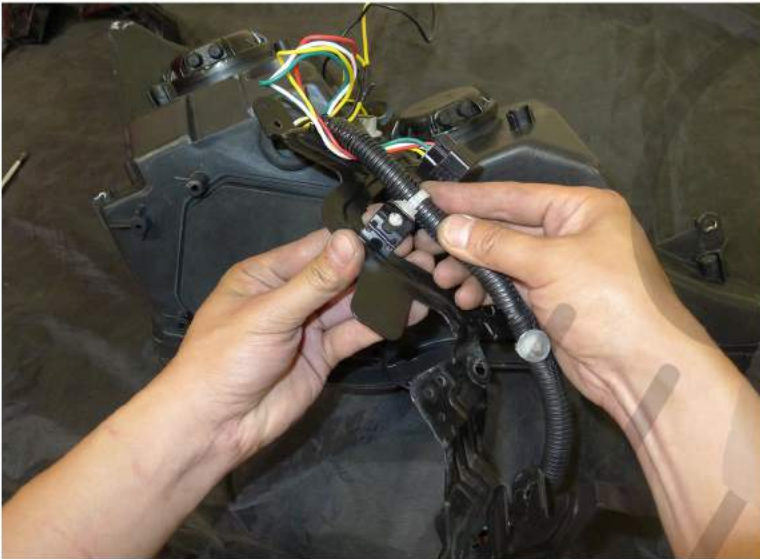
43. Attach the new projector headlight harness to the metal bracket
