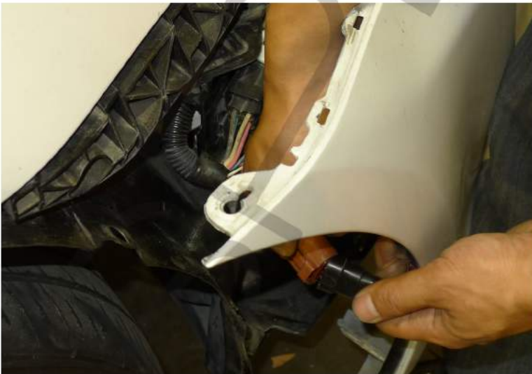
15. Disconnect the fog light harness
