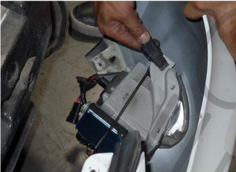
55. Connect the wire harness
