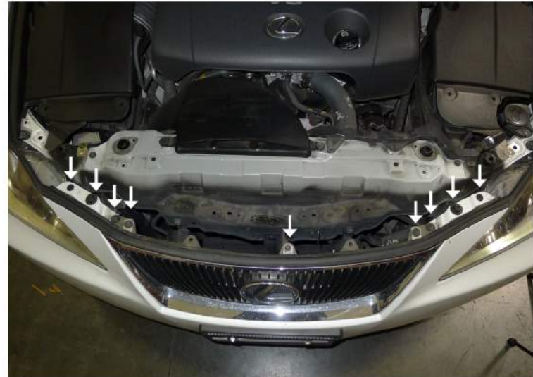
10. (6) plastic clips, (2) Phillips head screws, and 10mm bolt location
