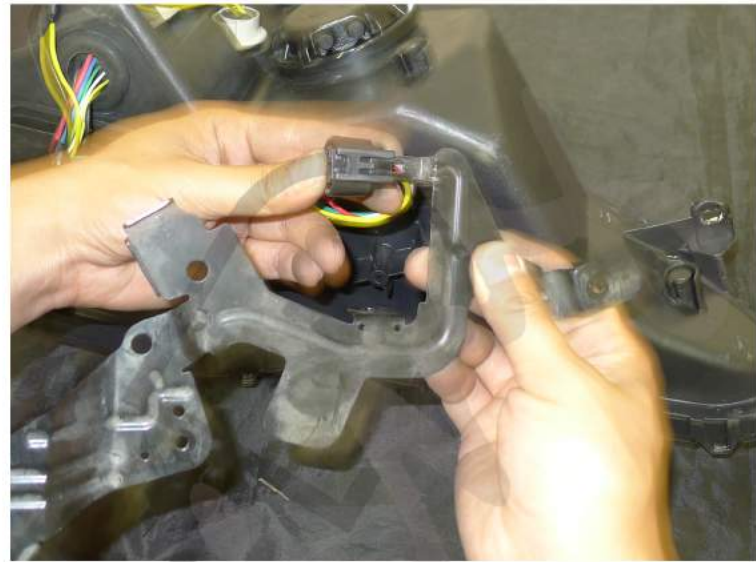
42. Attach the new projector headlight harness to the metal bracket
