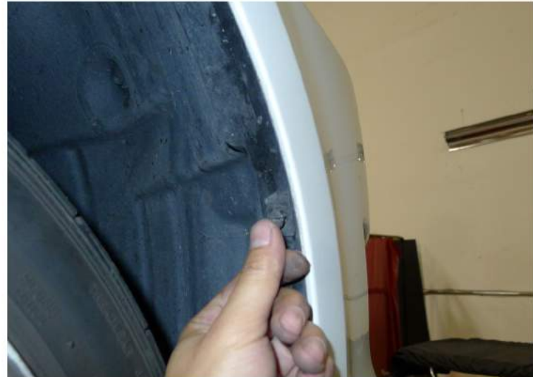
64. Replace the 2 plastic clips
