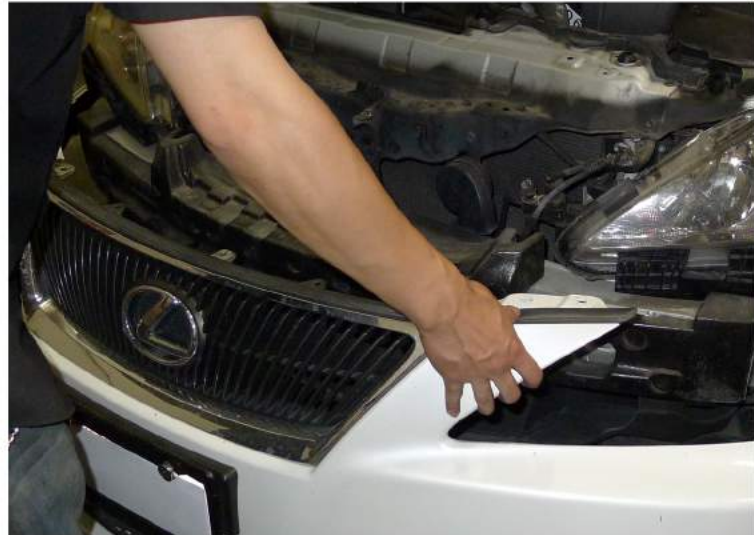
16. Remove the front bumper
