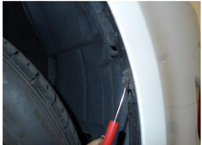
4. Remove the (2) plastic clips
