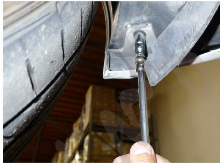
66. Tighten the (9) 10mm bolts
