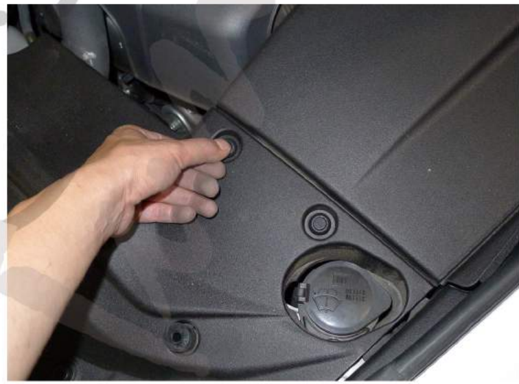
62. Replace the (11) plastic clips
