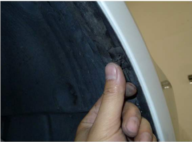
65. Replace the (2) plastic clips
