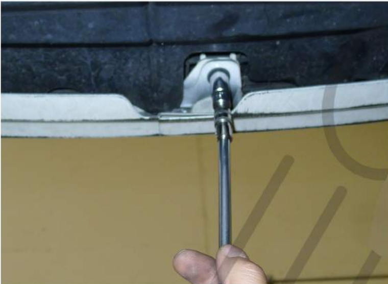
67. Tighten the (9) 10mm bolt Please repeat the steps from 1 to 67 for the opposite side
