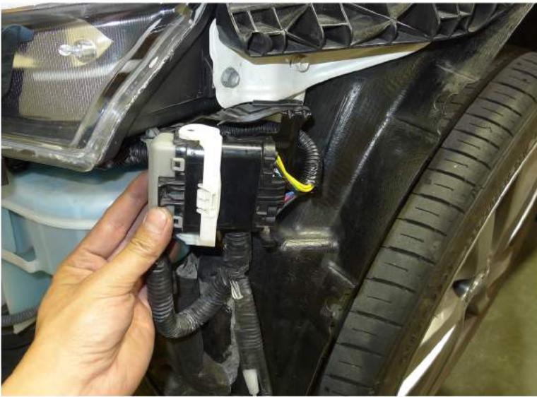
53. Connect the headlight harness
