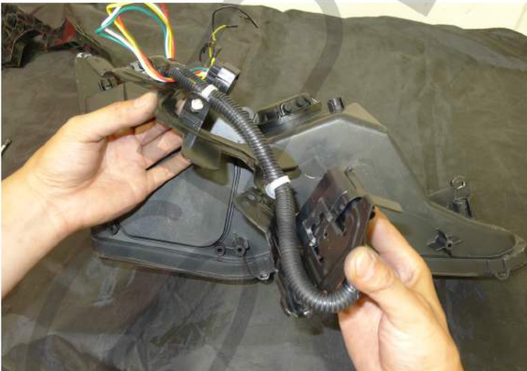
45. Attach the new projector headlight harness to metal bracket
