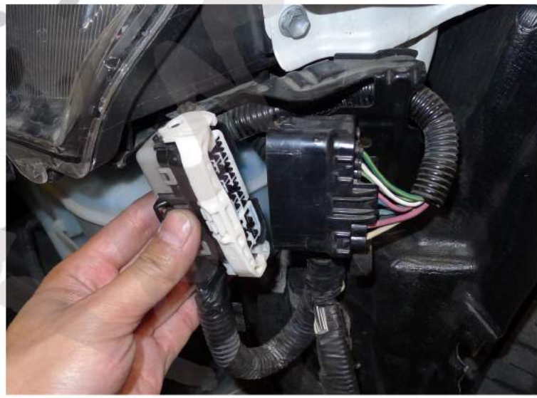
20. Disconnect the headlight harness
