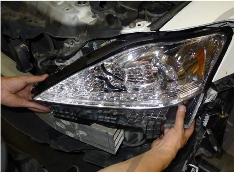
49. Place the new projector headlight in the stock location
