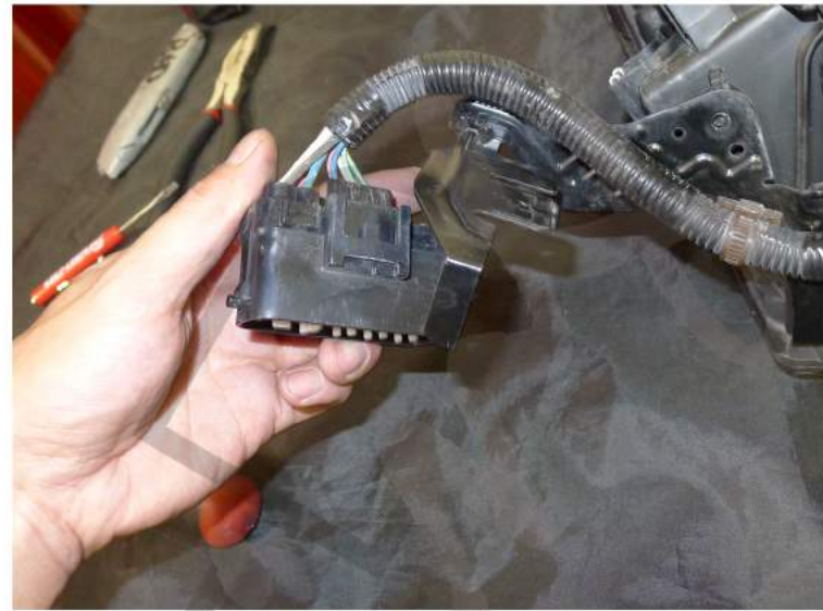
36. Remove the headlight harness connect from the metal bracket
