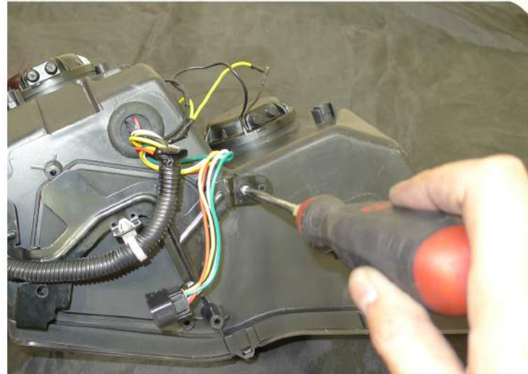
46. Secure the metal bracket to the new projector headlight
