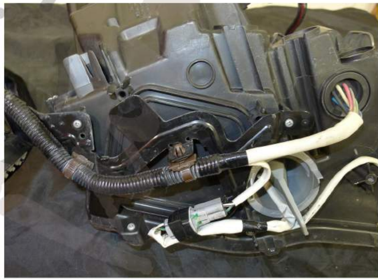
32. 2 Phillips head screws location
