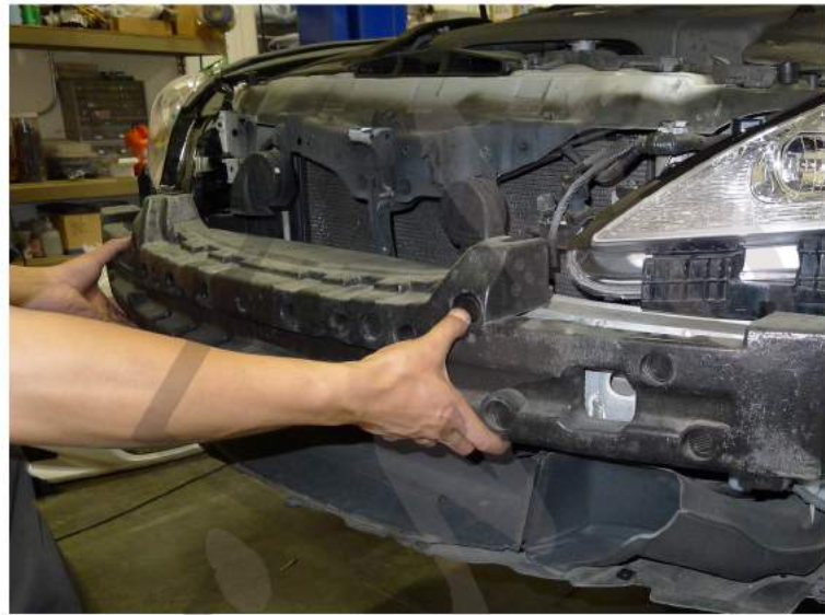
54. Replace the impact absorber
