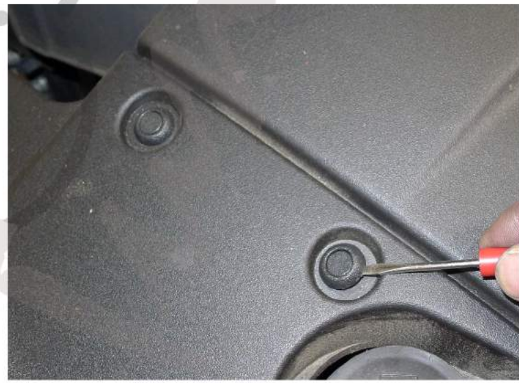
8. Remove the (11) plastic clips
