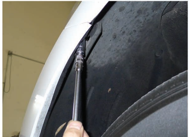
4. Remove the 10mm bolt
