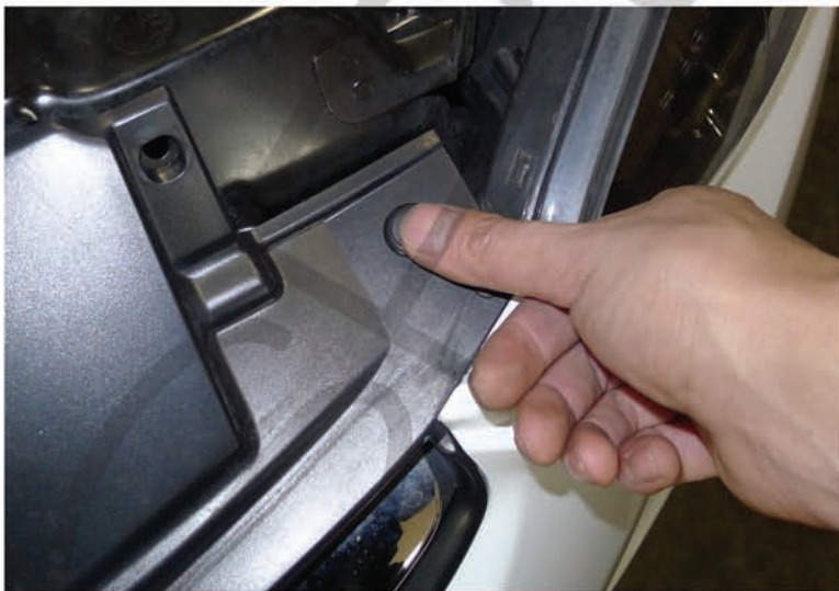
15. Replace the (5) plastic clips
