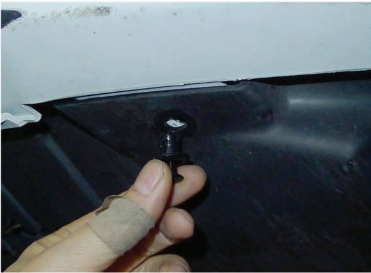
17. Replace the (6) plastic clips
