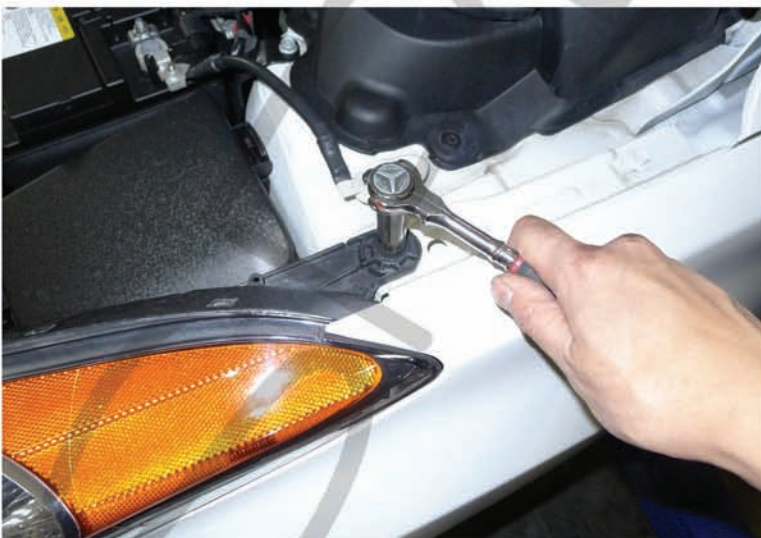
9. Remove the 12mm bolt
