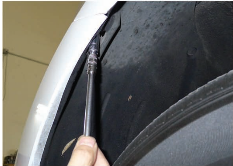
16 Tighten the 10mm bolt
