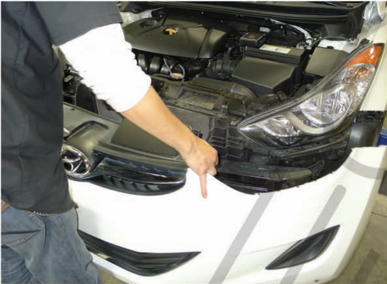
7. Remove the front bumper
