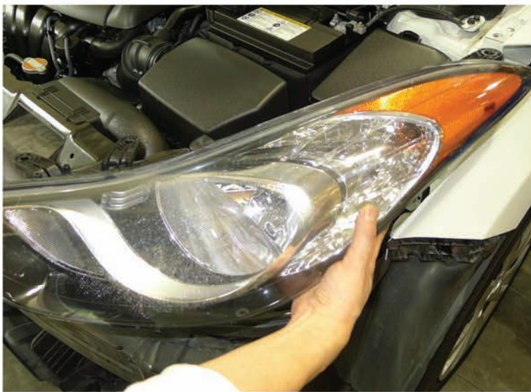
11. Remove the headlight
