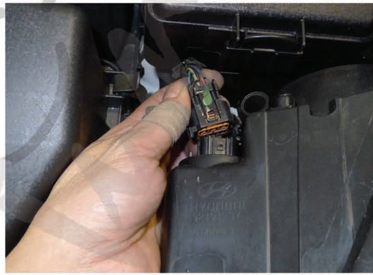
8. Disconnect the headlight harness
