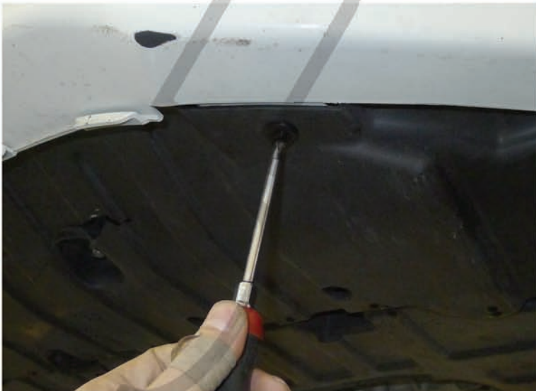
3. Remove the (6) plastic clips
