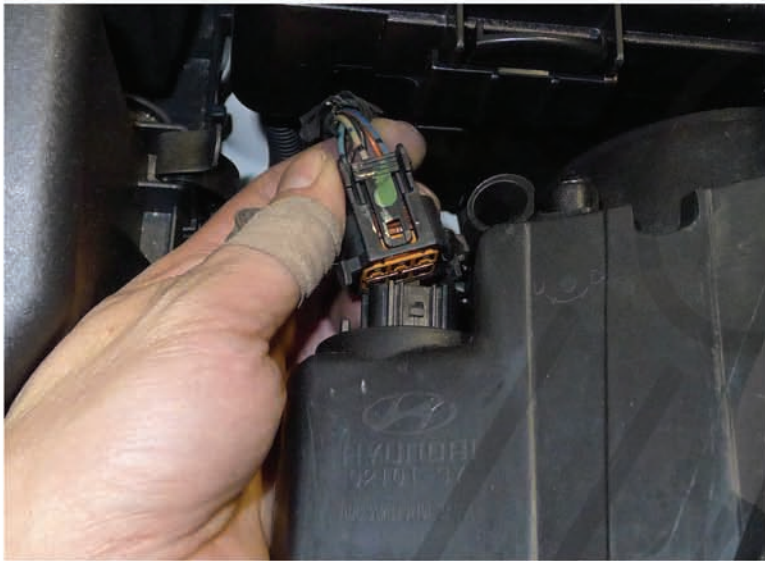
13. Connect the headlight harness
