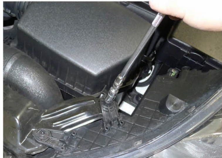
10. Remove the (2) 10mm bolts
