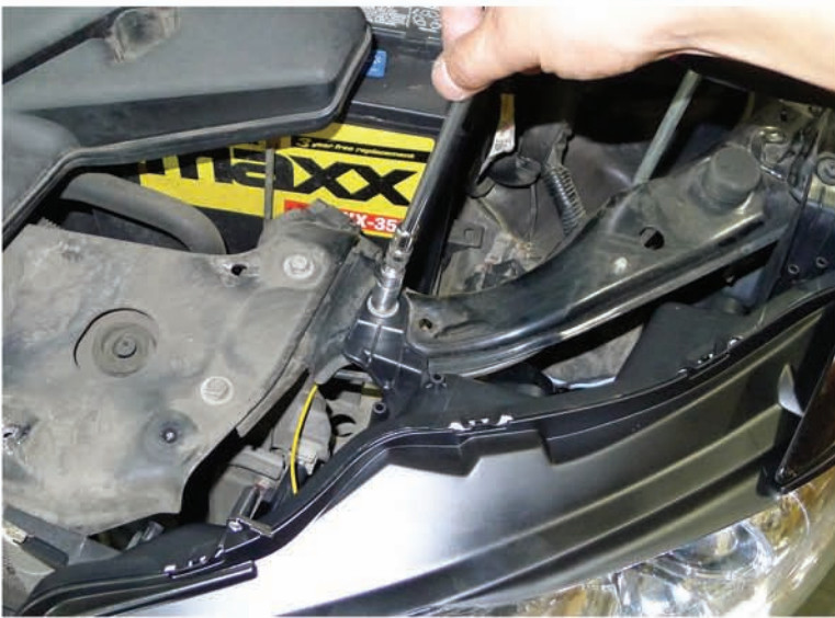
35. Tighten the (3) 10mm bolts
