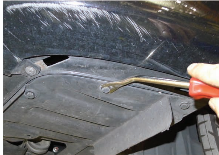
47. Replace the (6) plastic clips
