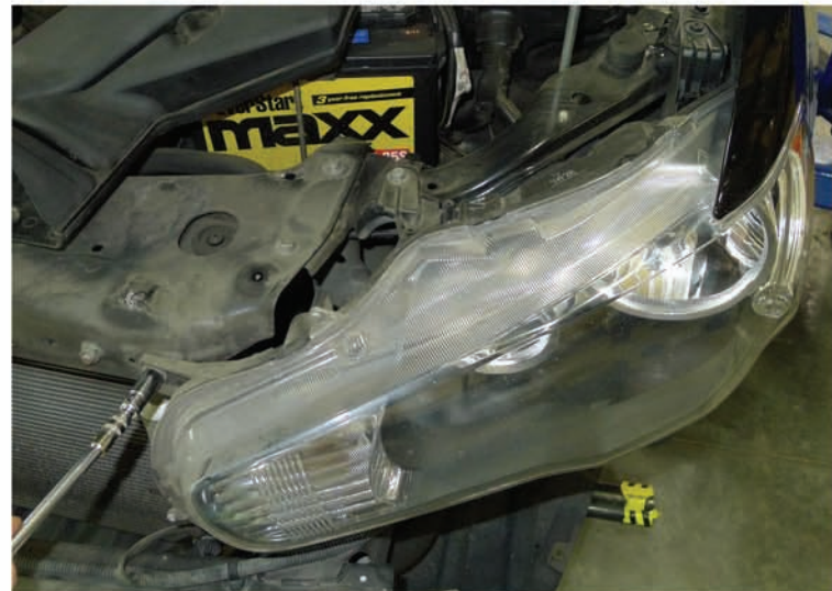
28. Remove the (3) 10mm bolts
