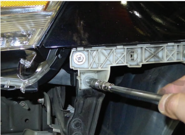
37. Tighten the 10mm bolt
