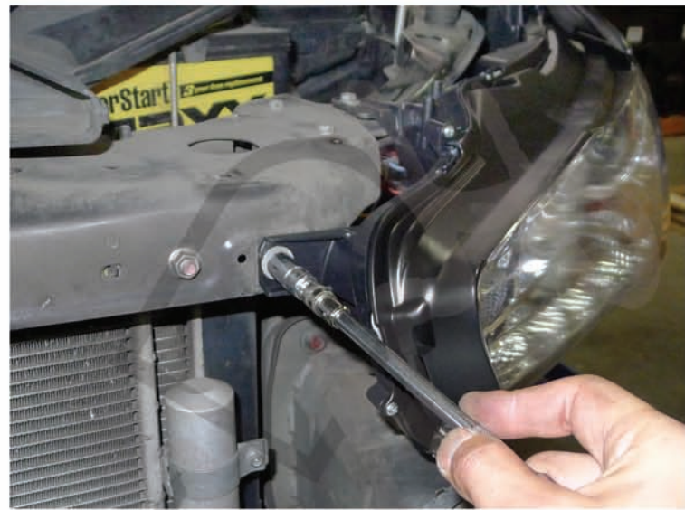
36. Tighten the (3) 10mm bolts
