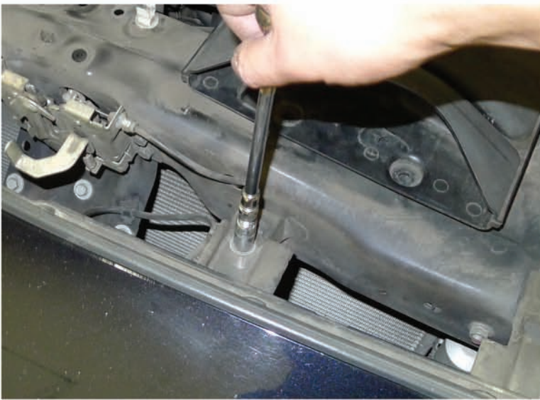
41. Tighten the (5) 10mm bolts
