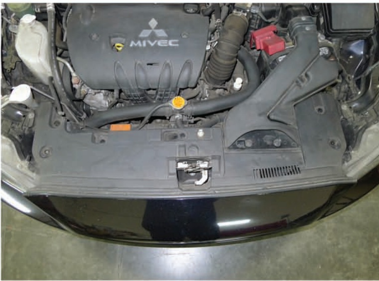
5. Remove the (4) plastic clips
