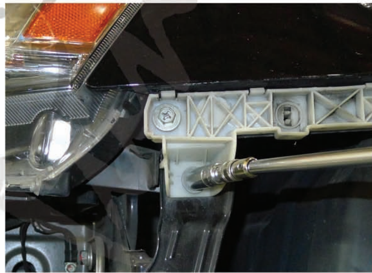
26. Remove the 10mm bolt
