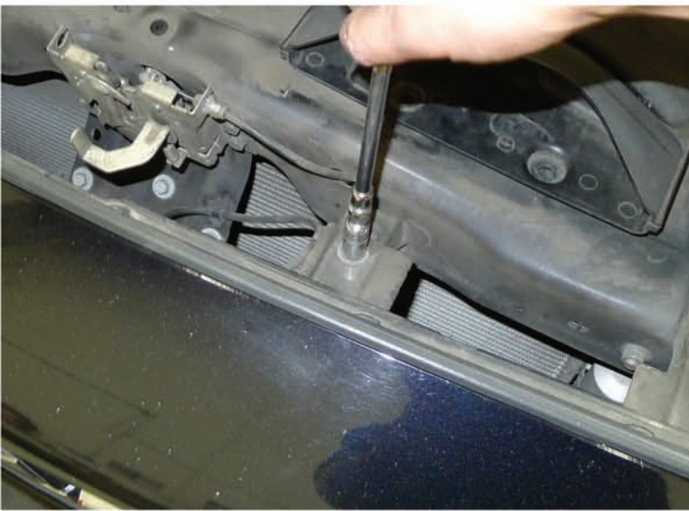
17. Remove the (5) 10mm bolts
