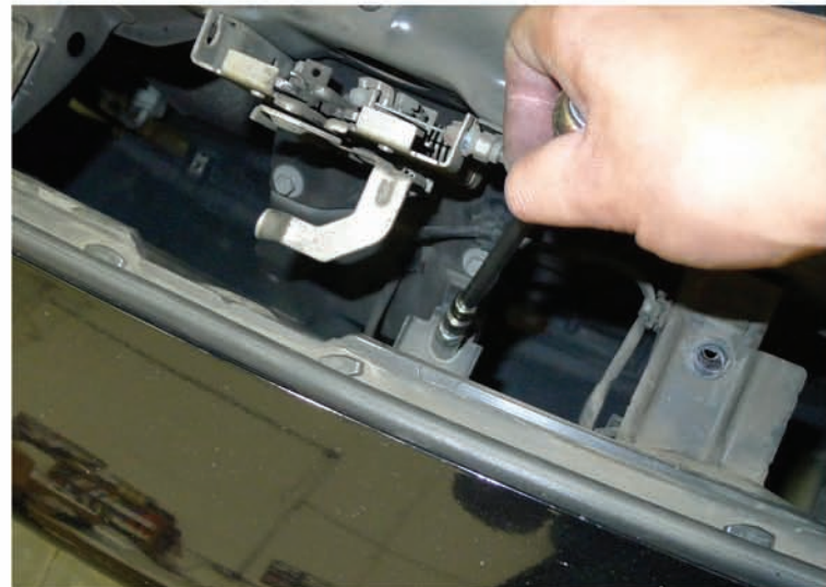
40. Tighten the (5) 10mm bolt
