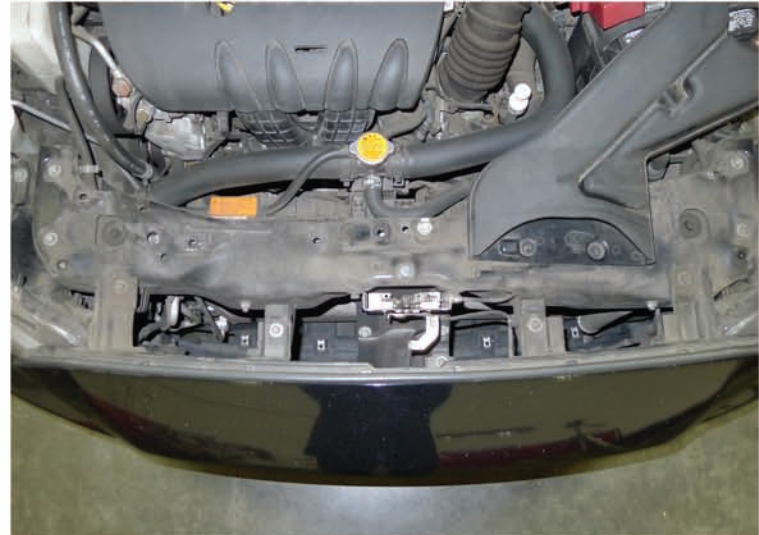
16. (5) 10mm bolts location
