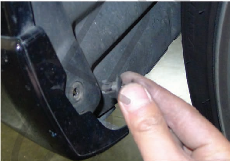
15. Remove the (2) plastic clips
