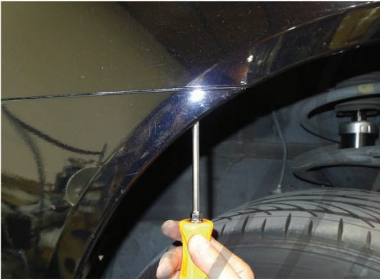
44. Tighten the phillips head screw
