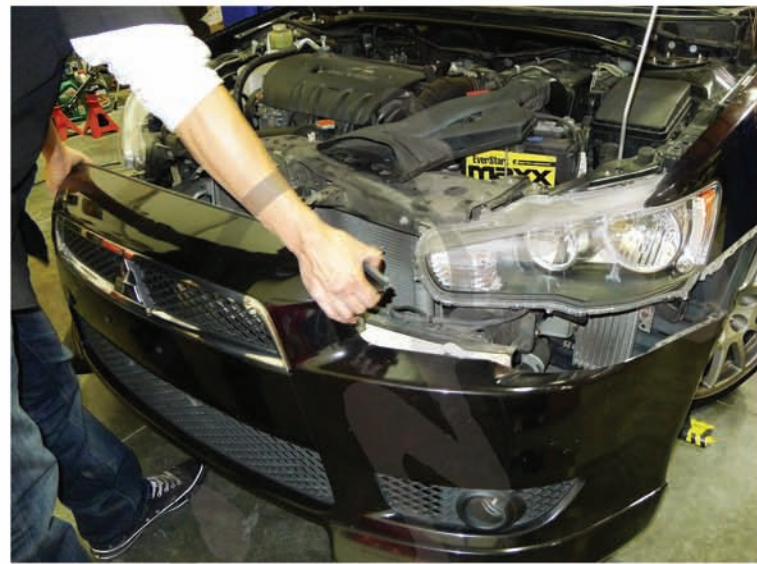
24. Remove the front bumper
