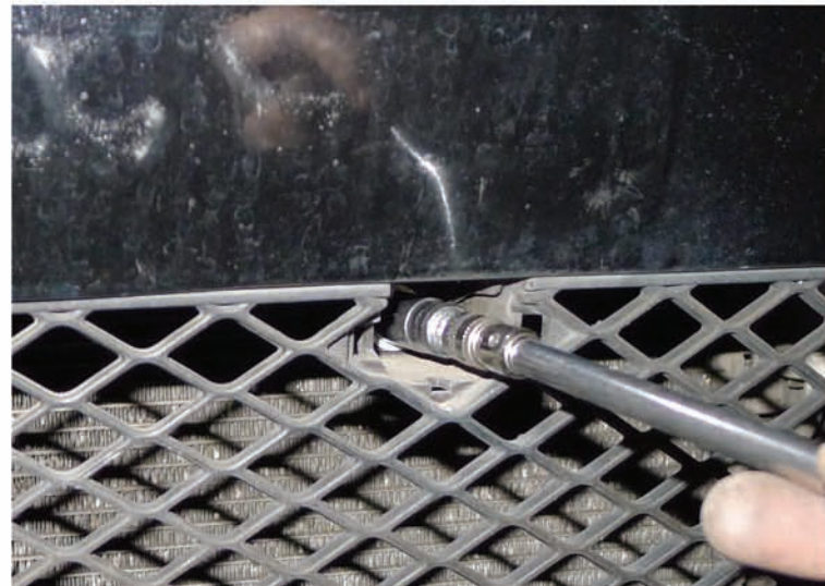
22. Remove the (2) 10mm bolts
