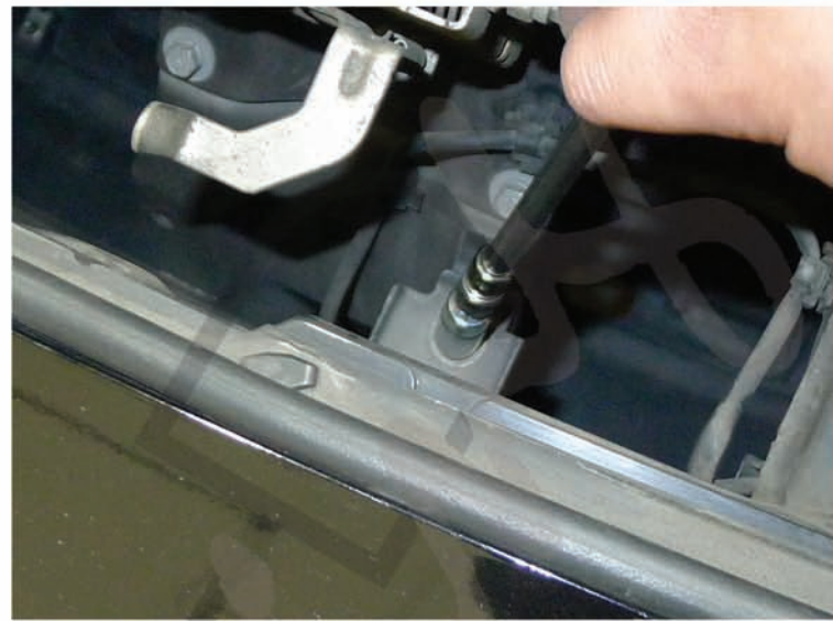
18. Remove the 10mm bolt
