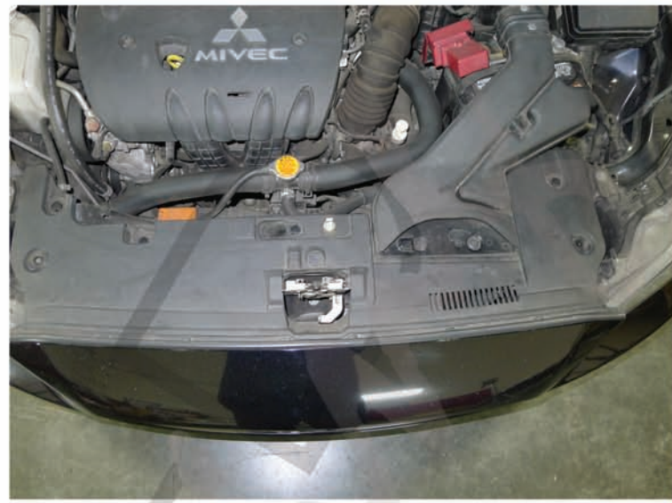
49. Replace the (4) plastic clips
