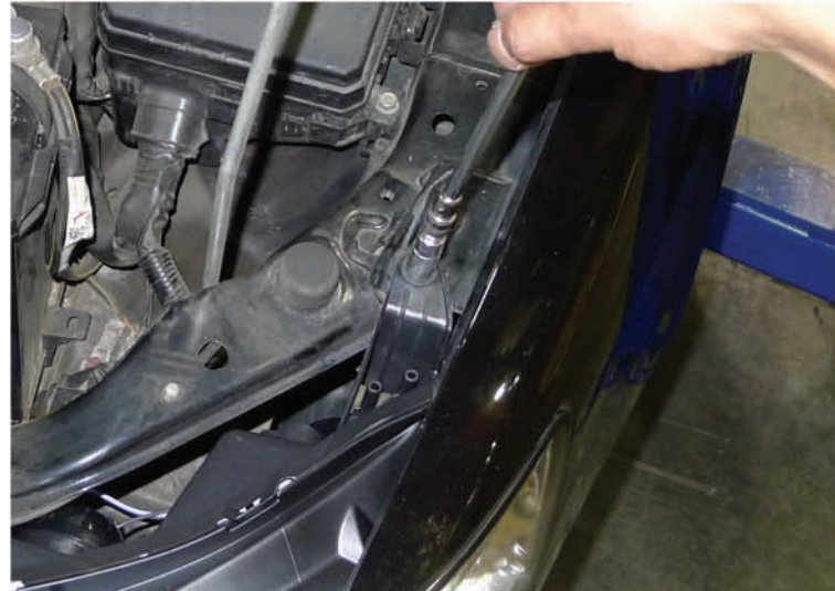
34. Tighten the (3) 10mm bolts
