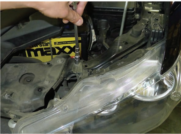
29. Remove the (3) 10mm bolts
