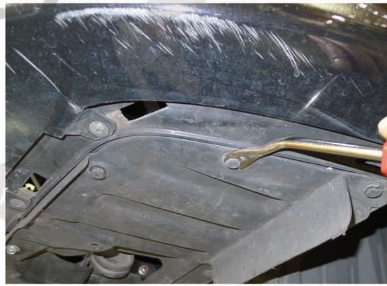
8. Remove the (6) plastic clips
