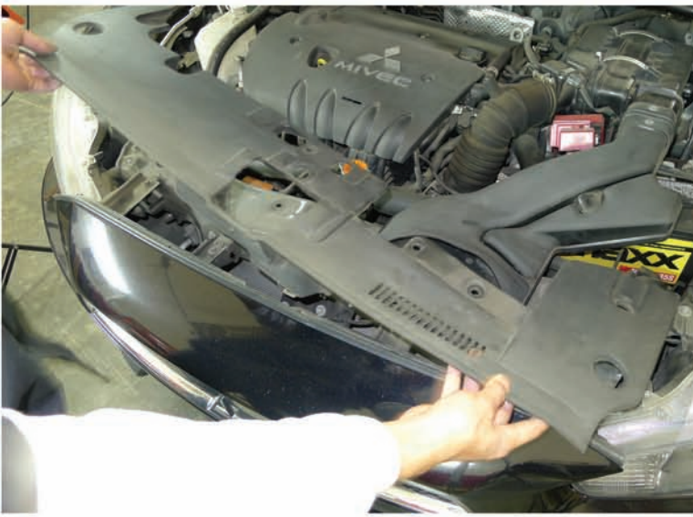
48. Replace the plastic moulding
