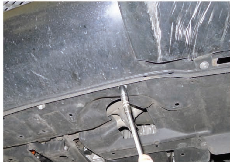
10. Remove the (5) 10mm bolts
