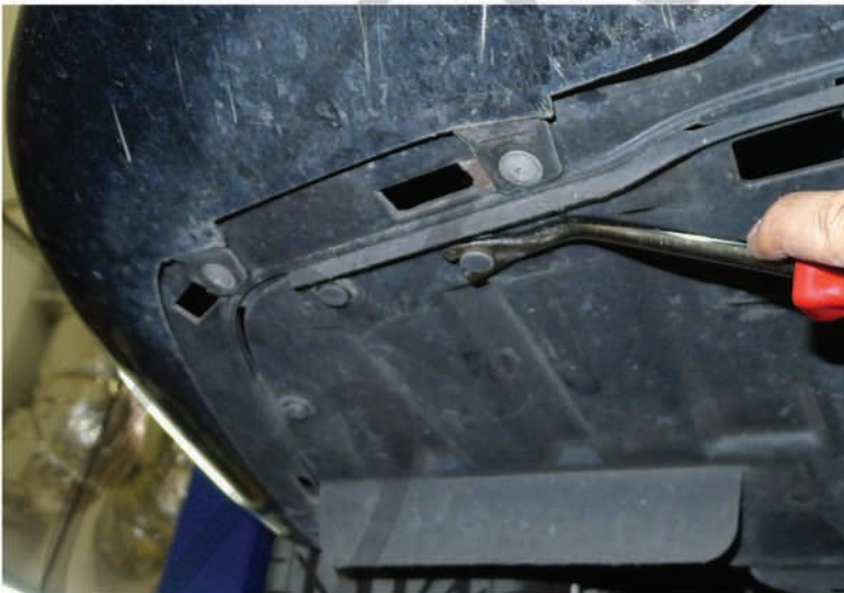
9. Remove the (6) plastic clips
