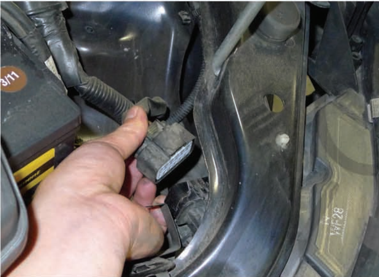
31. Disconnect the headlight and remove the headlight harness
