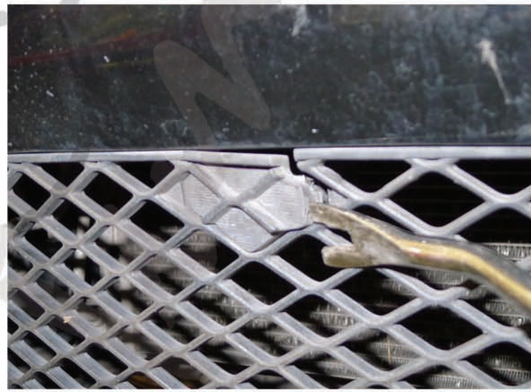
20. Remove the (2) plastic cover
