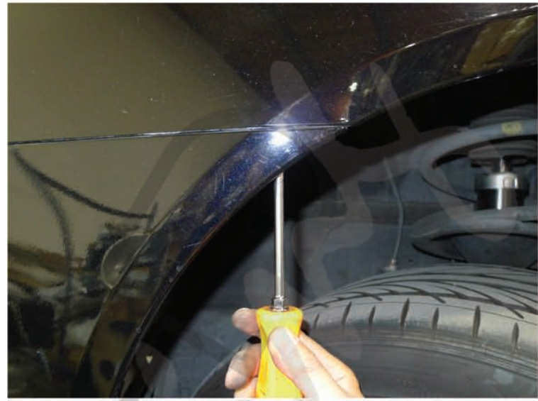
12. Remove the phillips head screw
