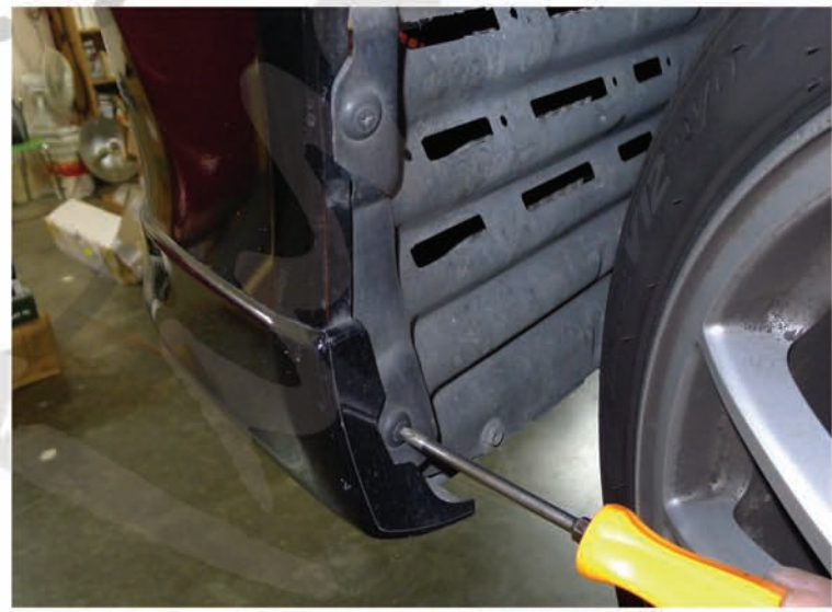
14. Remove the (2) plastic clips
