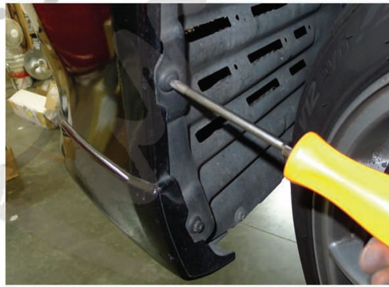
45. Replace the (2) plastic clips
