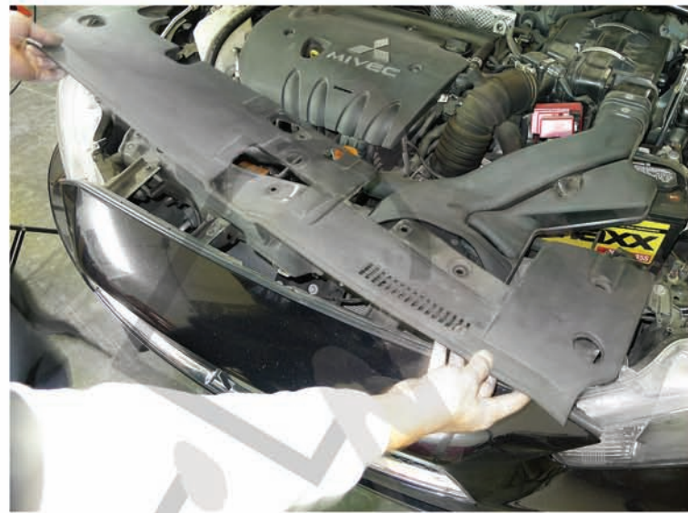
6. Remove the plastic moulding
