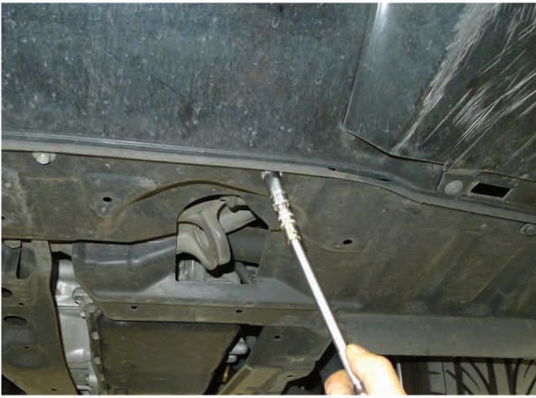
11. Remove the (5) 10mm bolts
