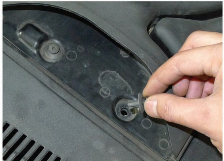
4. Remove the (2) plastic clips
