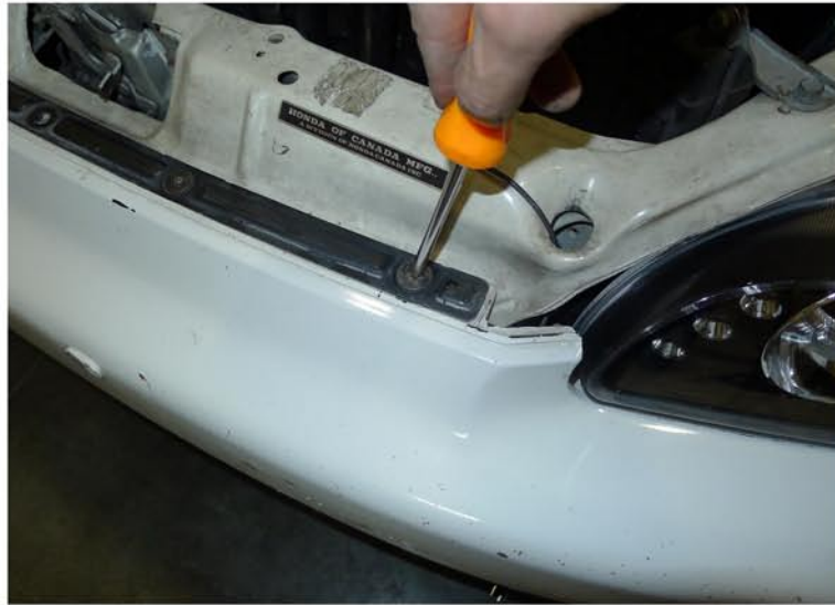
26. Replace the metal bracket and tighten the (5) phillips head screws
