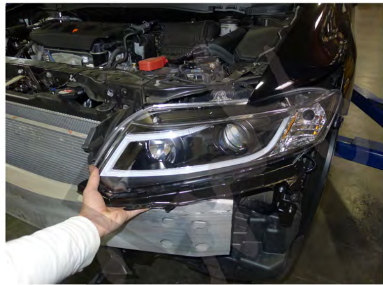
24. Place the new headlight in the stock location
