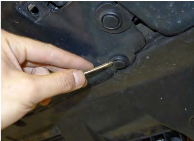
4. Remove the (12) plastic clips
