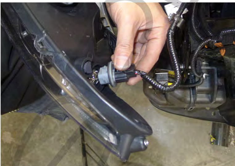
21. Connect the headlight harness to the new headlight Please see the " L. E. D. headlights installation instructions" If your headlights don't have L.E.D. You can skip the installation instruction.
