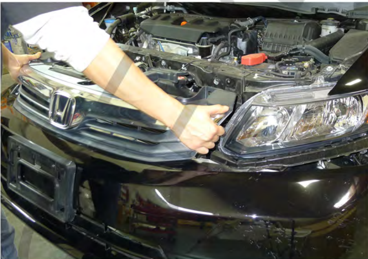
9. Remove the front bumper
