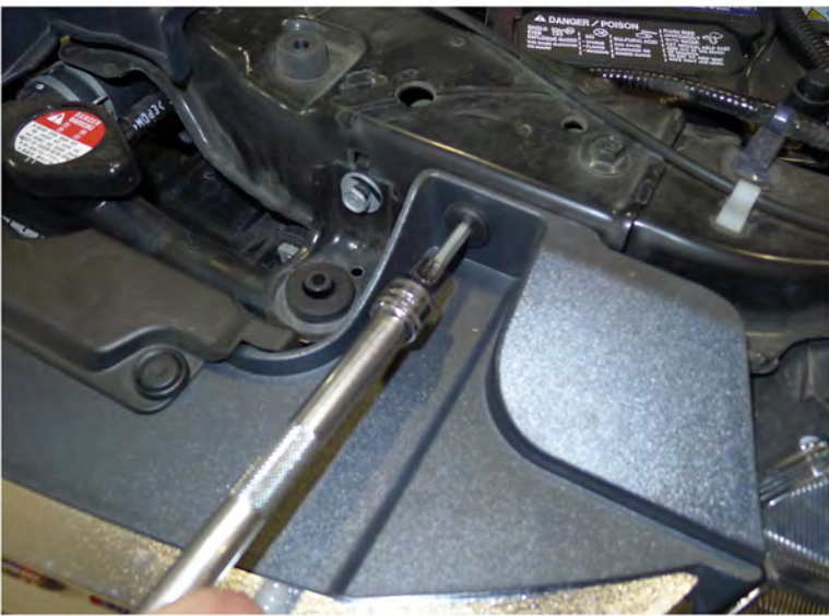
29. Replace the (2) 5mm allen bolts
