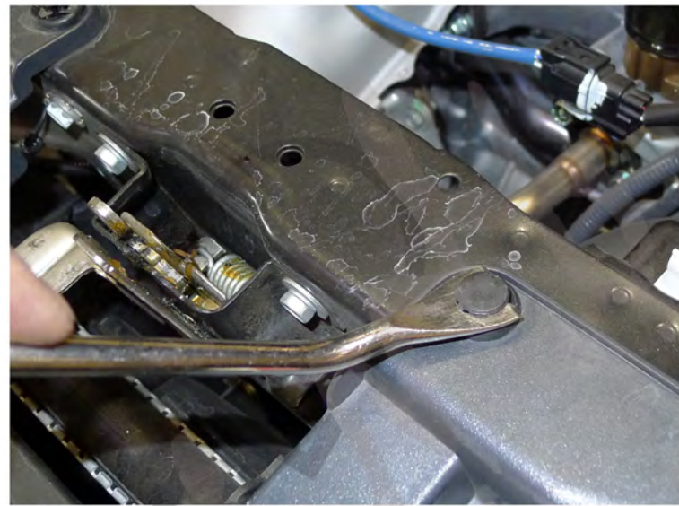
30. Replace the (2) plastic clips
