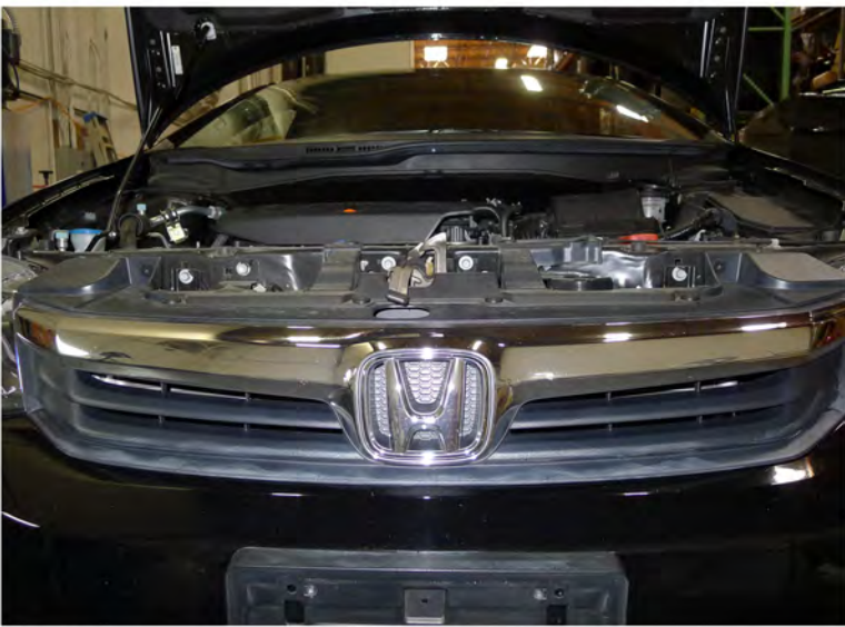
5. (2) 5mm allen bolt location
