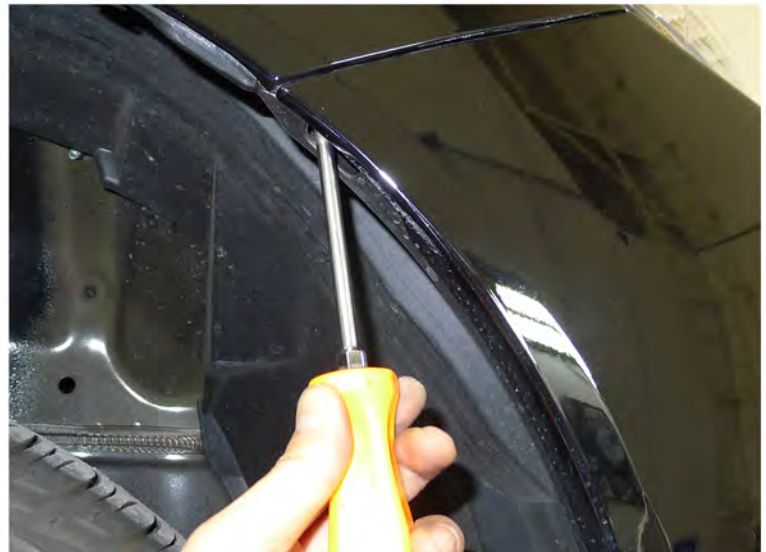
5. Remove the phillips head screw
