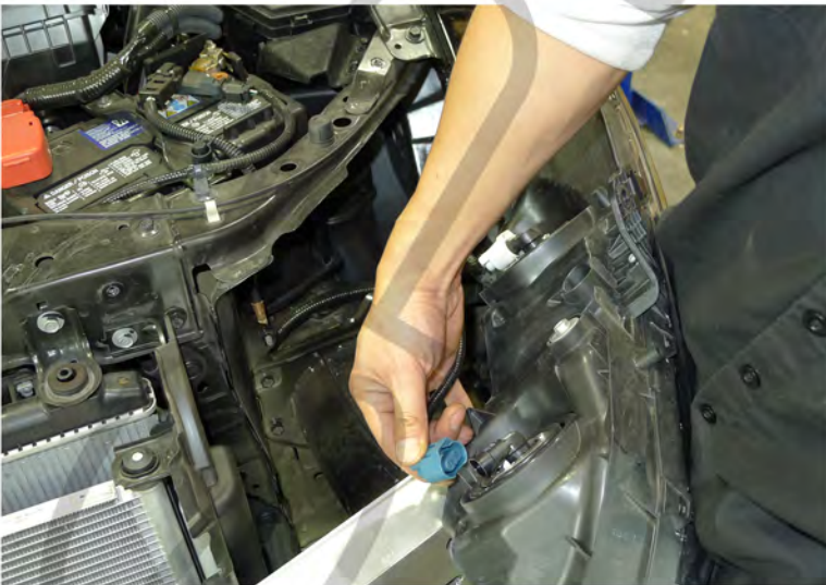
15. Disconnect the headlight harness
