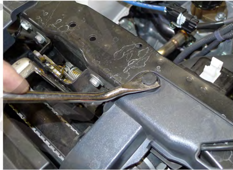
8. Remove the (2) plastic clips
