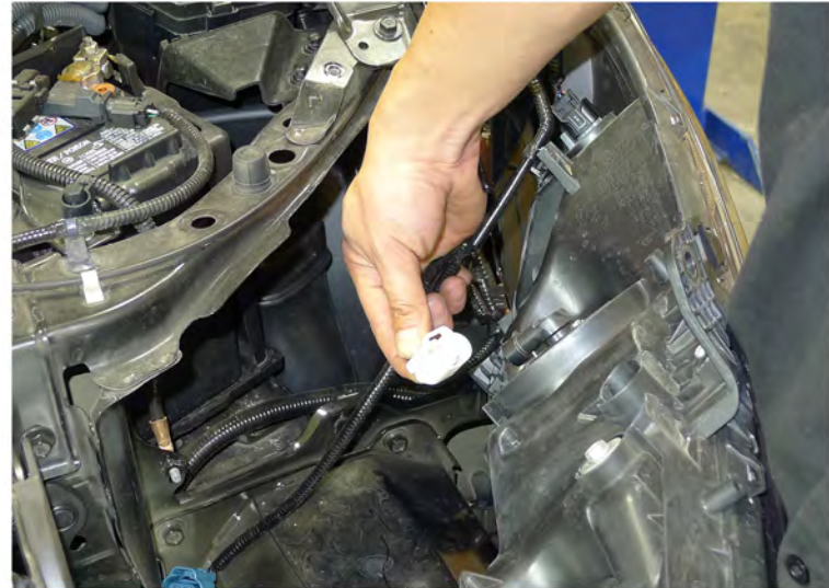
16. Disconnect the headlight harness
