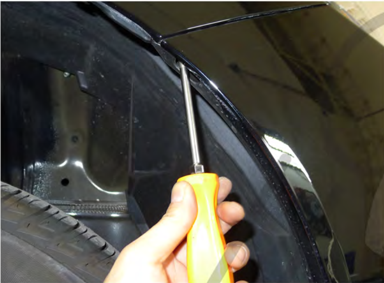
31. Replace the (2) phillips head screws
