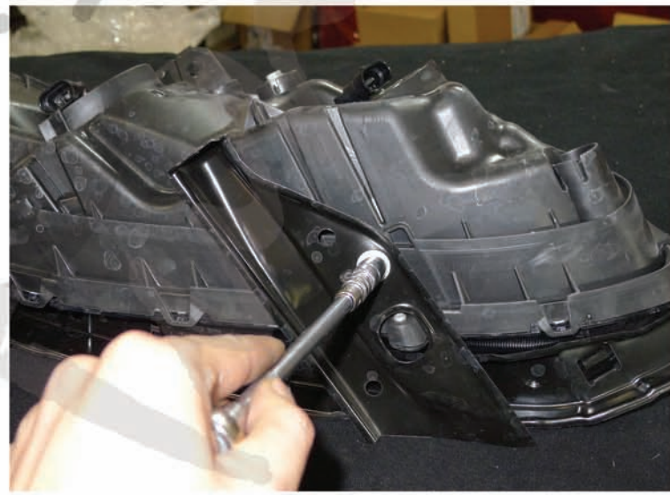
20.. Install the headlight bracket on the new headlight
