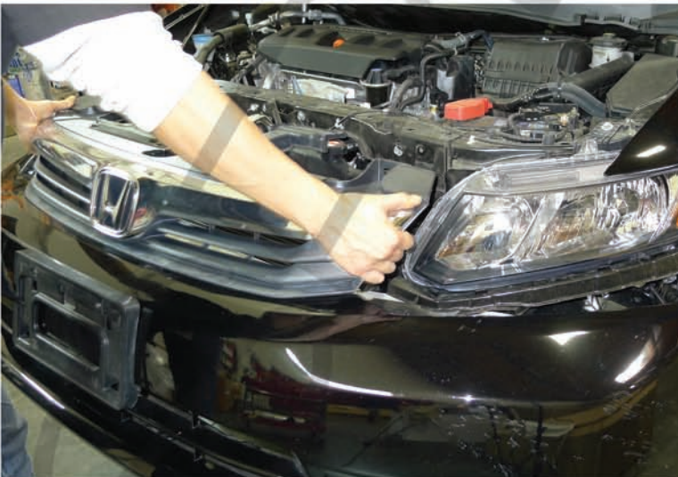
9. Remove the front bumper
