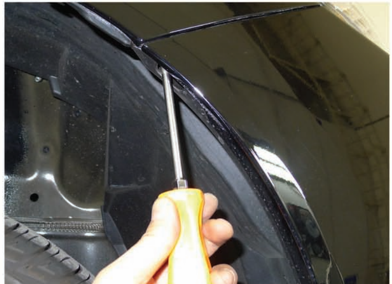
5. Remove the phillips head screw
