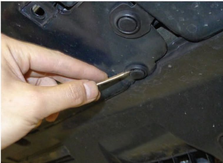
4. Remove the (12) plastic clips
