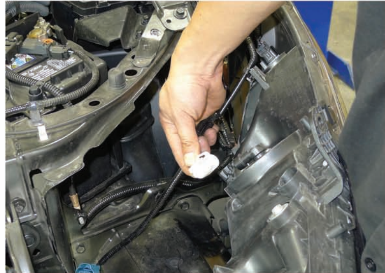
16. Disconnect the headlight harness
