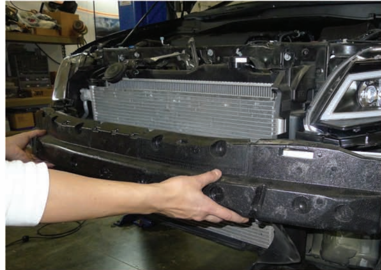
28. Replace impact absorber and place the front bumper
