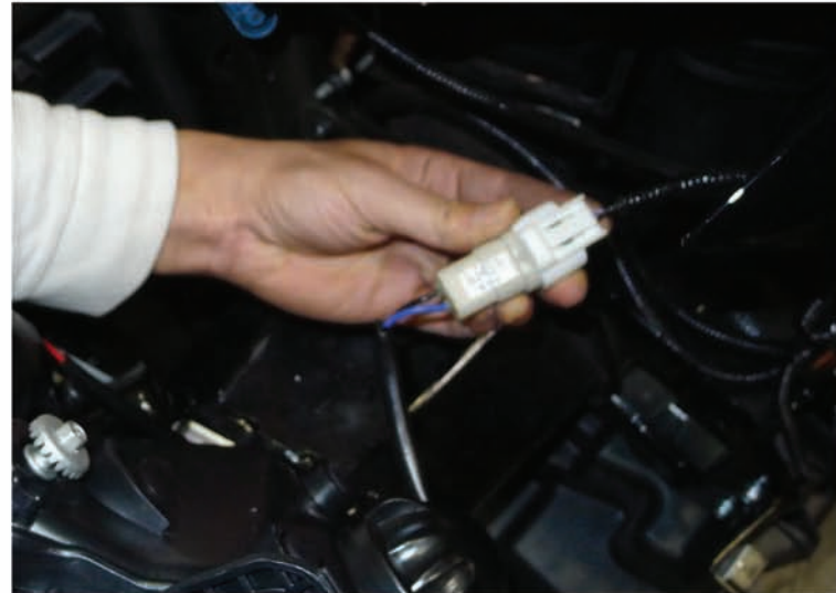
22. Connect the headlight harness to the new headlight
