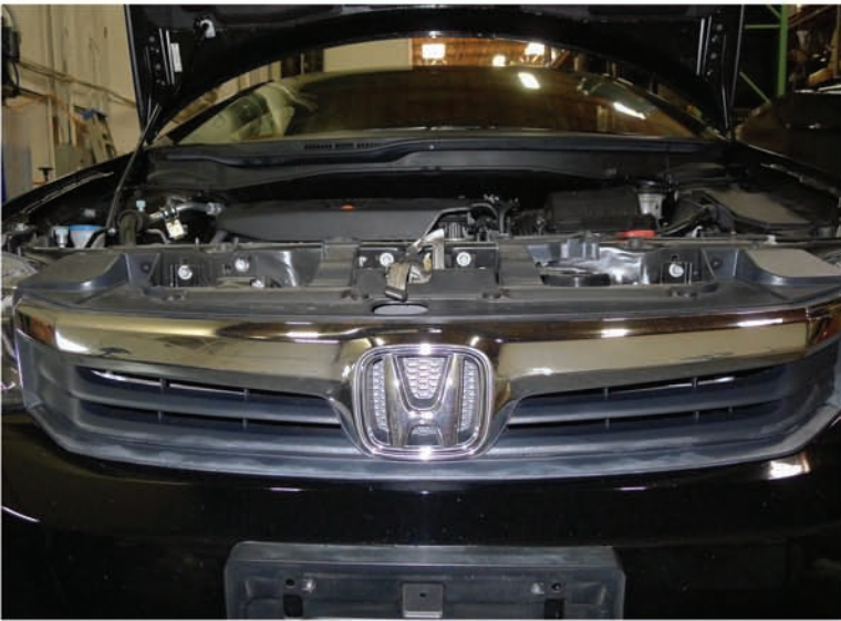
5. (2) 5mm allen bolt location
