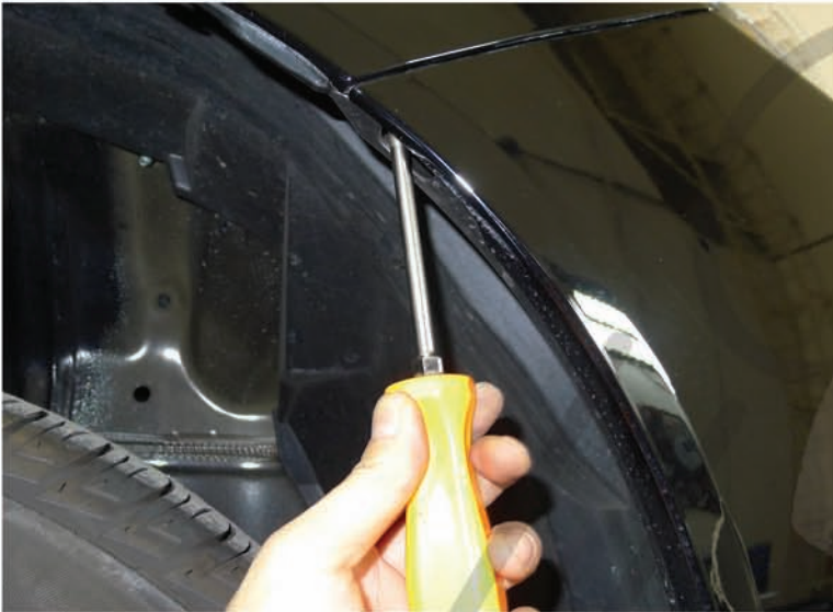
31. Replace the (2) phillips head screws
