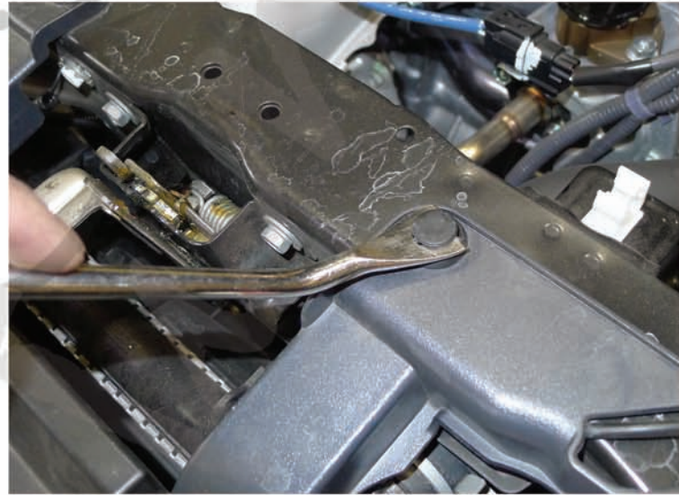
8. Remove the (2) plastic clips
