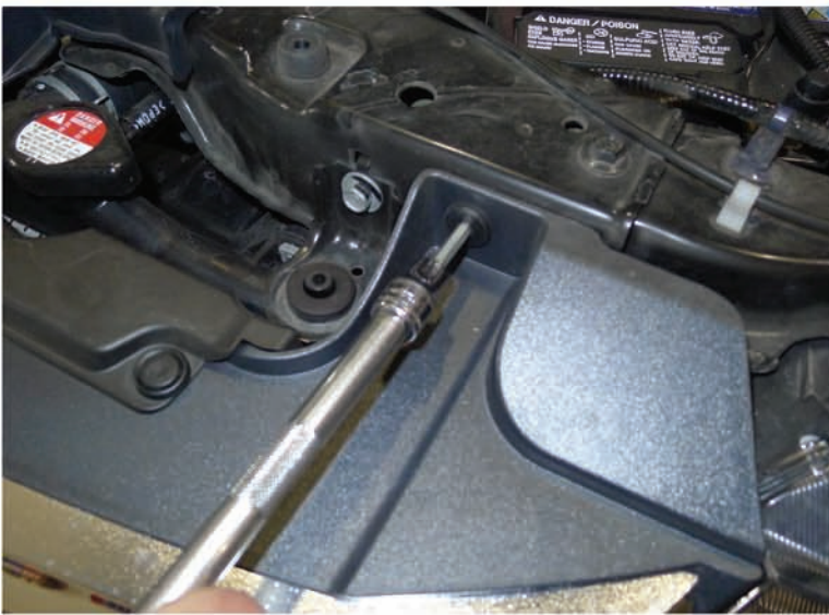
29. Replace the (2) 5mm allen bolts
