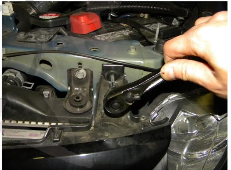
8. Remove the 5mm allen head bolt
