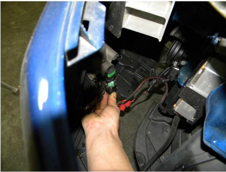
29. Connect the fog light harness
