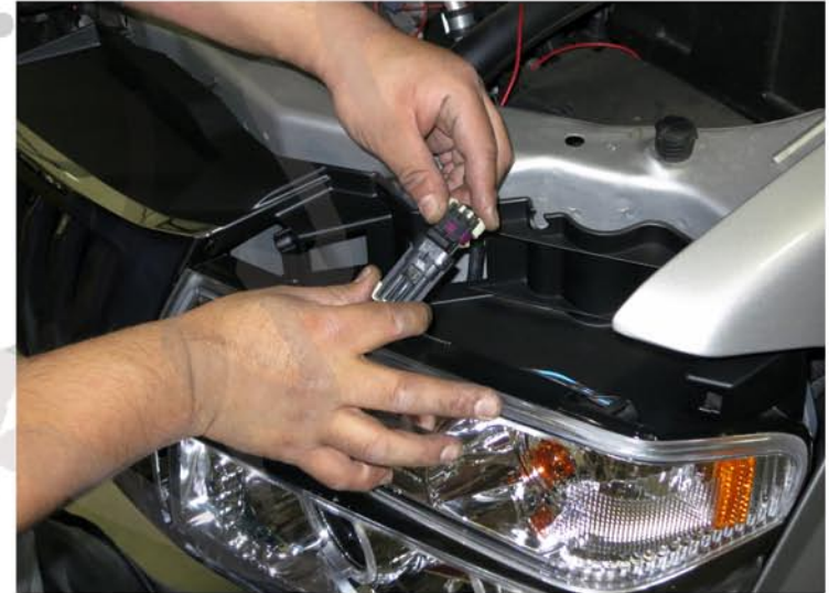
14. Connect the bumper light harness to the bumper light
