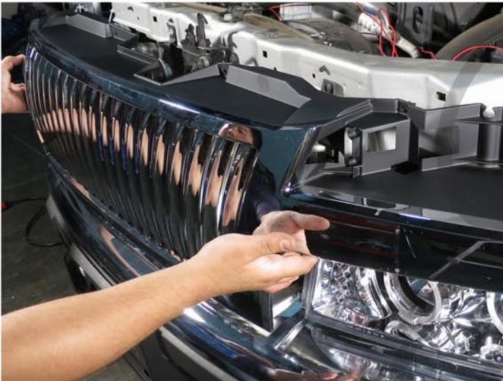
13. Replace the front grill
