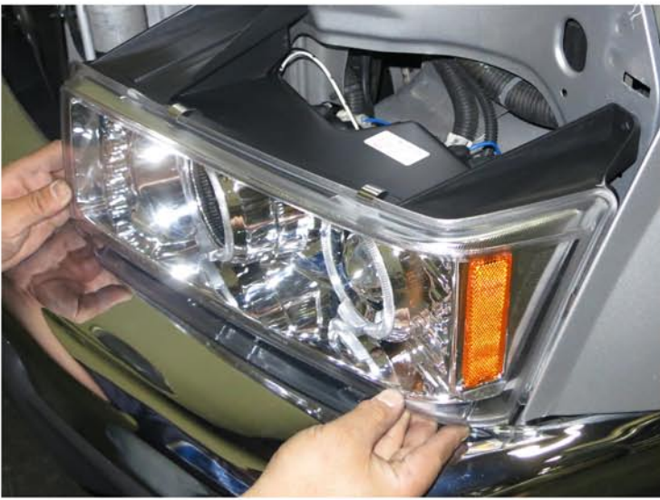
11. Place the projector headlight in the stock location
