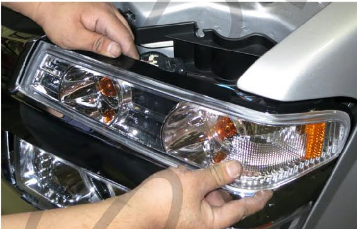
15. Replace the bumper light. Please repeat the steps in order from 1 to 15 for the opposite side
