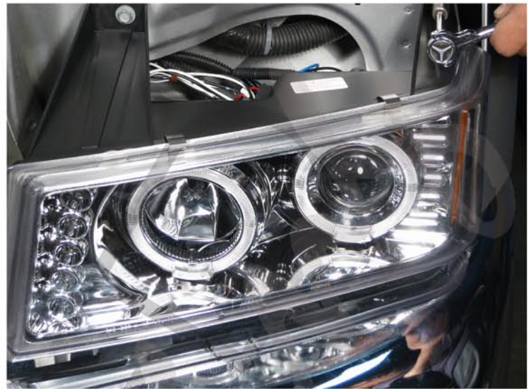
12. Tighten the (2) 10mm bolts
