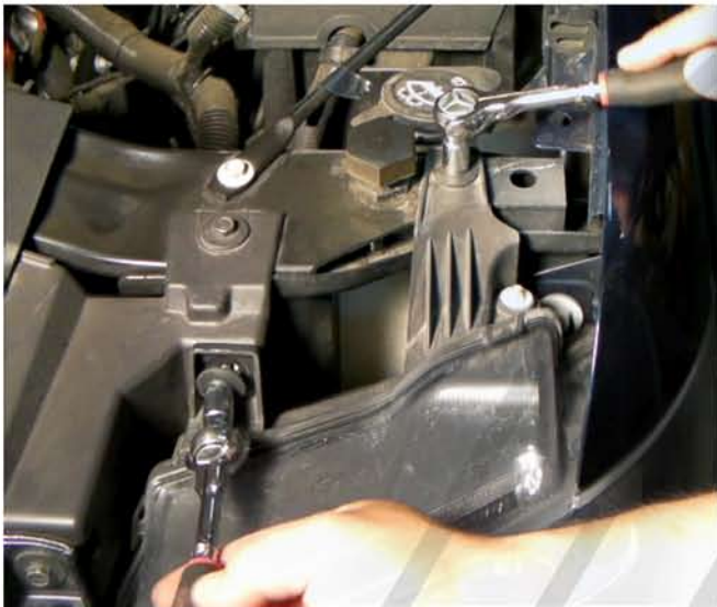
7. Remove two headlight screws
