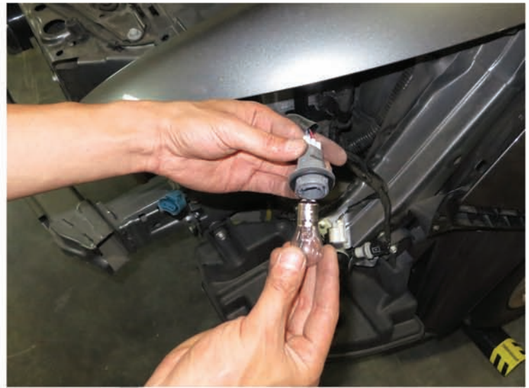
18. Remove the turn signal light bulb
