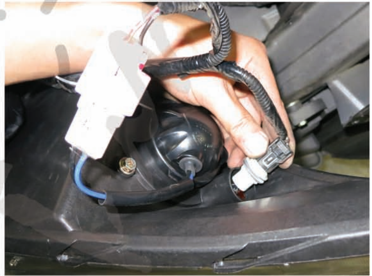
20. Place the turn signal socket into the projector headlight
