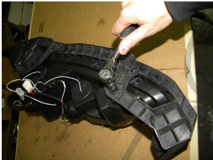
25. Place the bracket on the new headlight and tighten the (2) 10mm bolts
