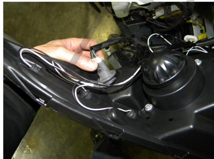
27. Connect the headlight harness to the new headlight Please see the Halo and L.E.D installation instructions If your headlights don't have HALO or L.E.D. You can skip it
