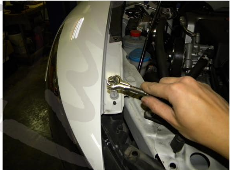
20. Remove the 10mm bolt
