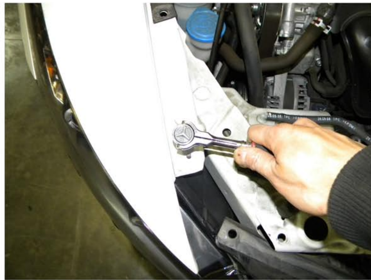
34. Tighten the 10mm bolt
