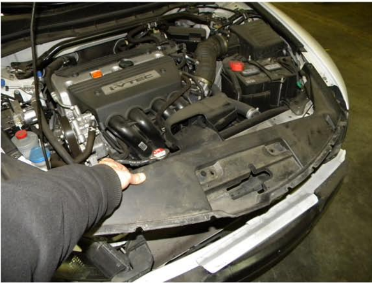
11. Remove the plastic moulding
