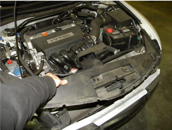
37. Remove the plastic moulding
