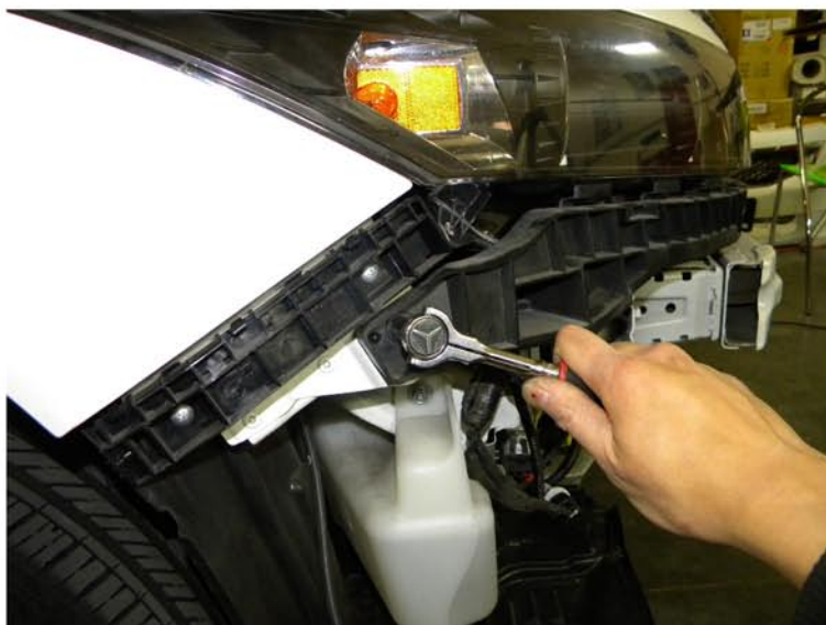
33.. Tighten the 10mm bolt
