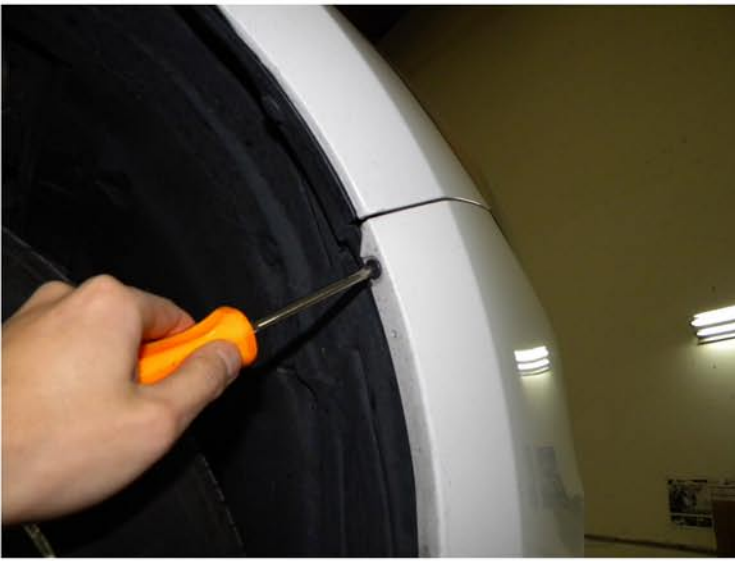
41. Tighten the phillips head screw
