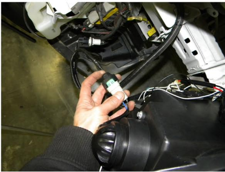
29. Connect the headlight harness to the new headlight
