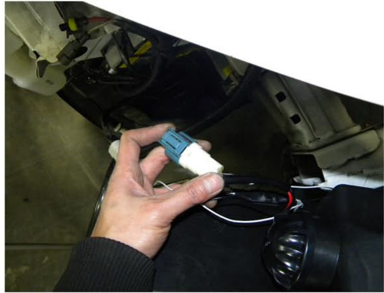
30. Connect the headlight harness to the new headlight
