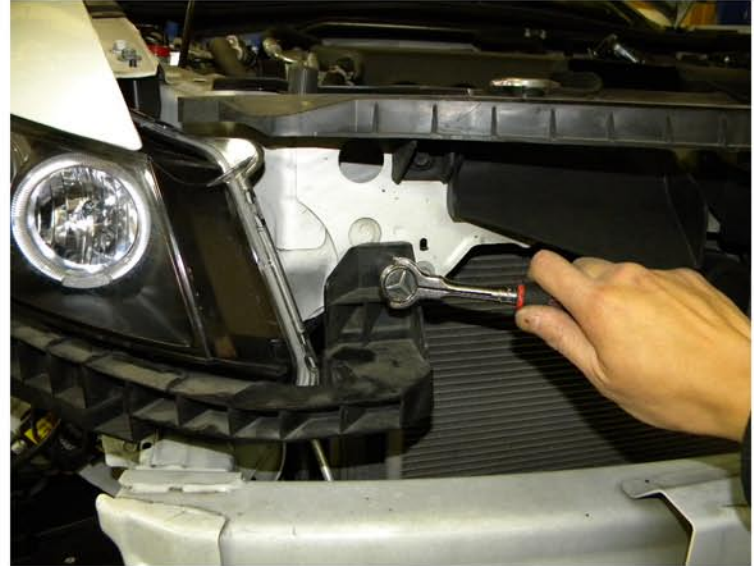
32. Tighten the 10mm bolt
