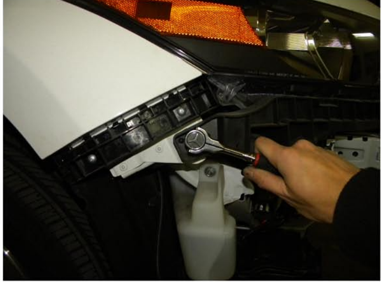
16. Remove the 10mm bolt
