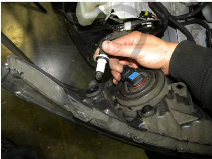
21. Remove the headlight and unplug the headlight harness
