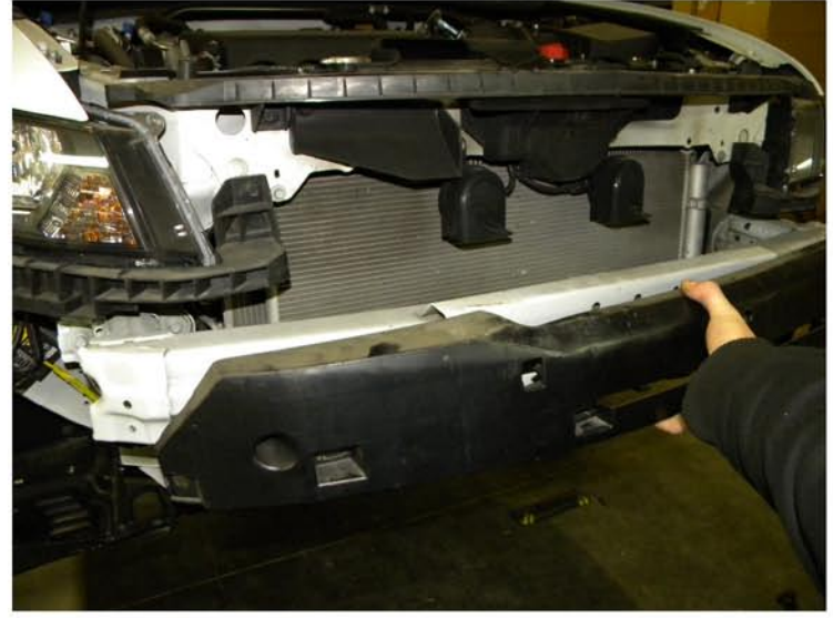
14. Remove the impact absorber
