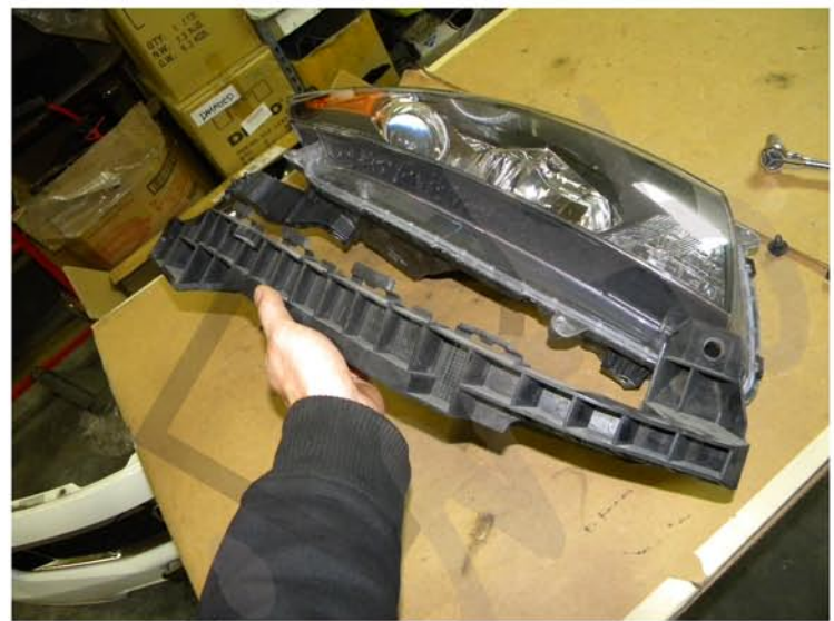
24. Remove the headlight bracket
