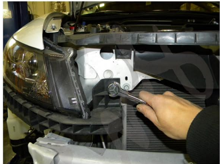
18. Remove the 10mm bolt
