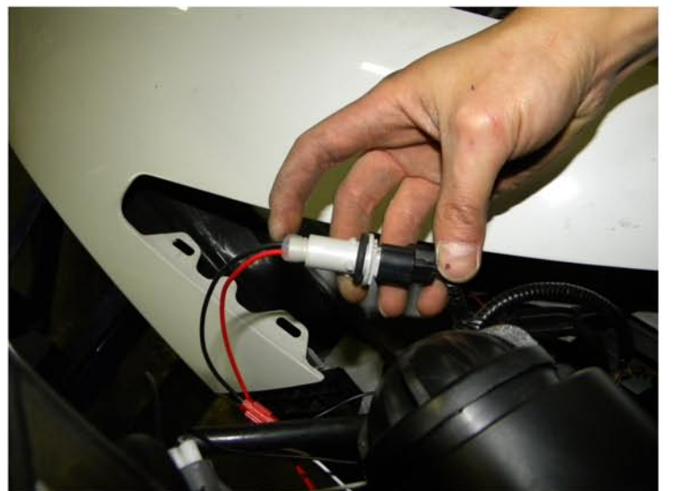
28. Connect the headlight harness to the new headlight
