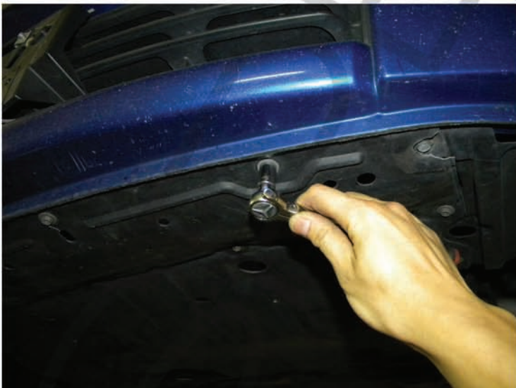
27. Tighten the (10) 10mm bolts Please repeat the steps in order from 1 to 27 for the opposite side
