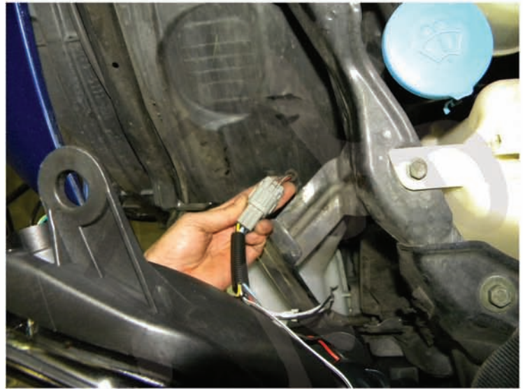
18. Plug in the new headlight to the headlight harness
