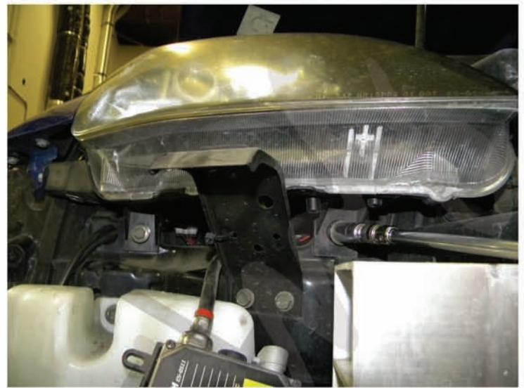
12. (2) 10mm bolts location
