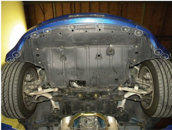
1. (10) 10mm bolts location
