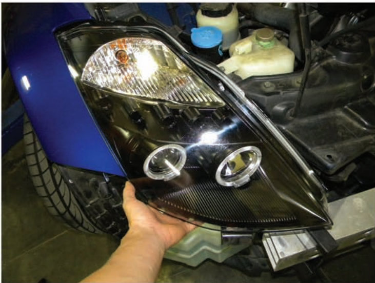
19. Place the new headlight into the stock location Please see the Halo and L.E.D installation instruction If your headlights don't have HALO or L.E.D. You can skip it
