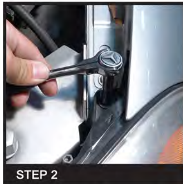
Remove (1) 7mm bolt then remove the headlight
