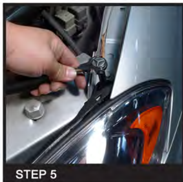
Tighten (1) 7mm bolt
