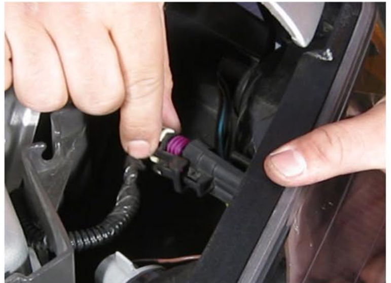
4. Disconnect the bumper light harness
