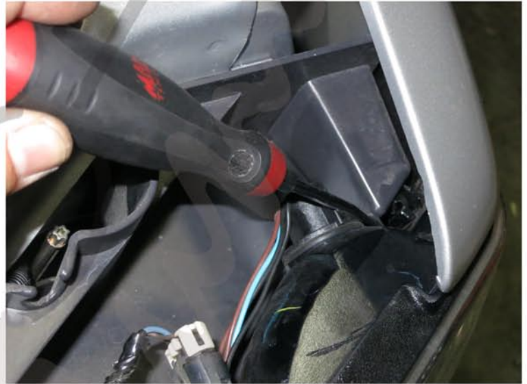
2. Release the retaining clip
