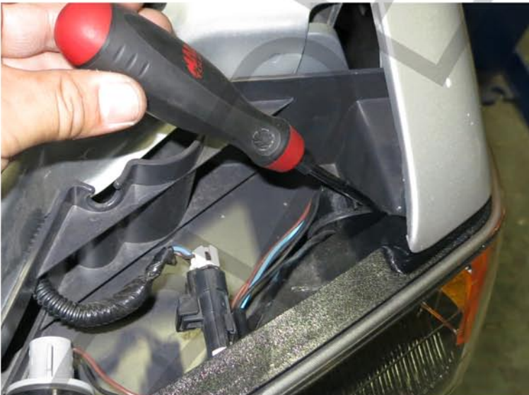
3.. Release the bumper light retaining clip
