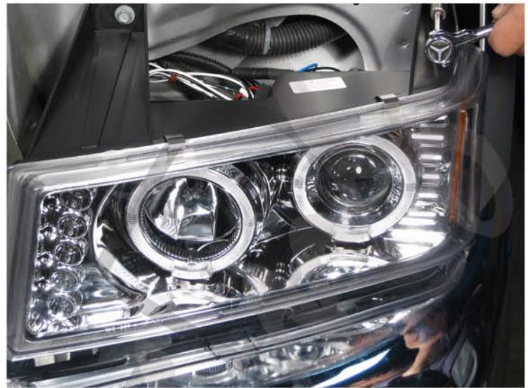
12. Tighten the (2) 10mm bolts
