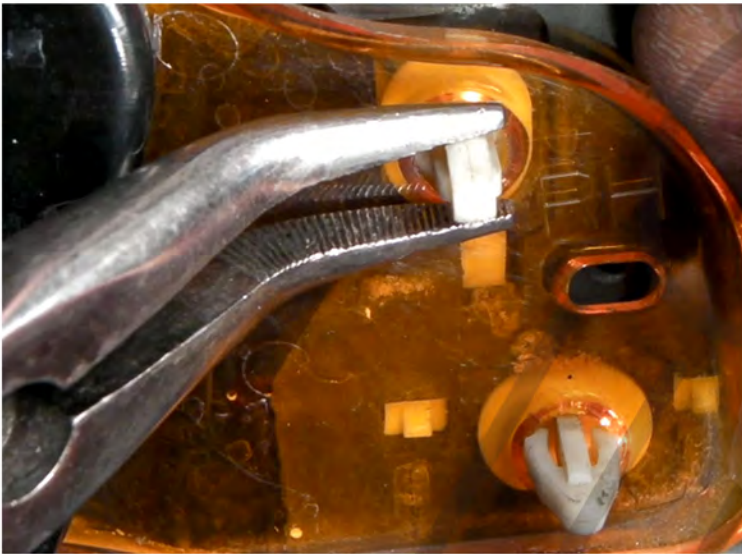
7. Squeeze two clips to remove the bumper light
