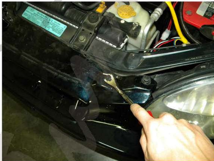
2. Remove the (4) plastic clips
