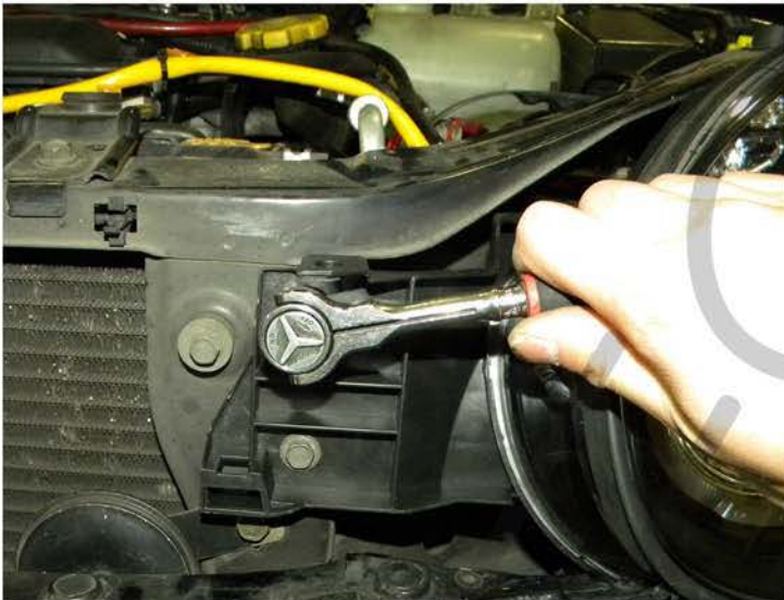
19. Tighten the (2) 10mm bolts
