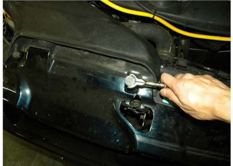
22. Tighten the (2) 10mm bolts
