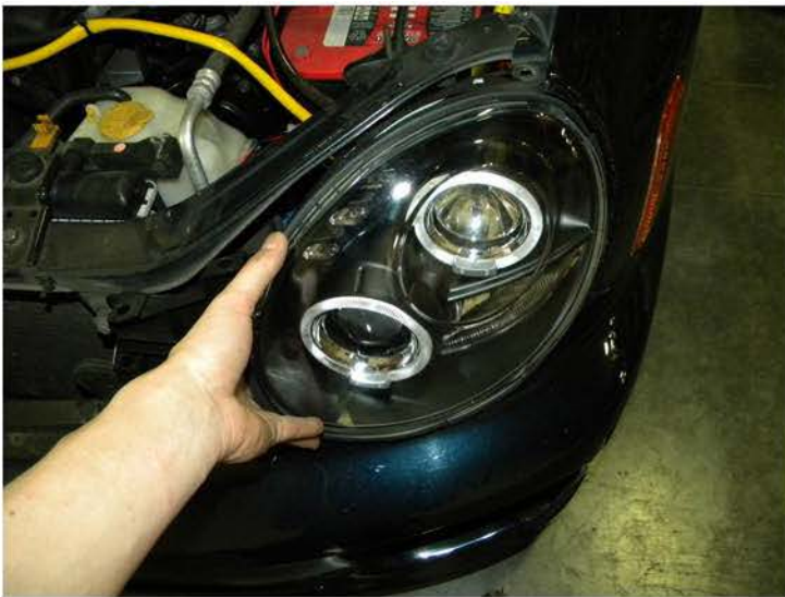
17. Place the new headlight in the stock location
