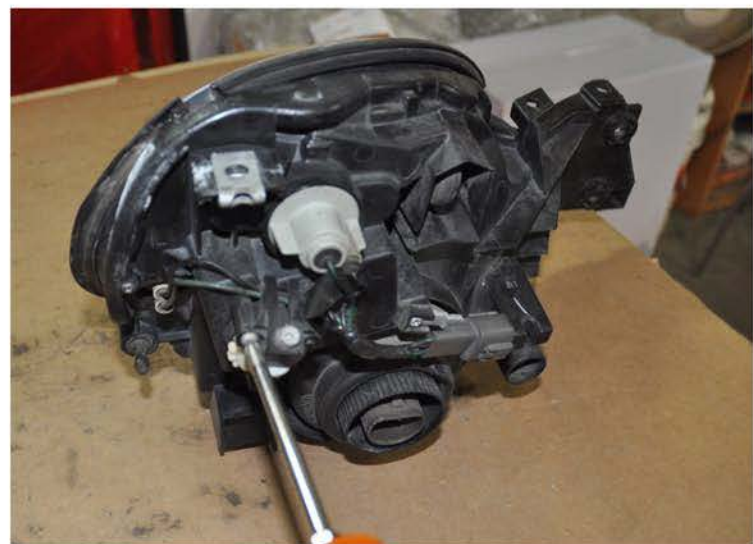
10. Disconnect the headlight harness
