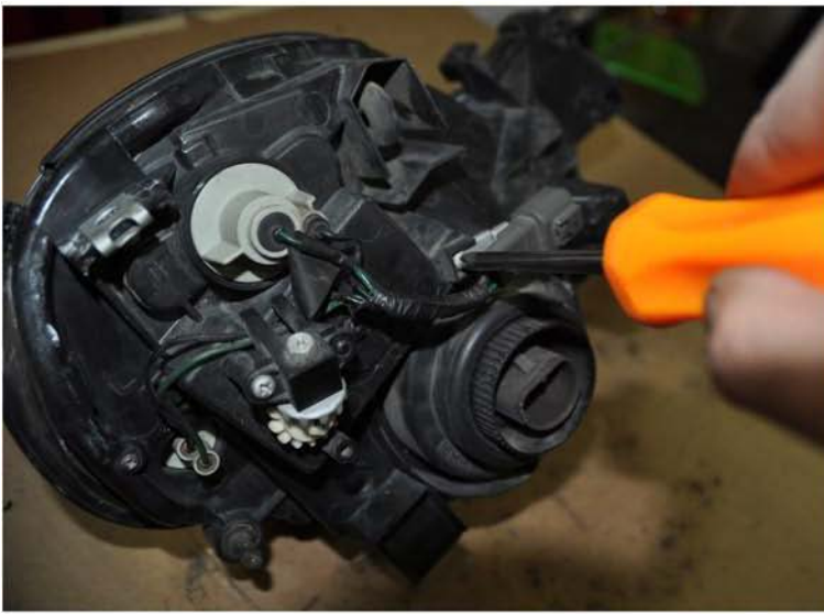
11. Remove the phillips head screw
