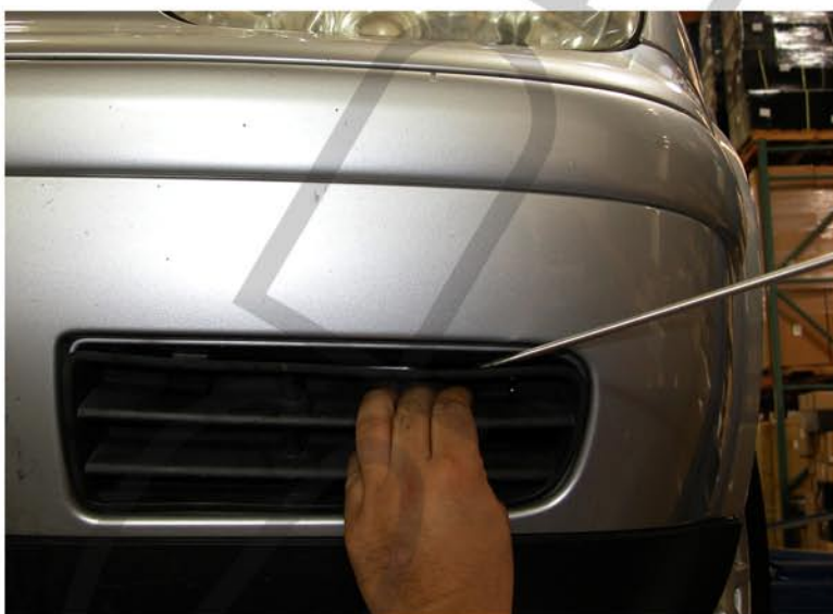
9. Remove the plastic cover from the fog light spot
