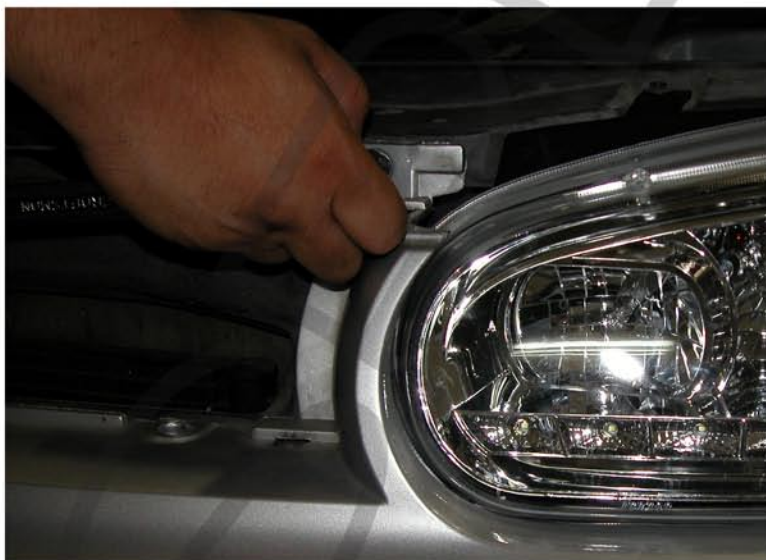
21. Reinstall the two clips removed from earlier
