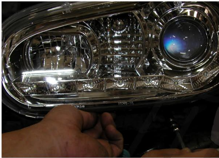
19. Install the bolts to the bottom of the headlight
