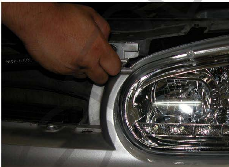
21. Reinstall the two clips removed from earlier
