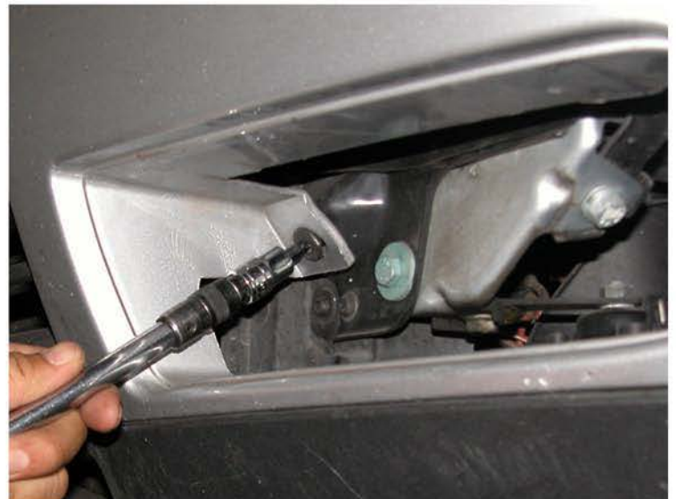
22. Install the bolt to the fog light opening
