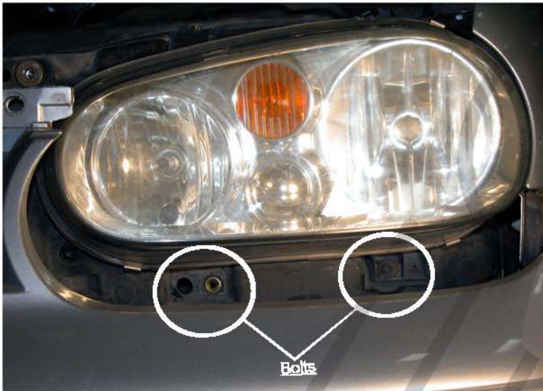
13. Use 8mm socket to remove the two bolts from the bottom of the headlight
