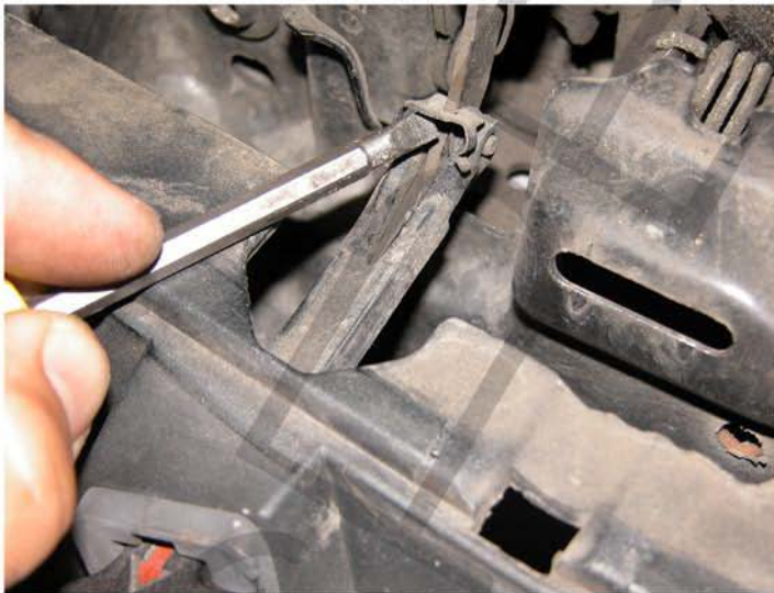
3. Use a flat-tip screwdriver to unlock the clip
