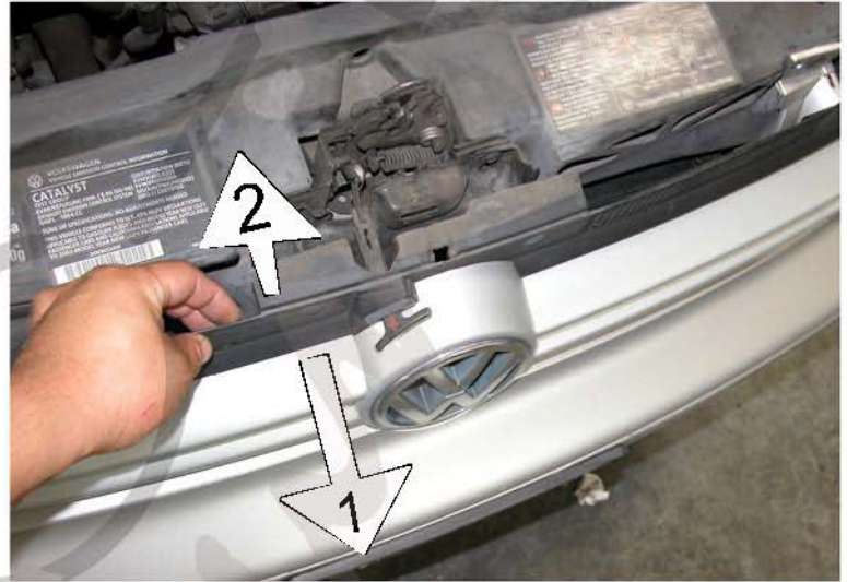
2. Pull the plastic to the front and remove by following the arrow
