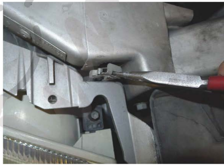
9. Remove the (2) metal clips
