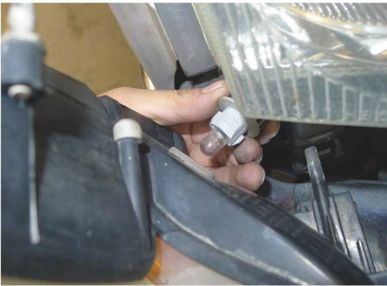
5. Remove the light socket
