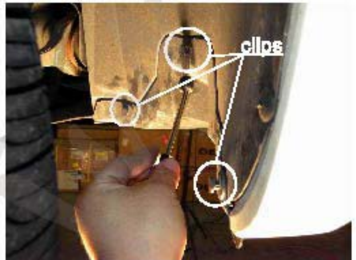
8. Remove three clips near the wheel well (Both side)
