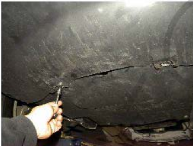
7. Using drive ratchet to remove the 10mm bolts
