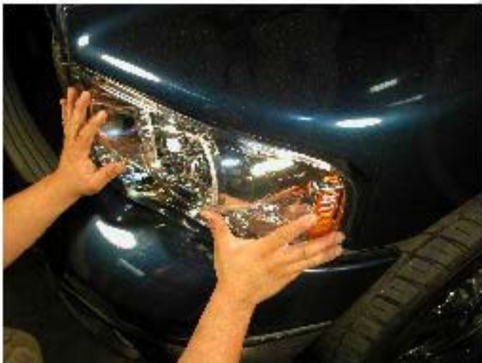
26. Install the new headlights
