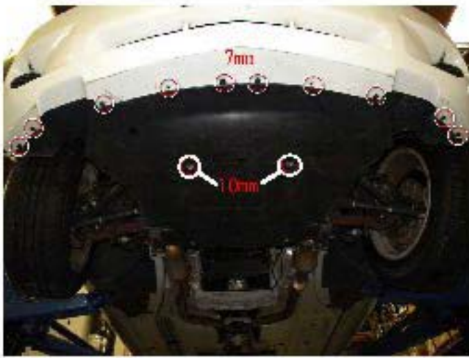
5. Remove ten 7mm bolts and two 10mm bolts
