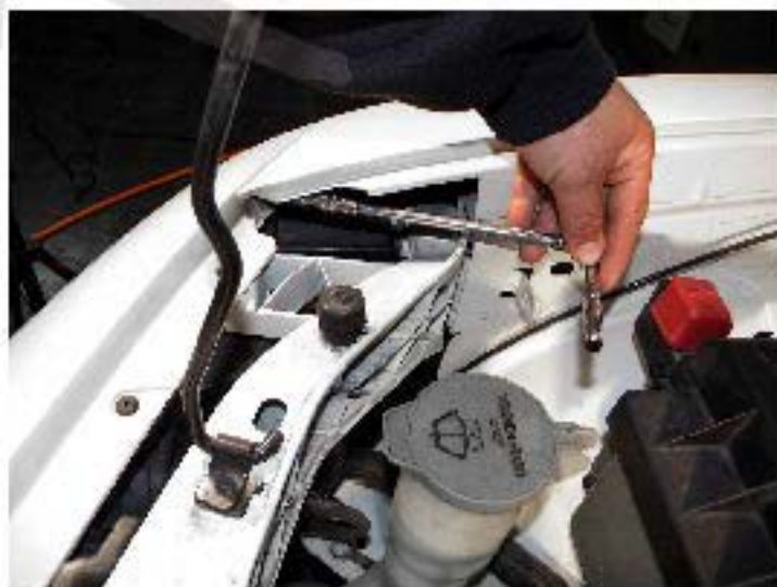
4. Remove one 10mm bolt by using 1/2" drive ratchet (Both side)
