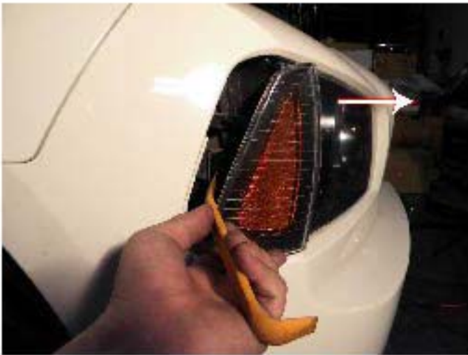
17. Pull out the corner light (Both side)
