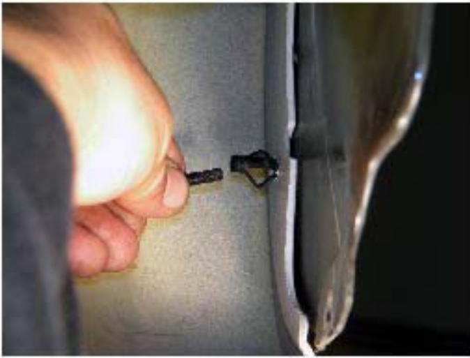
11. Pull out the screw inside the bumper
