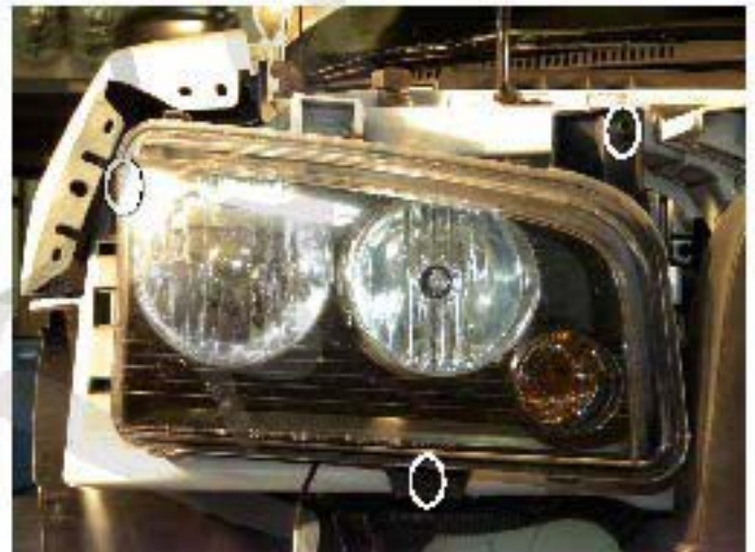
20. Remove three headlight bolts
