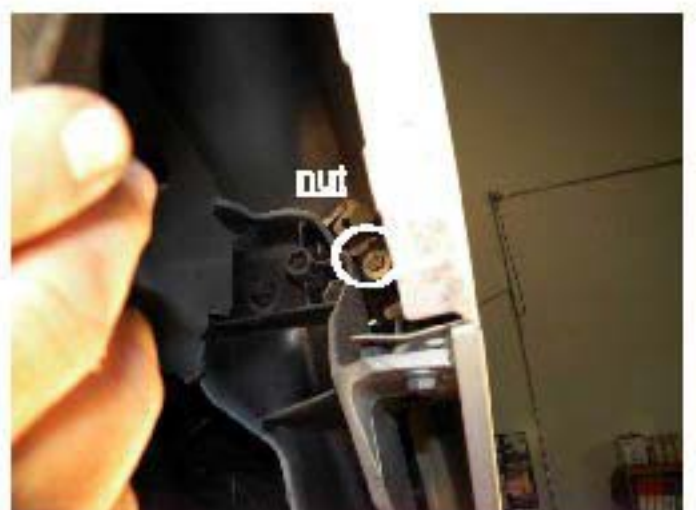
16. Remove one 10mm nut (Both side)
