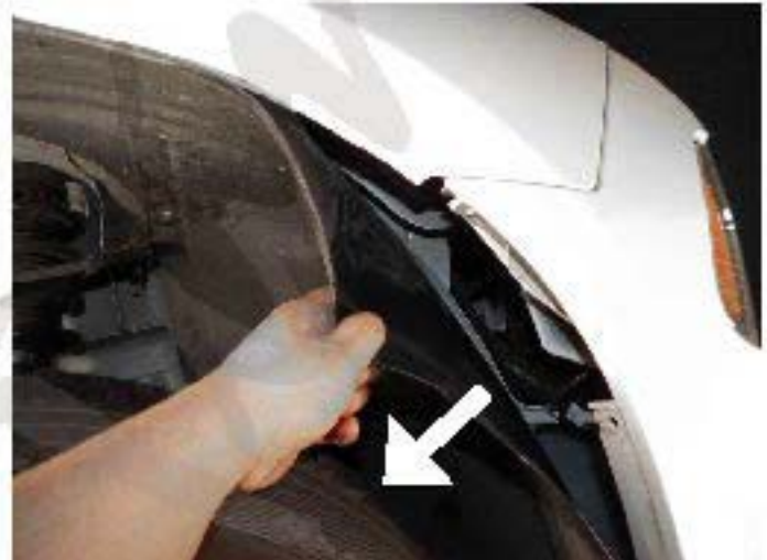
14. Pull out the cover (Both side)
