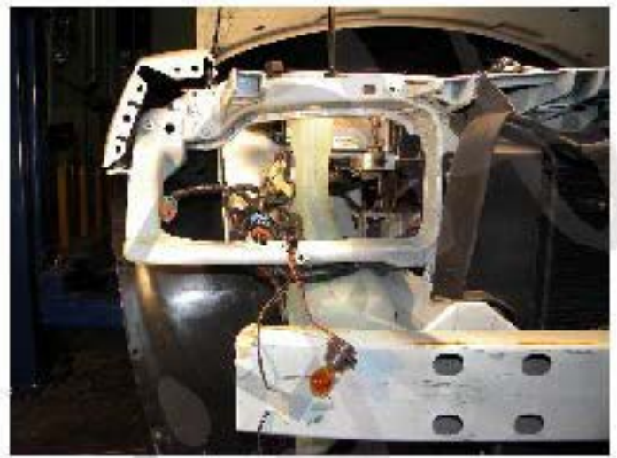
25. Connect new headlights to wire harness
