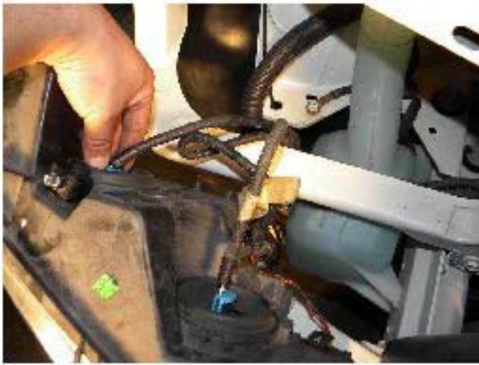
24. Disconnect all connectors from the headlight
