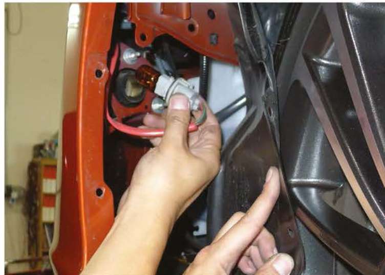
10. Remove the turn signal light socket
