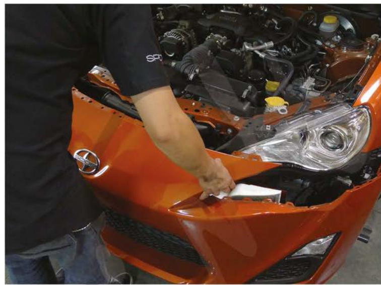
18. Remove the front bumper
