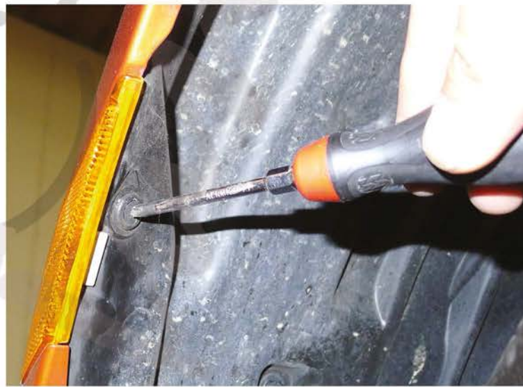
8. Remove the plastic clip
