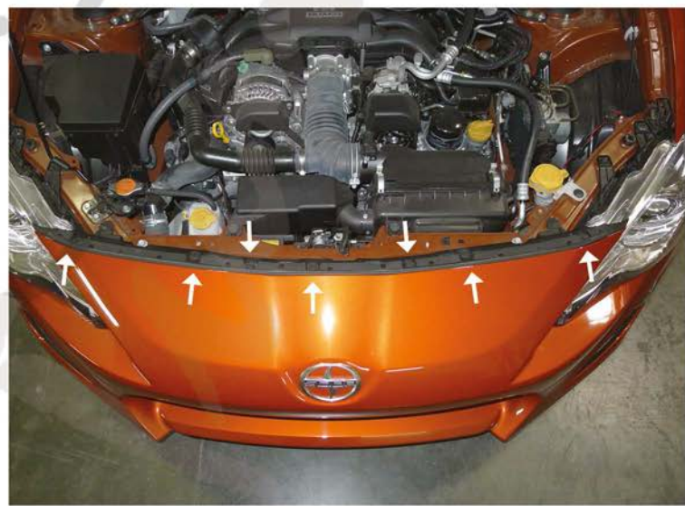
14. (5) 10mm bolts and (2) plastic clips location
