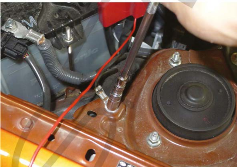
39. Remove the ground bolt
