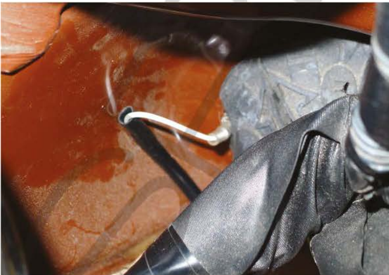
45. White wire through the rubber grommet
