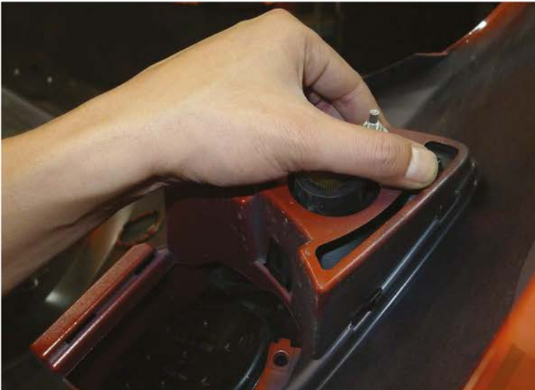
19. Release the mounting tabs on the fog light hole cover
