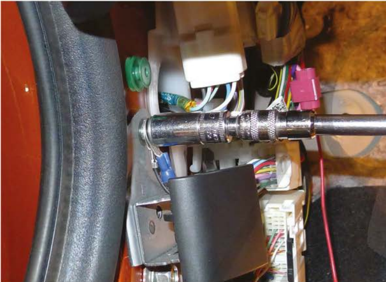
31. Tighten the 10mm hood latch release mounting bolt
