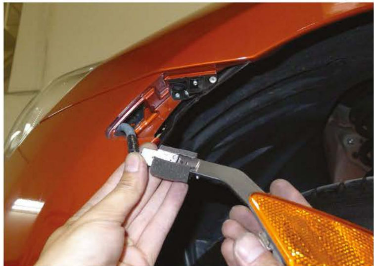
64. Connect the bumper light harness
