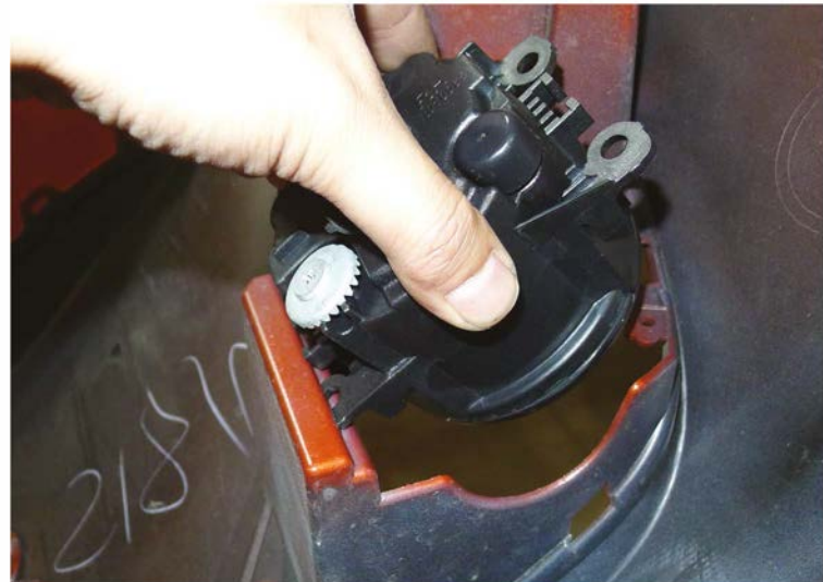
22. Slide the inner mounting tabs in to the slots
