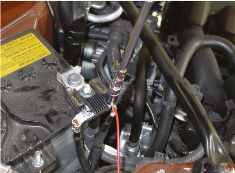
37. Attach the red wire from the fog light harness to the positive terminal and tighten
