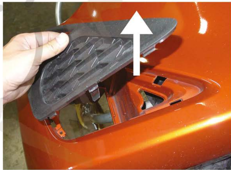
20. Remove the fog light hole cover
