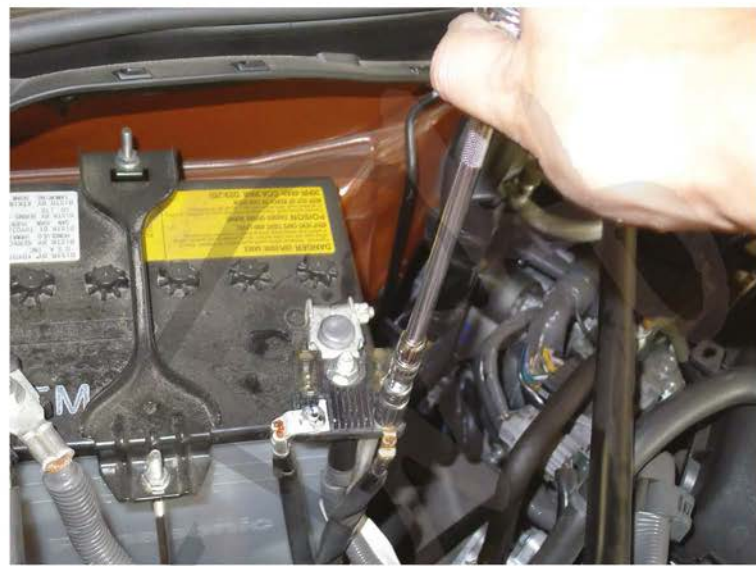
36. Remove the 10mm nut from the positive terminal
