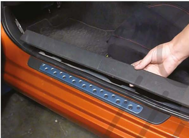
55. Replace the side sill trim moulding
