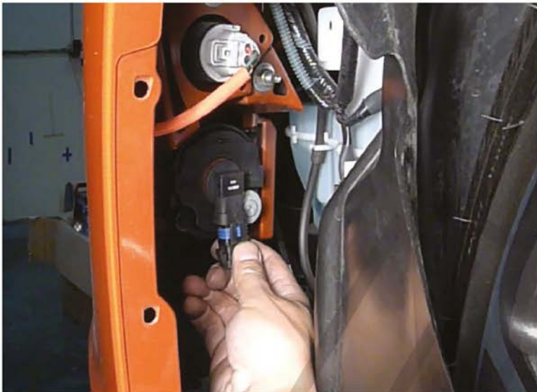
66. Connect the fog light harness
