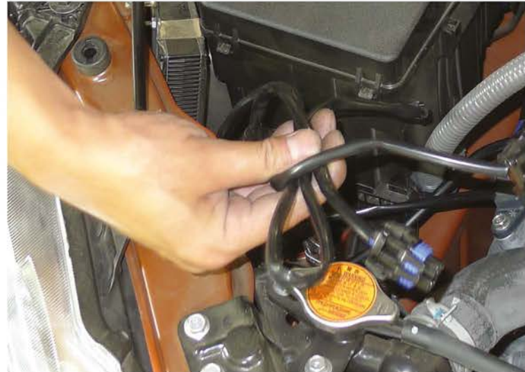
46. Run the fog light connector ends of the fog light harness toward the front of the car along the factory harness
