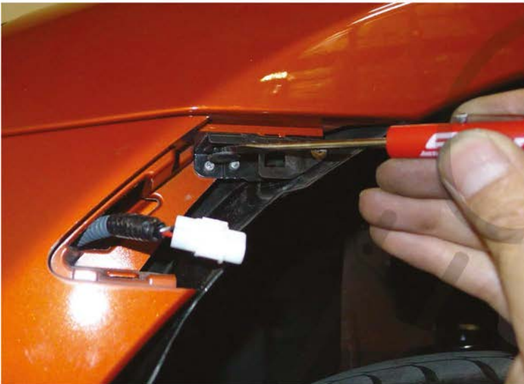
13. Remove the plastic clip
