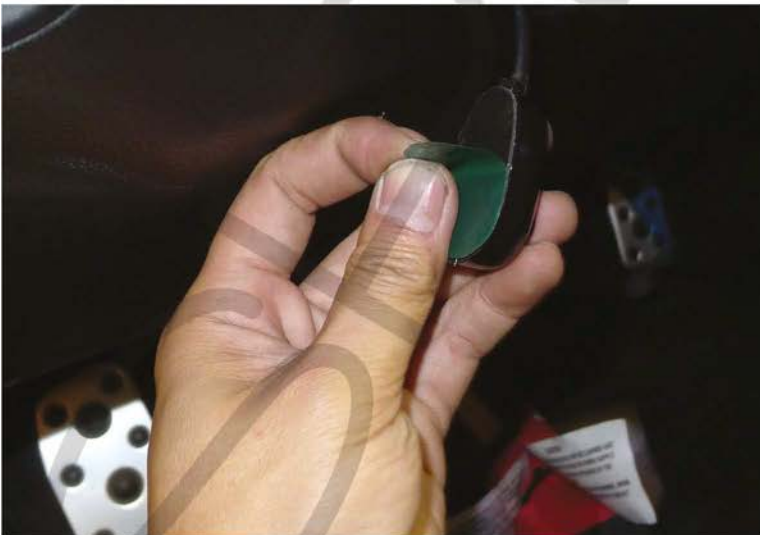
33. Peel off the adhesive back on the switch
