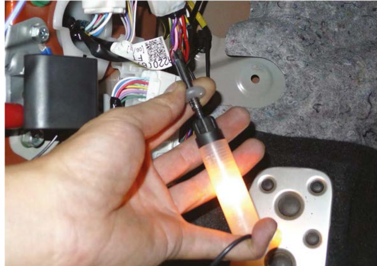
28. Turn on the ignition to ACC and find the ACC power wire with the test light
