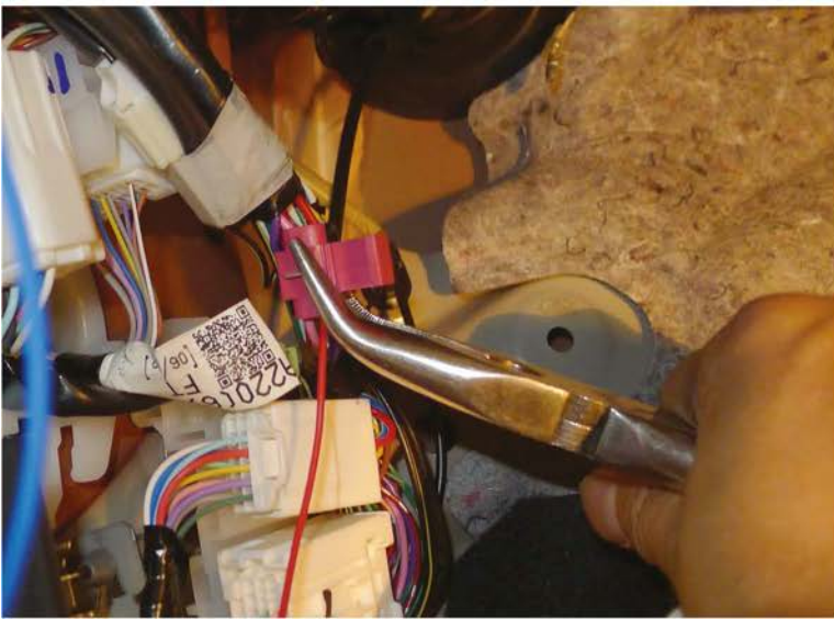
29. Connect the red wire on the fog light switch harness to ACC power wire with the quick connector
