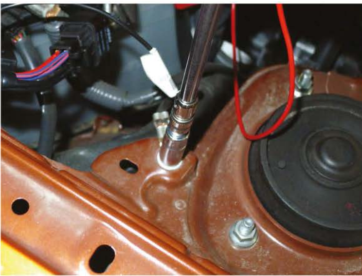
41. Tighten the 10mm ground bolt
