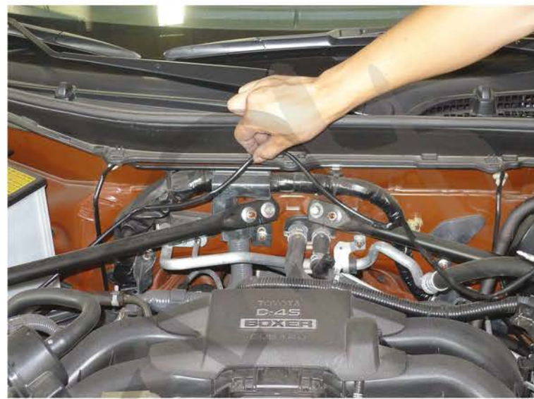
42. Run the white wire across the firewall along the factory harness
