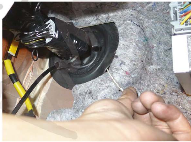
50. Pull the white wire through the firewall
