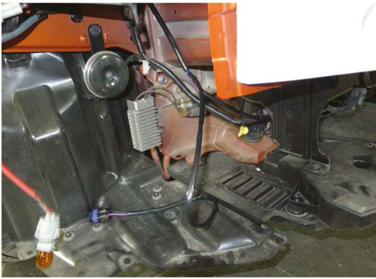
47. Fog light harness under the passenger side headlight
