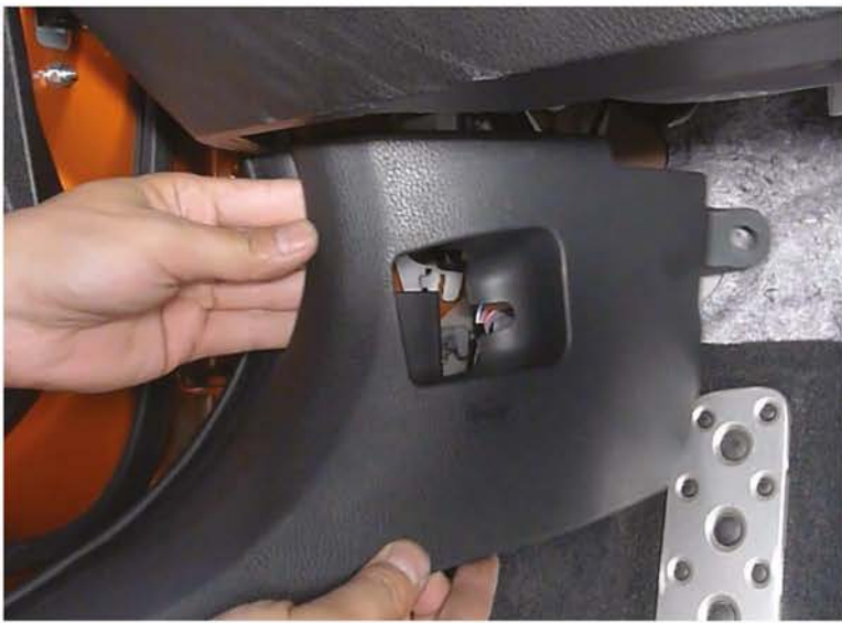
53. Replace the kick panel moulding
