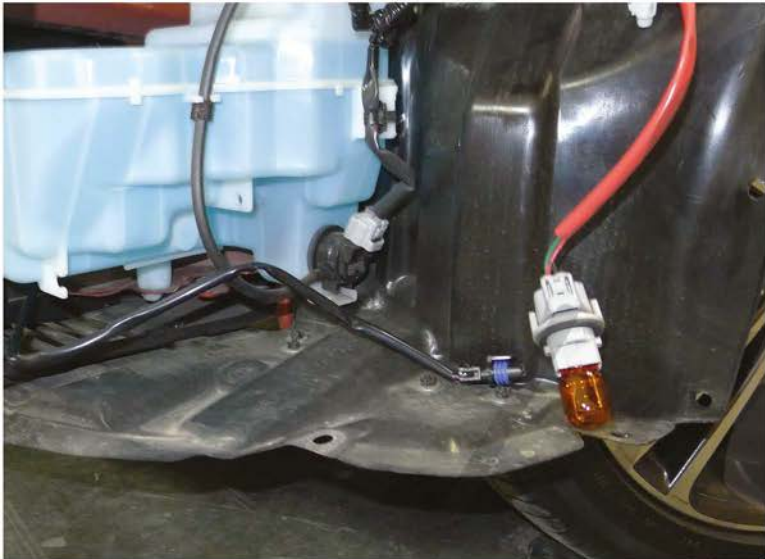
49. Connector should end up under the driver side headlight
