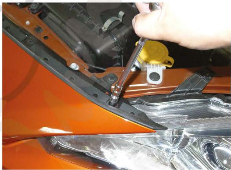
62. Tighten (5) 10mm bolts
