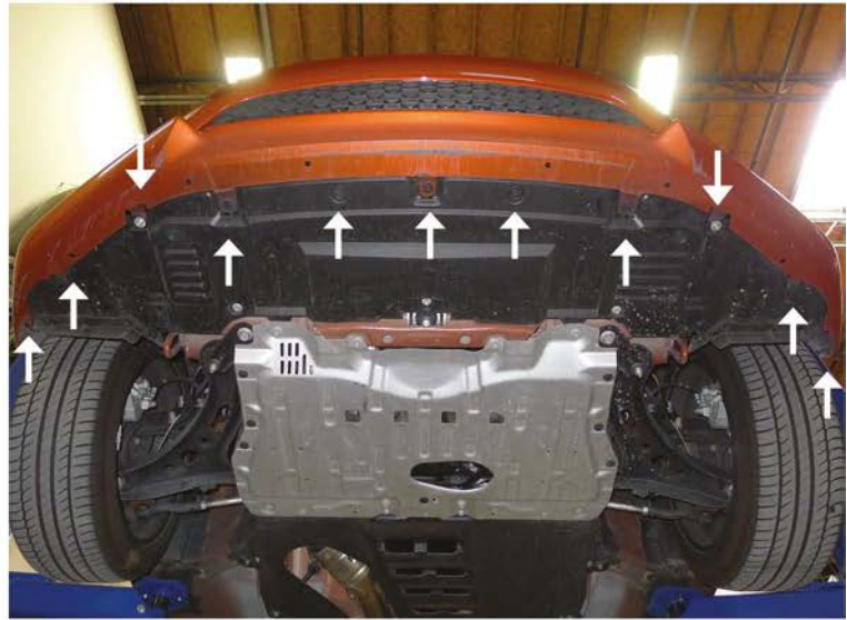
2. (9) plastic clips and (2) 10mm bolts location
