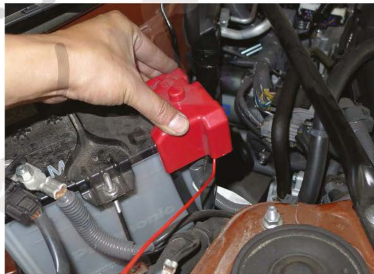
38. Replace the positive terminal cover
