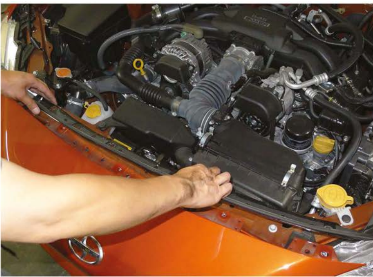
17. Remove the metal bracket
