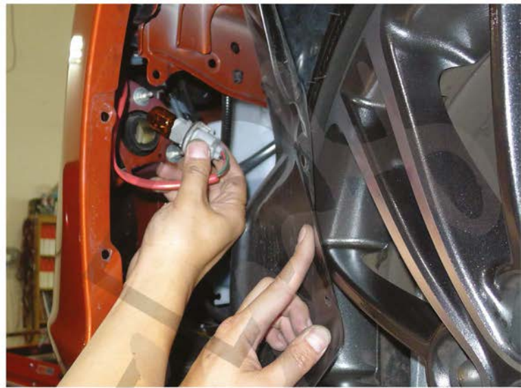
65. Replace the turn signal light socket
