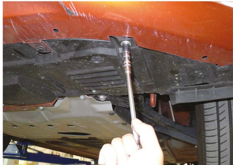
69. Tighten (2) 10mm bolts
