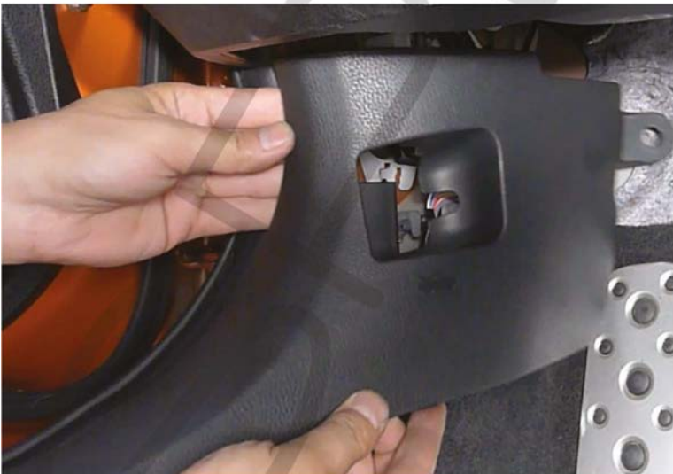
27. Remove the kick panel moulding
