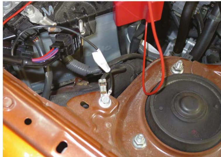
40. Attach the ground wire to the ground bolt
