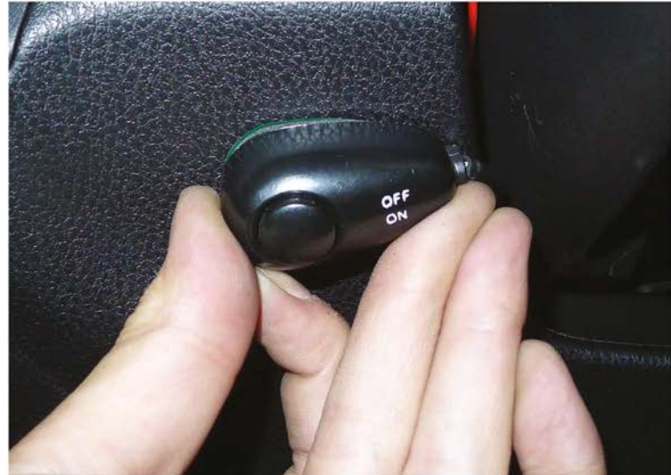
34. Attach the switch to dash panel, or chosen spot in the car.
