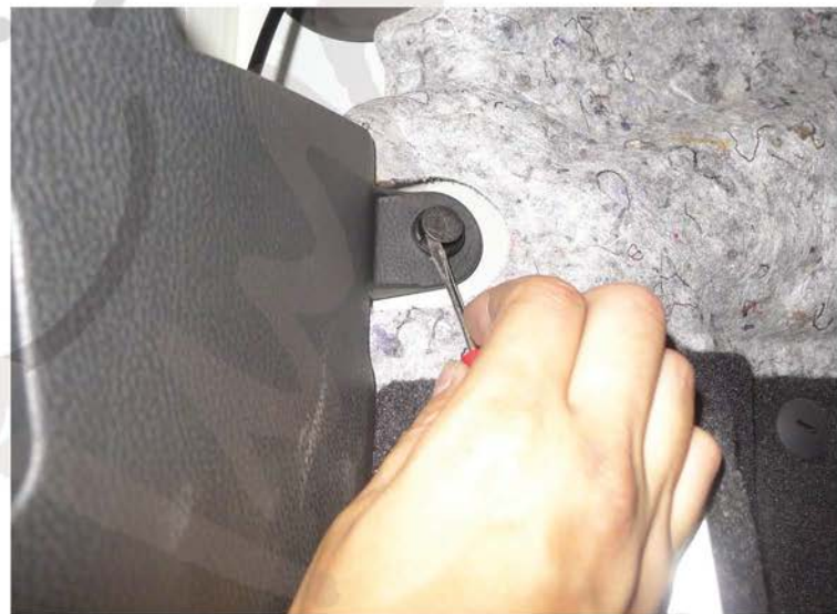
26. Remove the plastic clip
