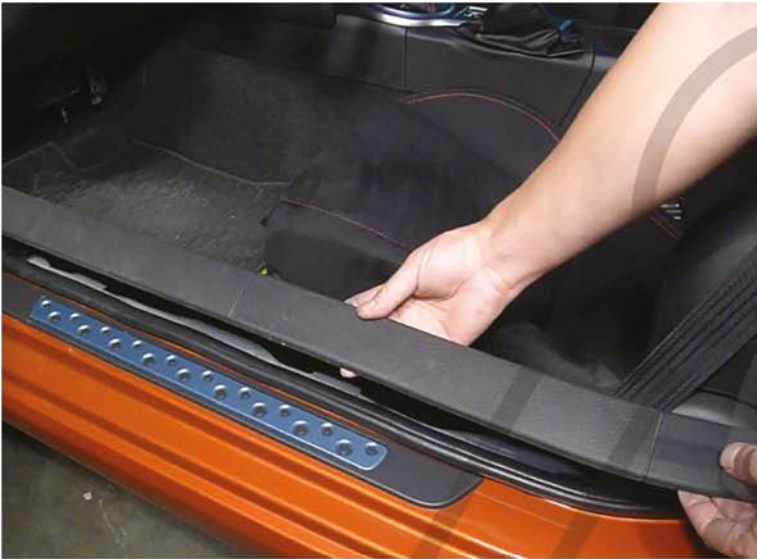
25. Remove the side sill trim moulding
