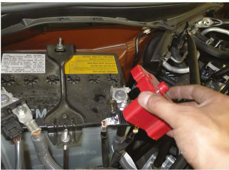
35. Remove the positive terminal cover
