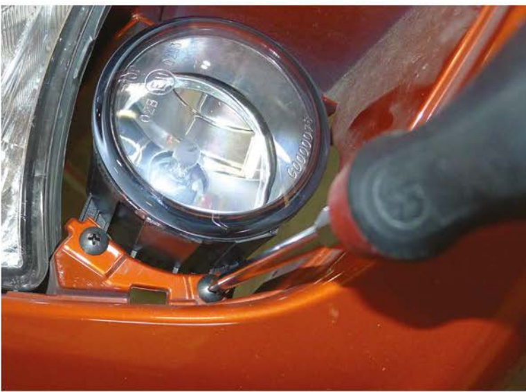
23. Tighten (2) phillips head screws
