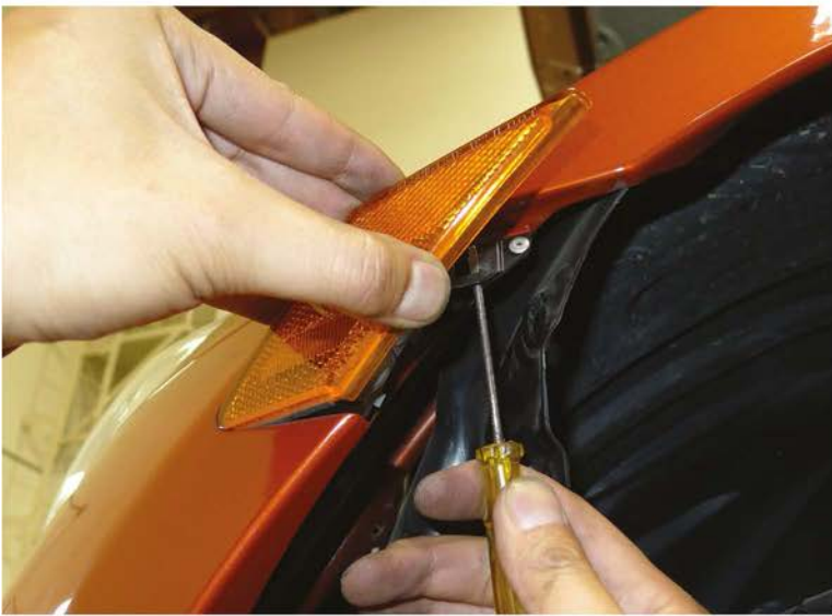
11. Remove the bumper light
