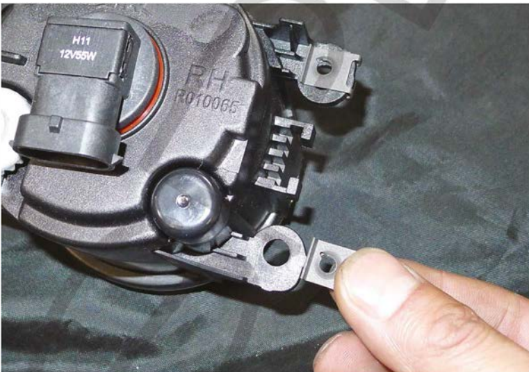
21. Place the spring nuts on the two outer mounting tabs on the fog lights
