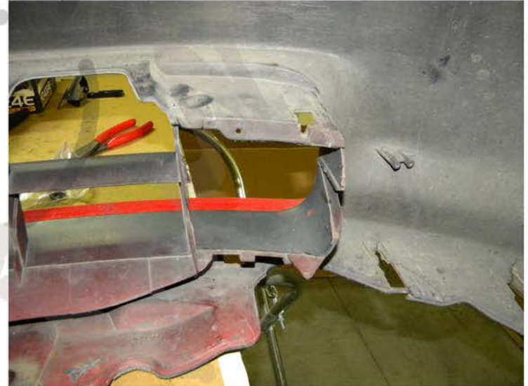
14. Center the rib removed
