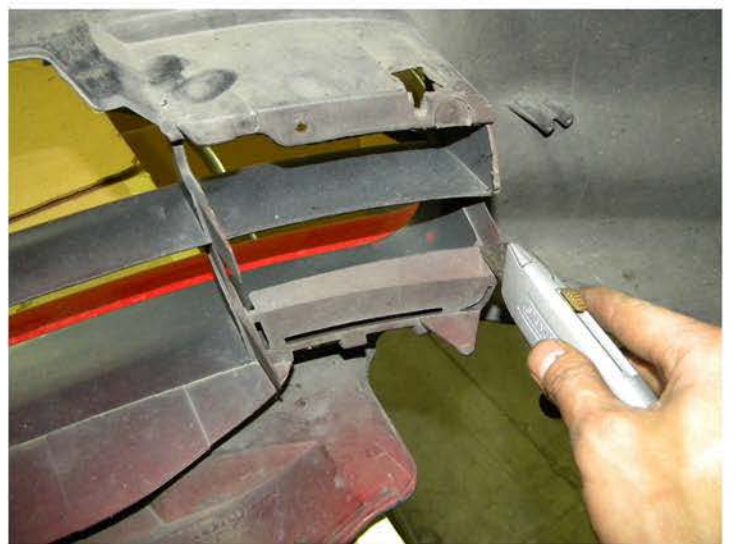
10. Remove the cut out from front the bumper
