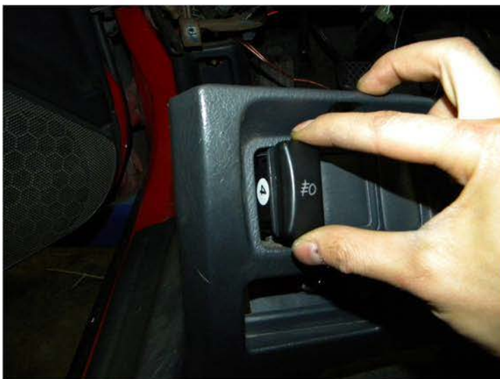
51. Replace the cover with a fog light switch
