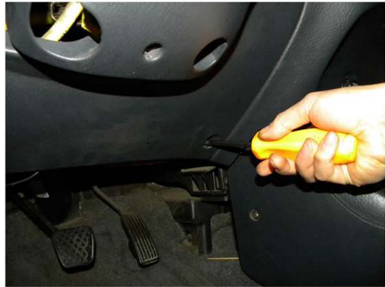
54. Tighten the (3) Phillips head screws
