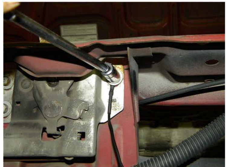
28. Connect the fog light harness ground wire to the 10mm bolt and tighten
