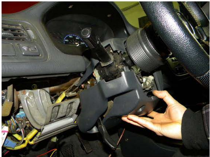
45. Remove the steering column cover
