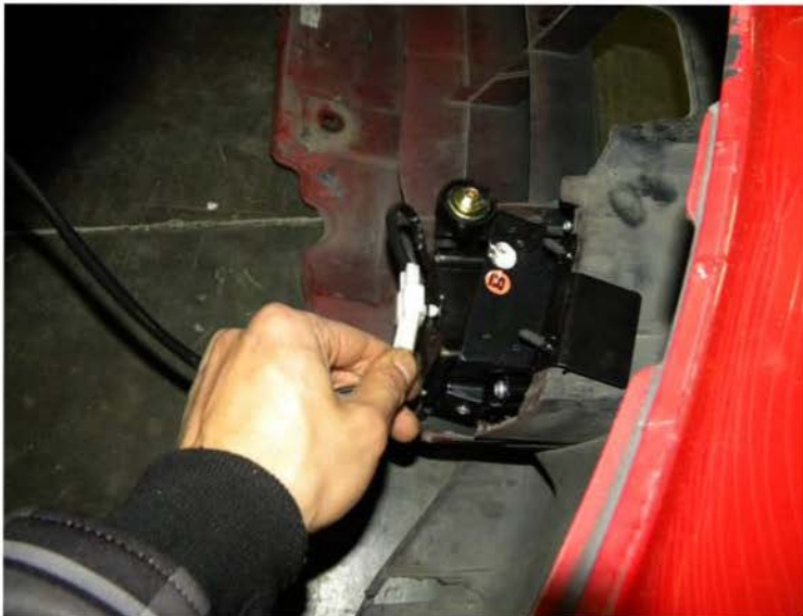
31. Connect the fog light to the fog light harness
