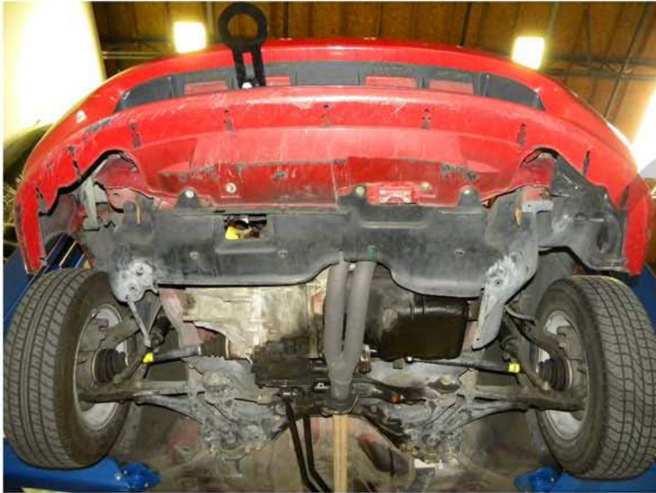
1. Under the bumper are the 10mm bolt locations
