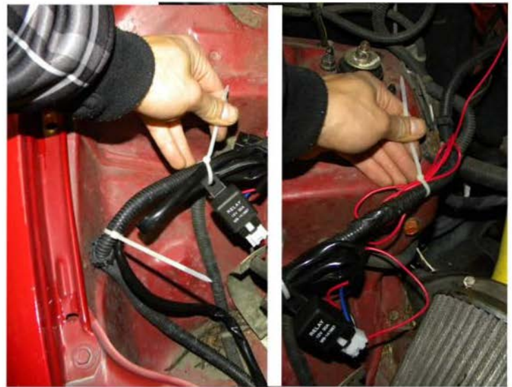
30. Zip the excess wiring and relay to the stock harness
