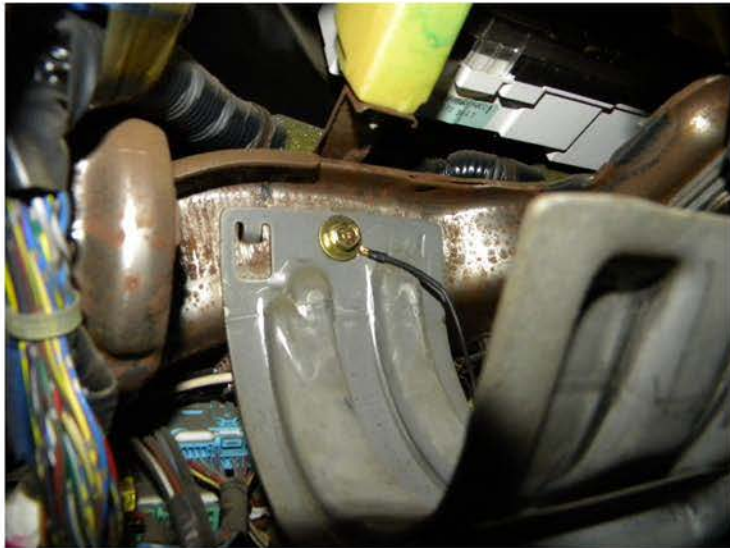
43. Switch the harness ground wire
