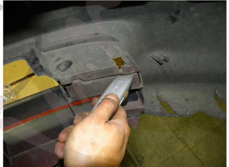
8. Remove the cut out from the front bumper
