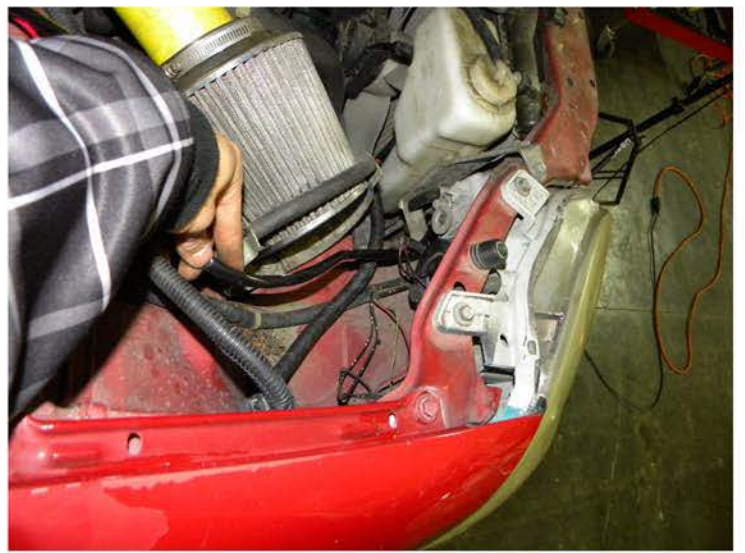
22. Run the fog light harness though the bulkhead along the stock harness
