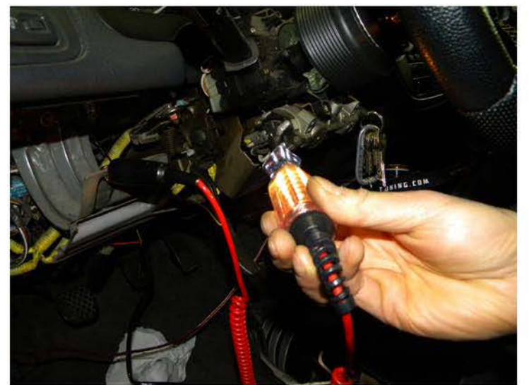
46. Locate the ACC power wire with the test light
