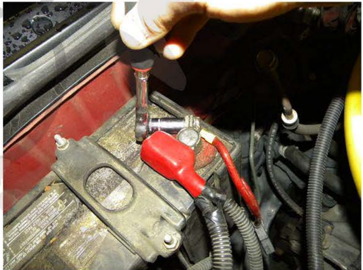
20. Remove the 10mm bolt
