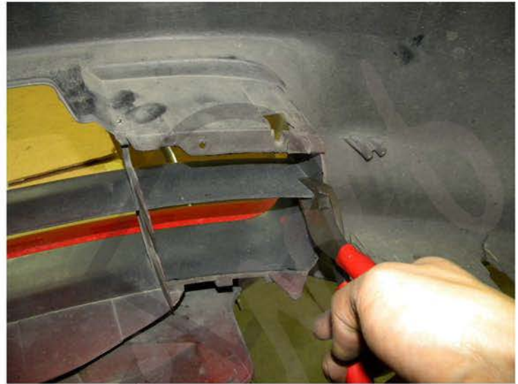
12. Cut the center rib with a cutter or a saw
