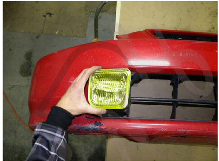
18. Place the fog light assembly into the position
