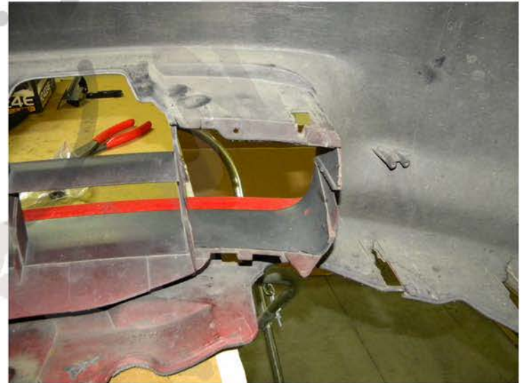
14. Center the rib removed
