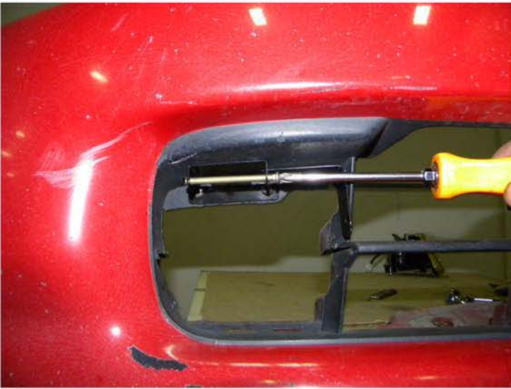
17. Tighten the phillips head screws
