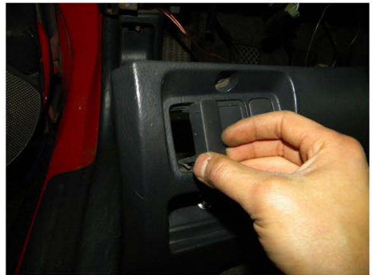
50. Remove the plastic cover on the lower dash panel
