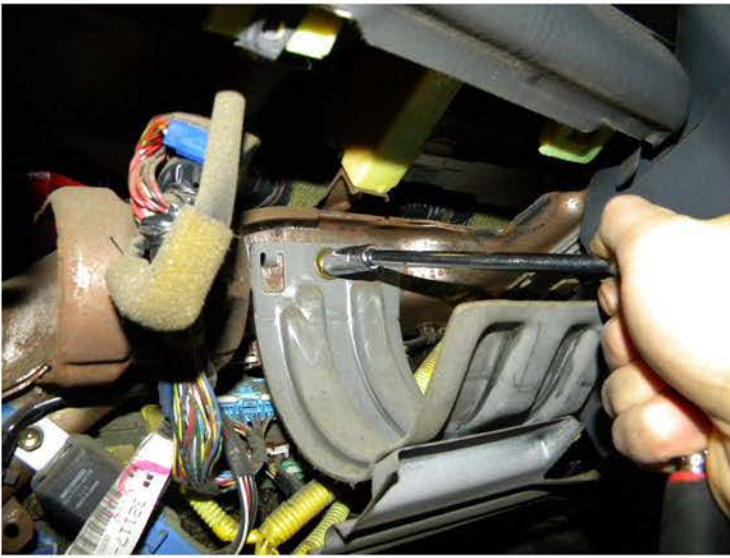
41. Remove the 10mm bolt
