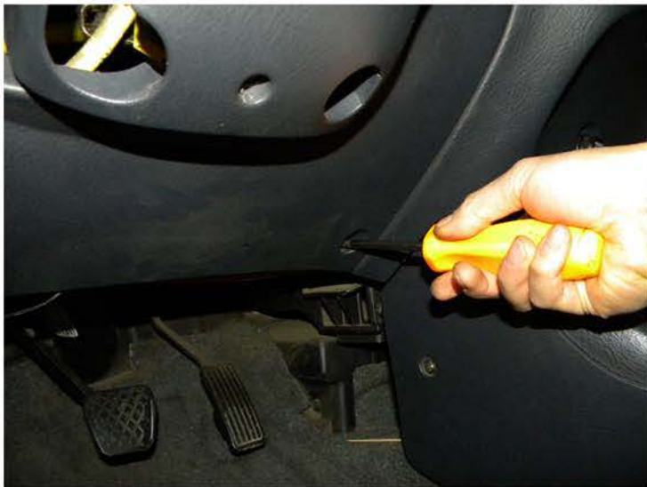
37. Remove the (3) phillips head screws from the lower dash panel
