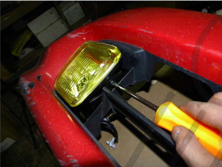
19. Tighten the phillips head screw
