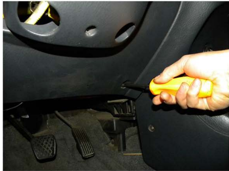
54. Tighten the (3) Phillips head screws
