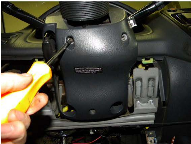
49. Tighten the (3) phillips head screws
