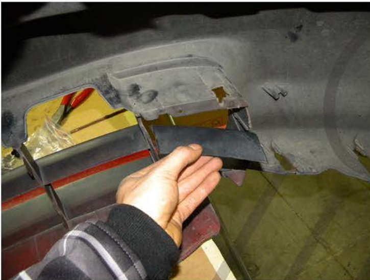
13. Remove the center rib
