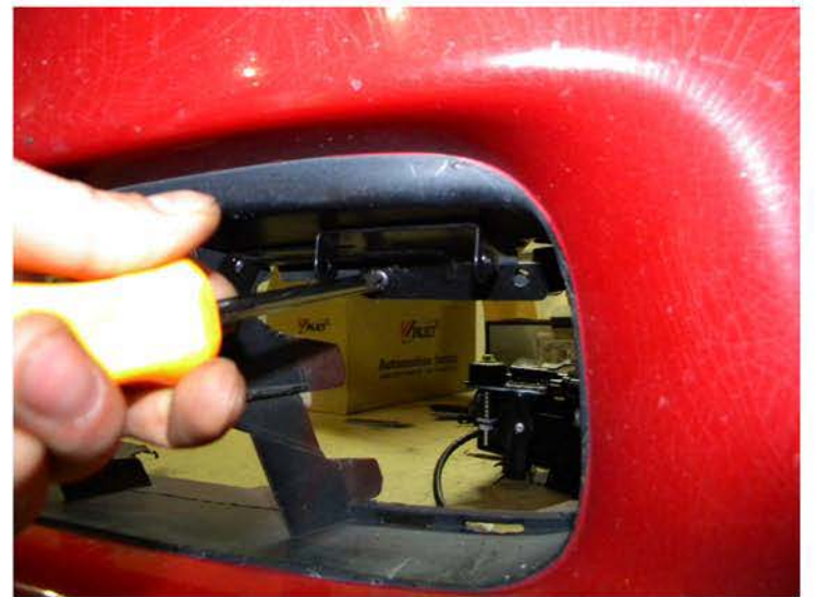
16. Fasten the mounting brackets onto the bumper with the (2) phillips head screws
