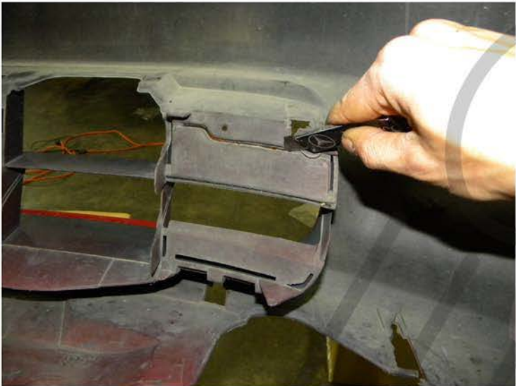
7. Remove the cut out from the front bumper
