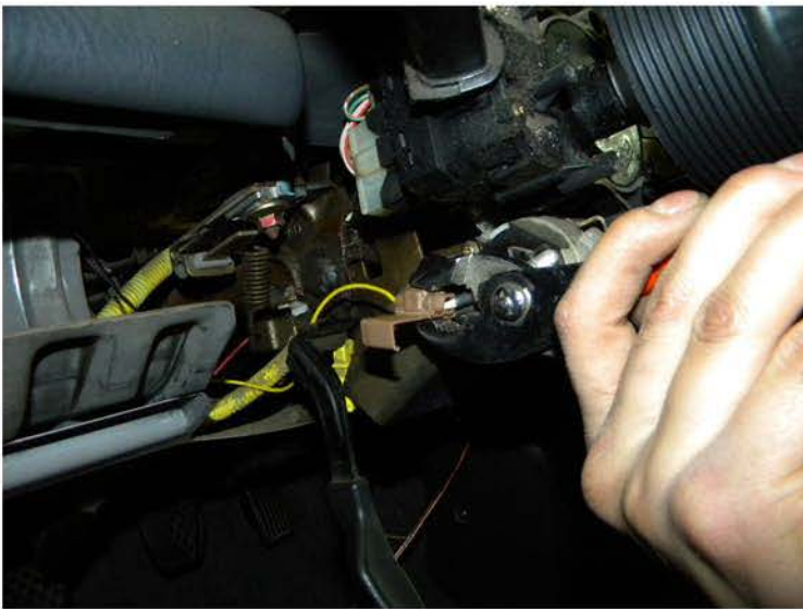
47. Connect the yellow wire on the switch harness to the ACC power wire using a quick connector
