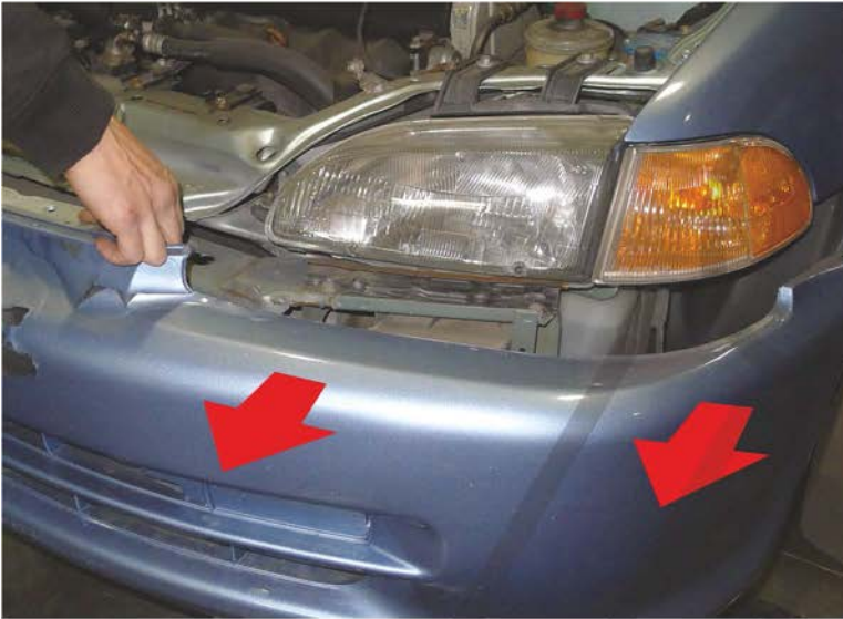
7. Remove the front bumper
