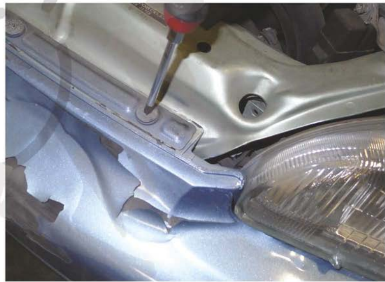
26. Tighten the (5) phillips head screws
