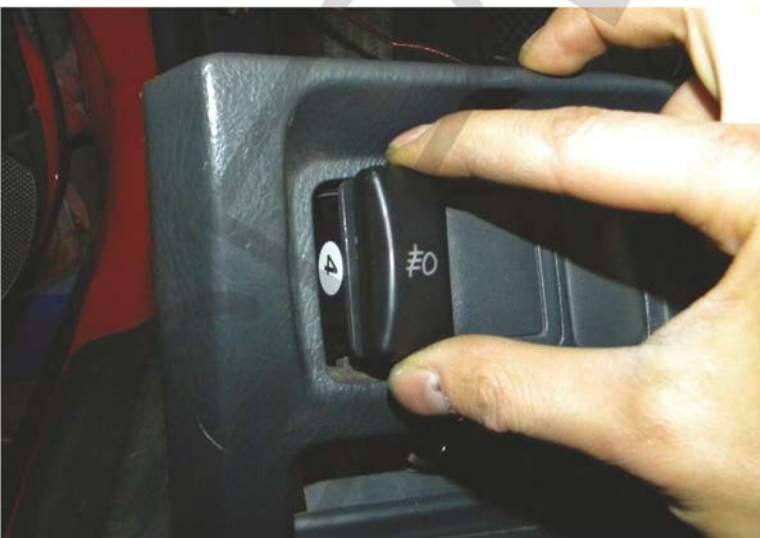
45. Replace the cover with the fog light switch
