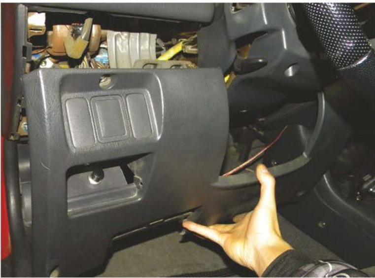
47. Replace the lower dash panel
