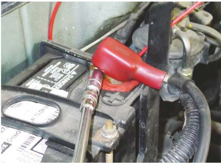
11. Loosen the 10mm nut on the positive battery terminal
