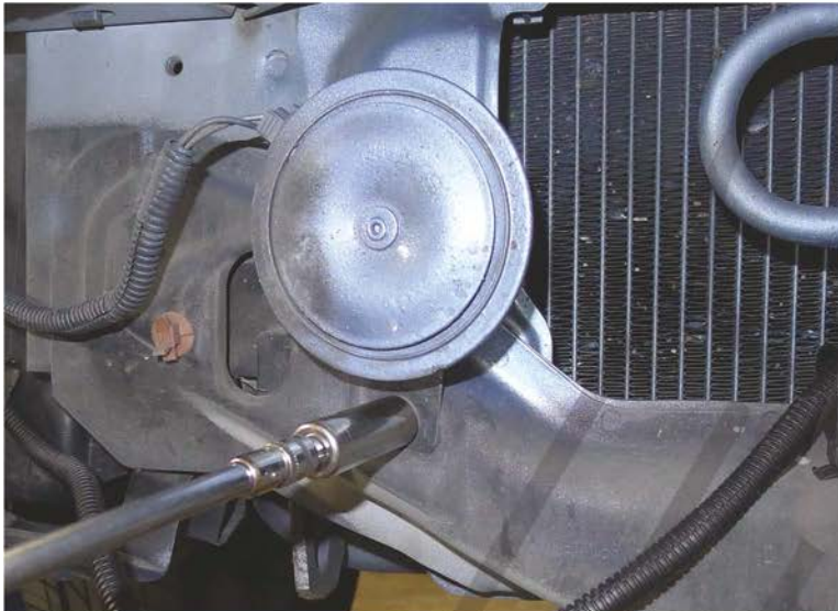
13. Loosen the 10mm bolt
