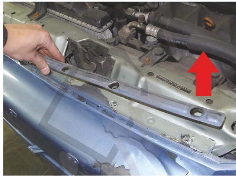
6. Remove the metal bracket
