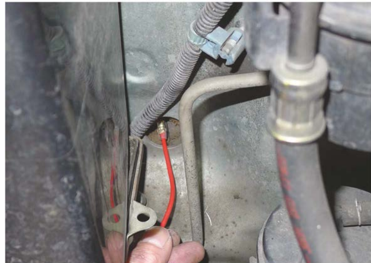
16. Run the extension wire through rubber grommet to the cockpit
