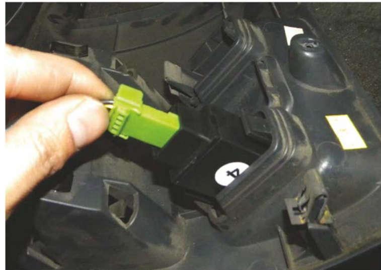
46. Connect the switch harness to the fog light switch
