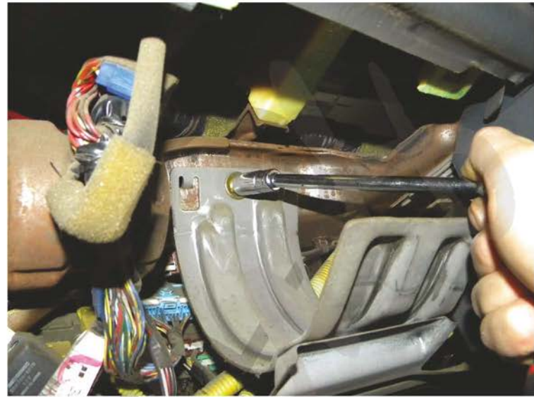
36. Remove the 10mm bolt
