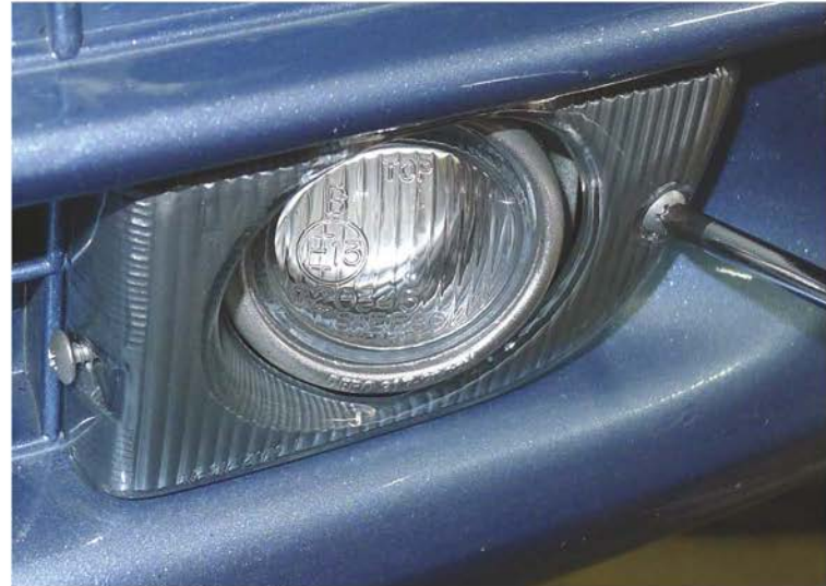
22. Secure the fog light bezel with the (2) phillips head screws
