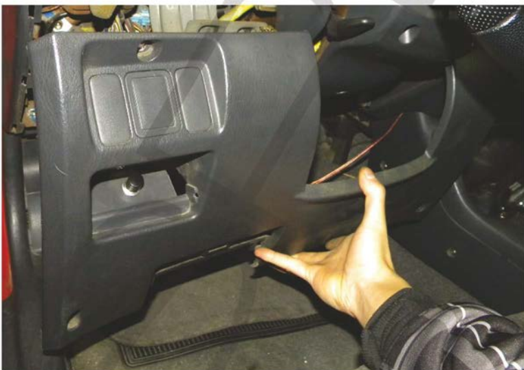
33. Remove the lower dash panel
