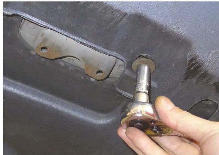
28. Tighten the (2) 10mm bolts
