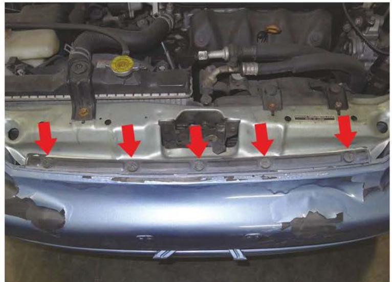
4. (5) phillips head screws location
