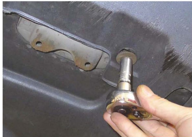
28. Tighten the (2) 10mm bolts
