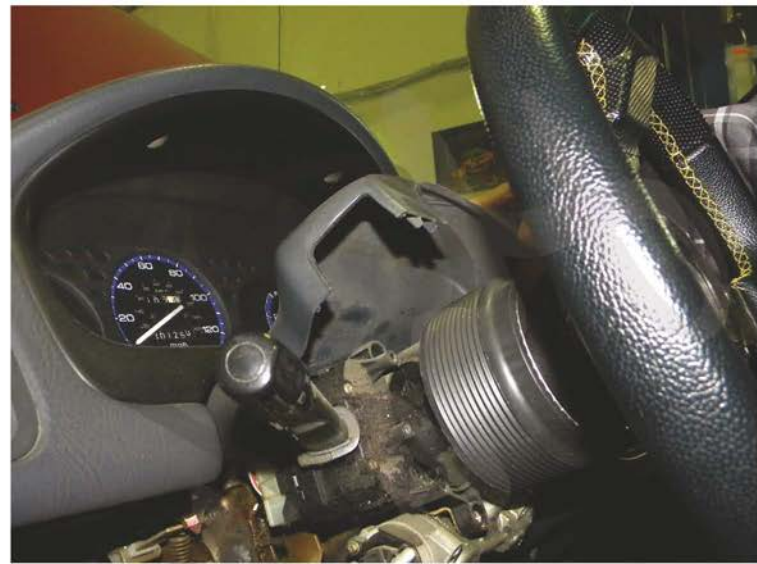
42. Replace the steering column cover
