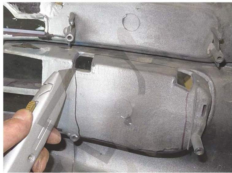
18. Cut the area previously marked
