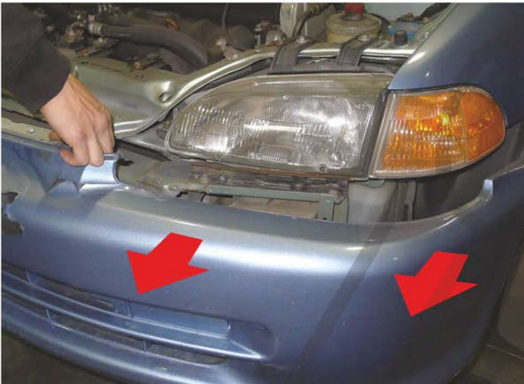
7. Remove the front bumper
