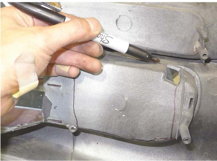
17. Mark the area to be cut with the marker
