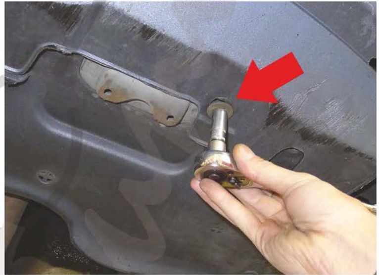
2. Remove the (2) 10mm bolts
