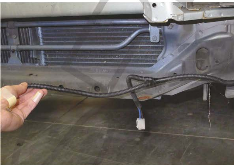
9. Run the fog light harness across the front of the bulkhead
