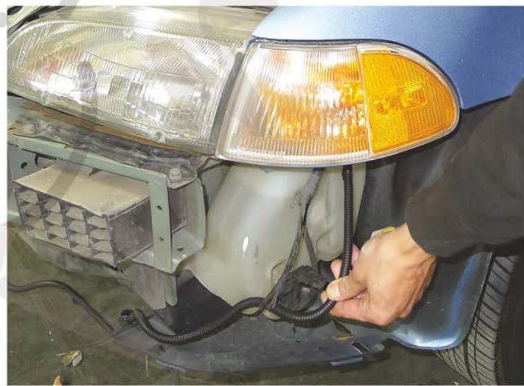
8. Run the fog light harness through the bulkhead
