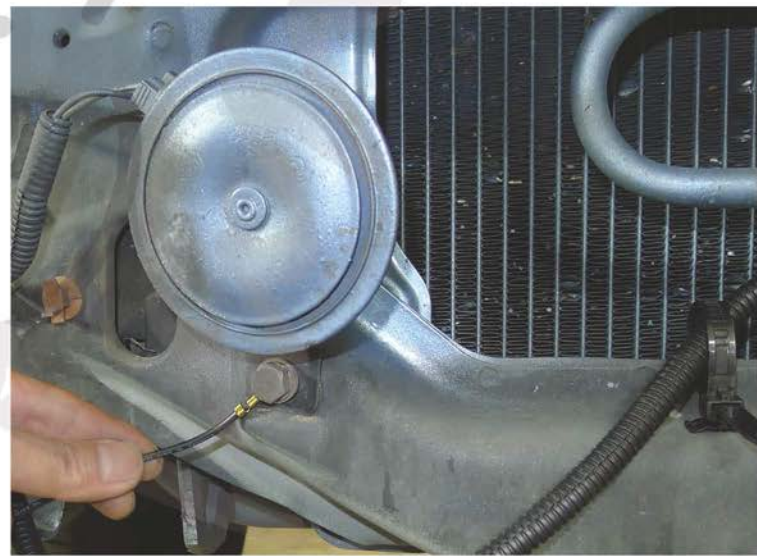
14. Place the fog light harness ground wire behind 10mm bolt
