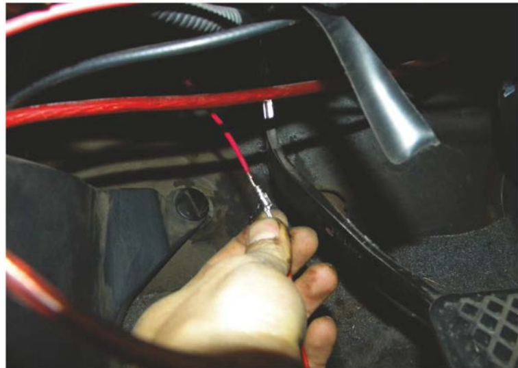
34. Connect the switch harness
