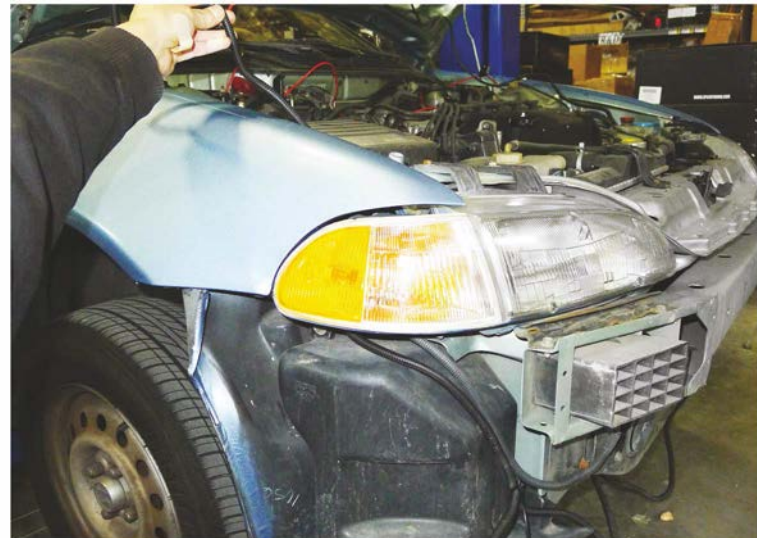
10. Run the fog light harness back through the bulkhead towards the engine bay
