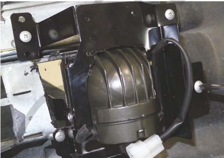
21. Secure the fog light assembly onto the bumper with the (4) phillips head screws
