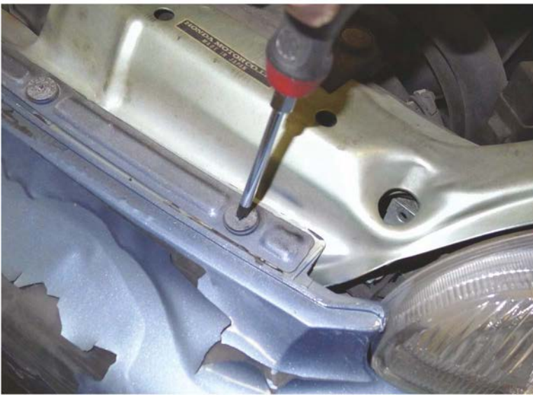
5. Remove the (5) phillips head screws
