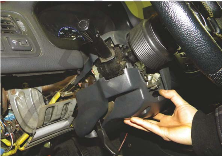
39. Remove the steering column cover
