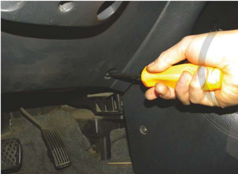
31. Remove the (3) phillips head screws from the lower dash panel
