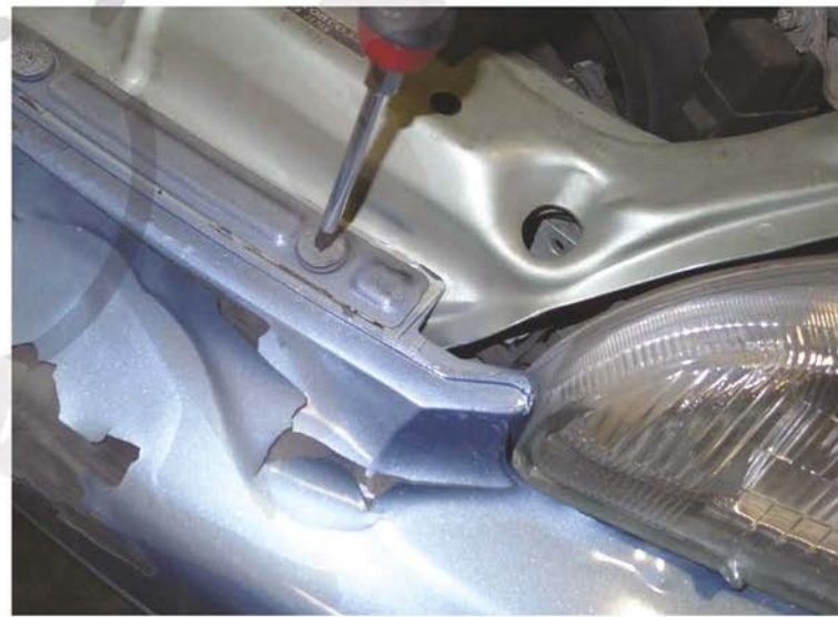
26. Tighten the (5) phillips head screws
