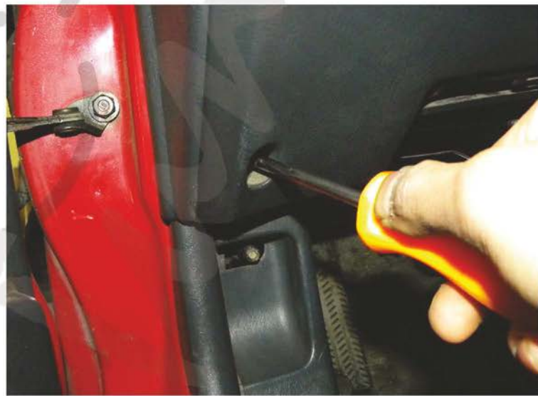
32. Remove the (3) phillips head screws from the lower dash panel
