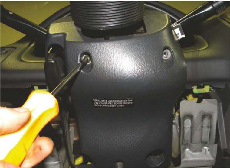
43. Tighten the (3) philip head screws
