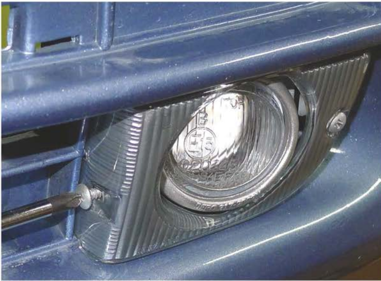
23. Secure the fog light bezel with the (2) phillips head screws
