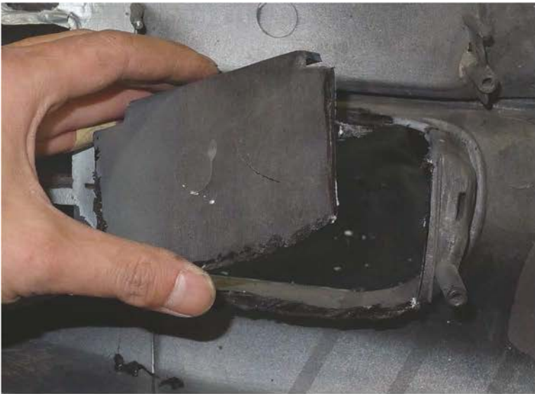
19. Remove the cut portion of the bumper
