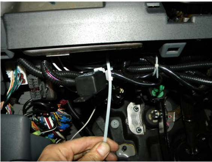
35. Zip the excess wire onto the factory wire harness
