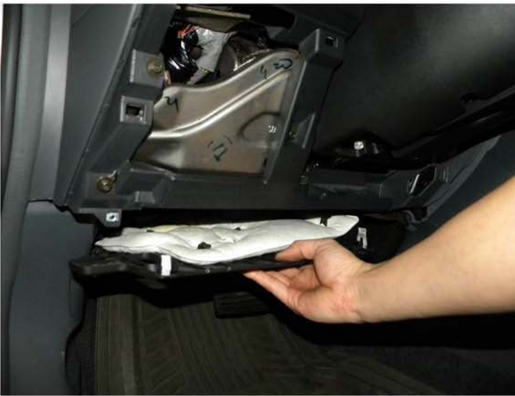
29. Remove the dashboard under cover
