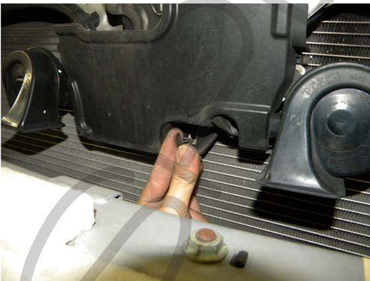
21. Remove the plastic clip
