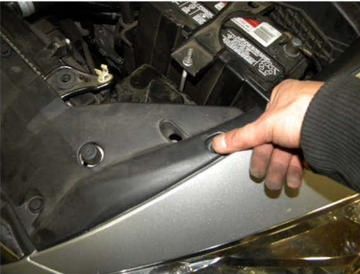
49. Replace the (10) plastic clips
