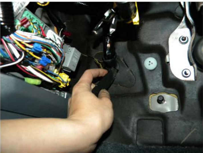
33. Cut a slit in the rubber grommet
