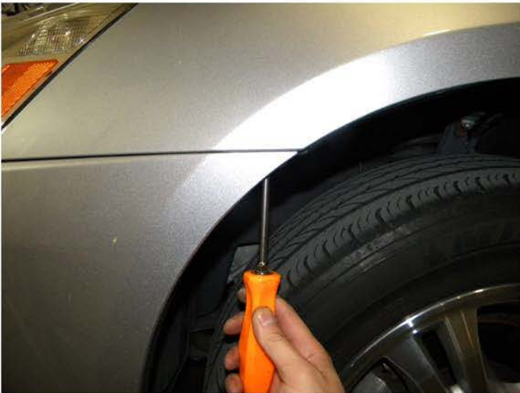
7. Remove the phillips head screw
