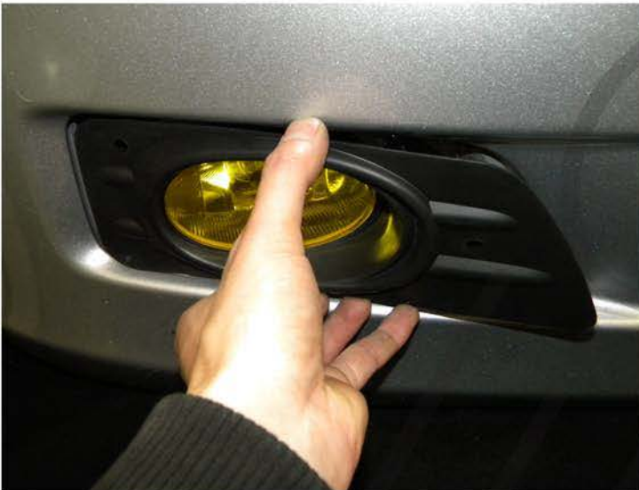
19. Place the fog light in the fog light hole
