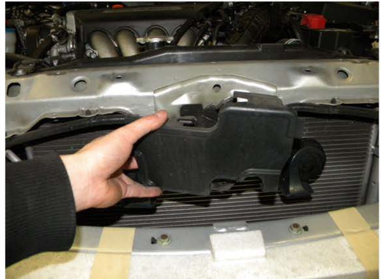
22. Remove the hood latch cover
