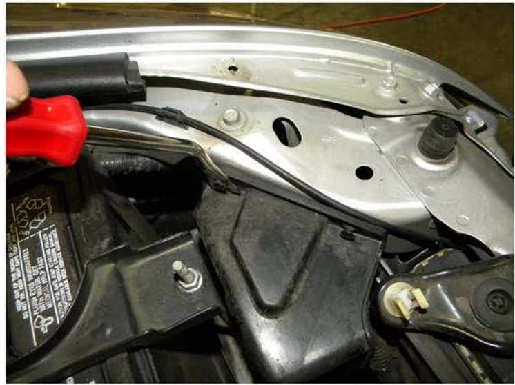
42. Remove the (2) plastic clips
