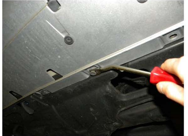
4. Remove the (6) plastic clips
