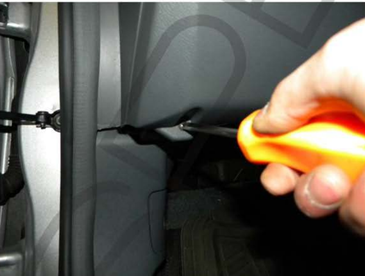
27. Remove the phillips head screw
