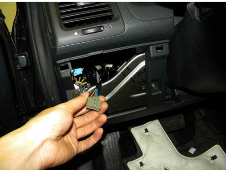
63. Pull the switch connector through the hole
