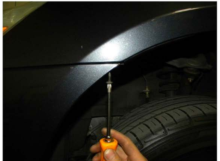
4. Remove the phillips head screw
