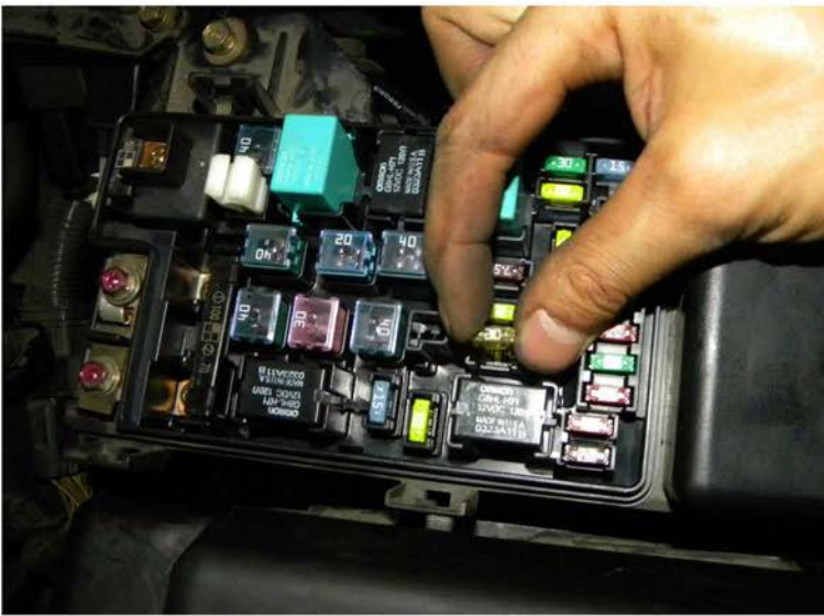
47. Place the 20 amp fuse in the slot 10
