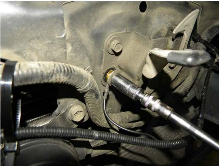
19. Secure the fog light harness ground cable, and tighten the 10mm bolt
