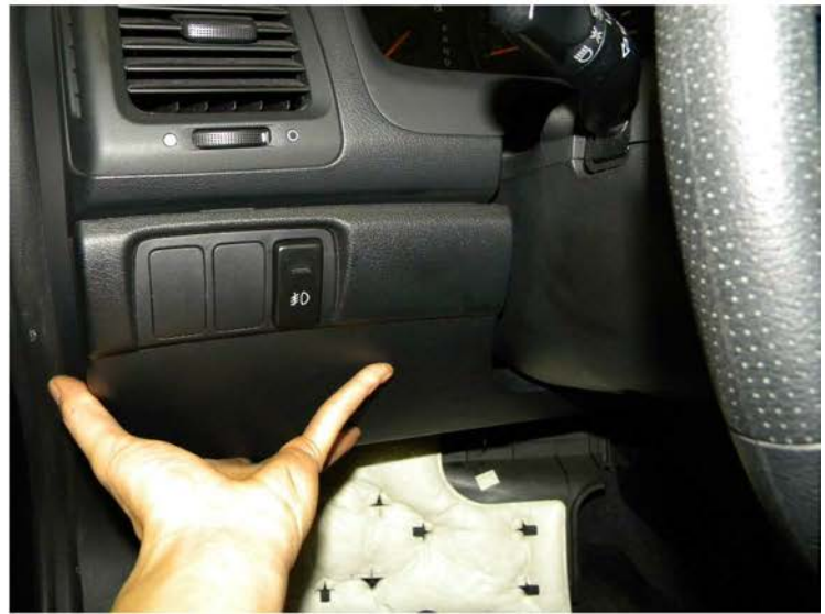
66. Replace the plastic panel
