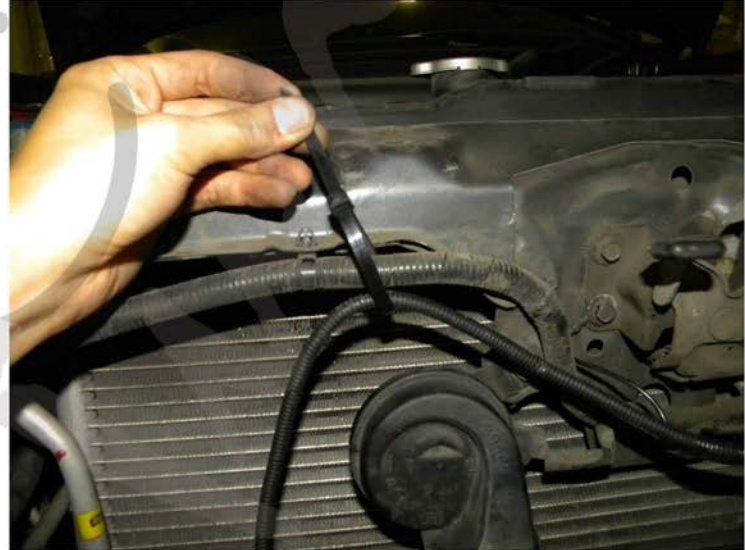
20. Zip tie the fog light harness to the factory harness
