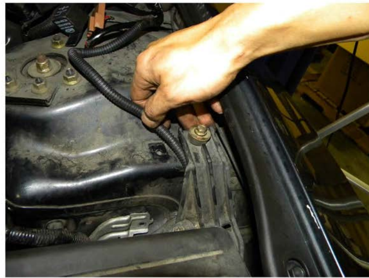
34. Slide the fog light harness under the airbox
