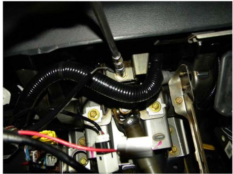
60. Attach the switch harness ground cable and tighten the 10mm bolt
