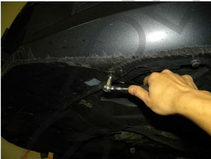
3. Remove the (4) 10mm bolts
