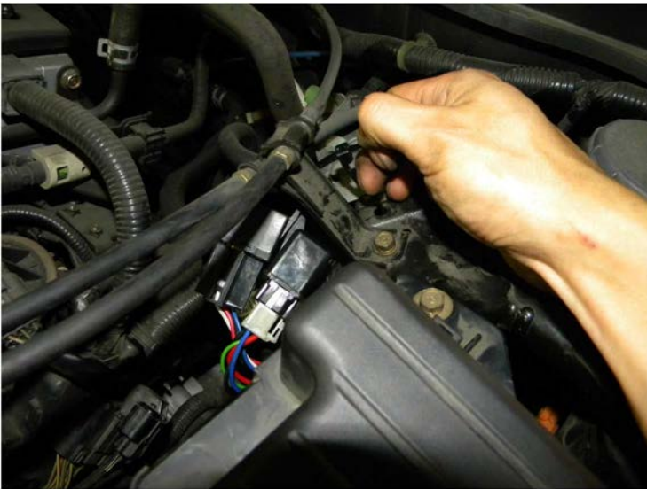
37. Zip tie relays
