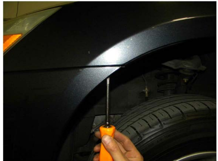
44. Replace the phillips head screw
