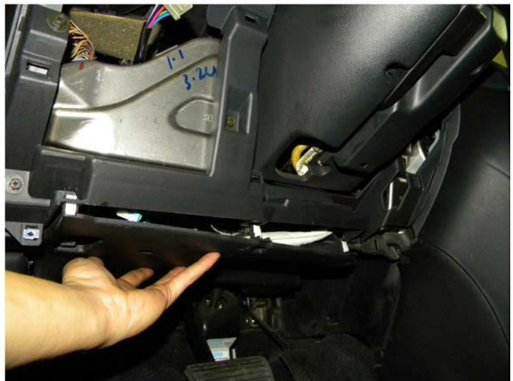
64. Replace the dash panel under the cover
