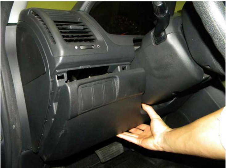
51. Remove the plastic panel
