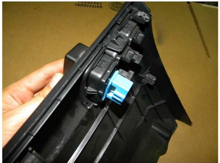
56. Place the fog light switch into the plastic panel
