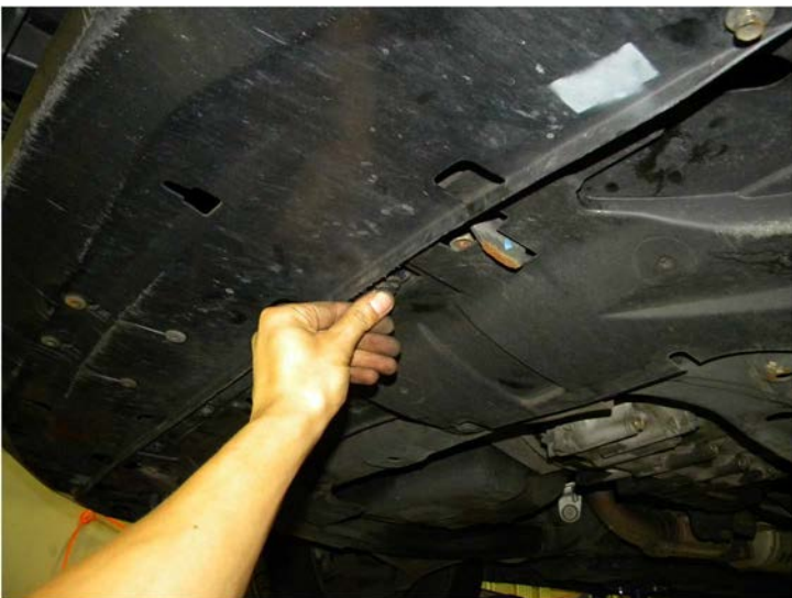
45. Replace the (6) plastic clips
