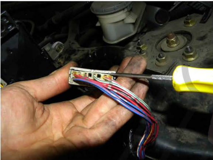
25. Remove the clip from the (14) pin connector
