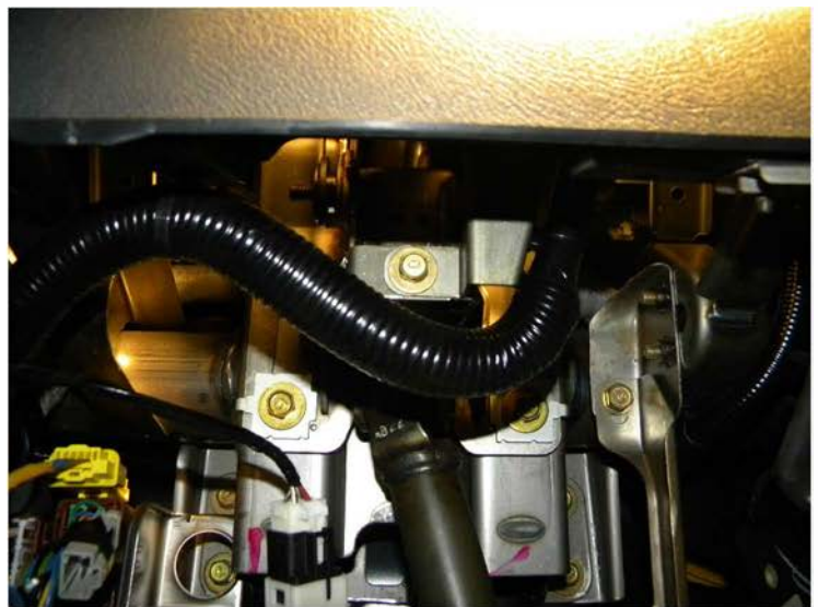
58. 10mm bolt under the dach
