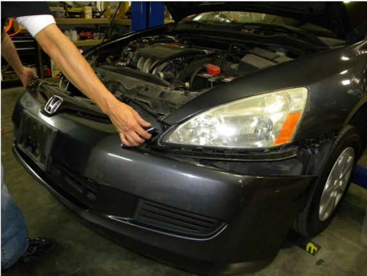
7. Remove the front bumper
