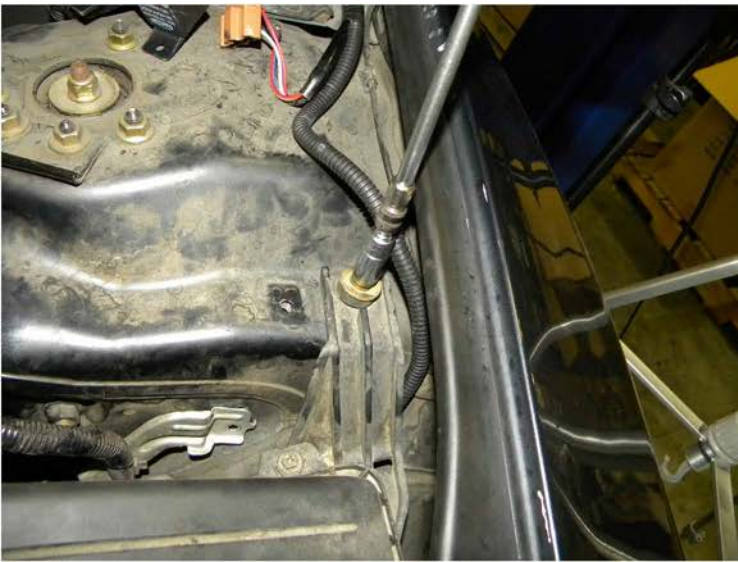
35. Tighten the 10mm bolt on the airbox
