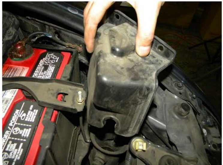
16. Remove the air duct cover
