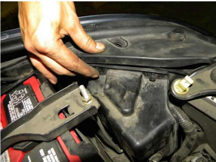
39. Replace the air duct cover, (2 clips)
