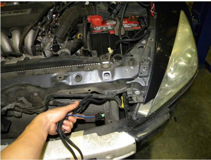
17. Run the fog light harness through the front bulkhead along the factory harness
