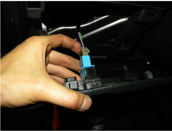
65. Connect the switch to the harness
