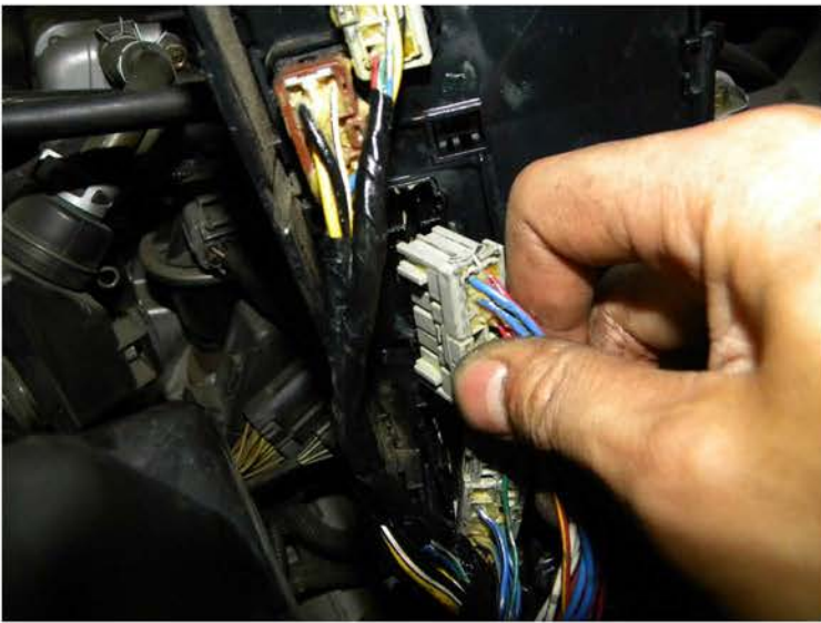
23. Remove the (14) pin connector
