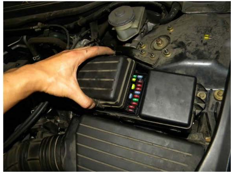
48. Replace the fuse box cover
