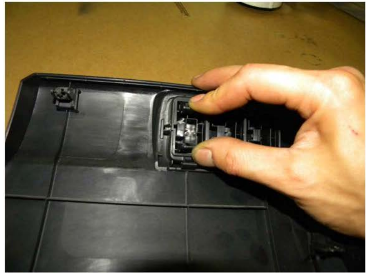
54. Unclip the switch hole cover
