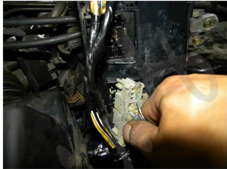
24. Remove the (20) pin connector
