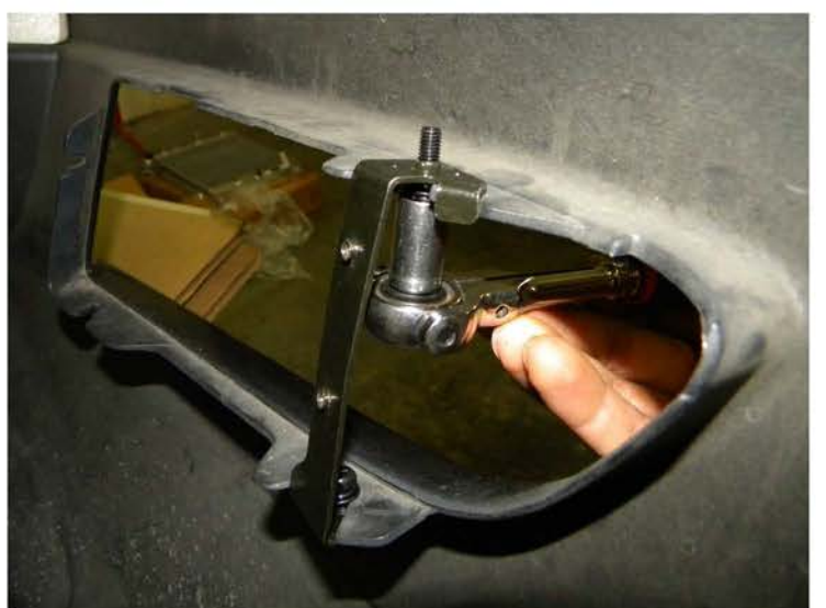
10. Install the fog light outer bracket. (the (2) 10mm bolts)
