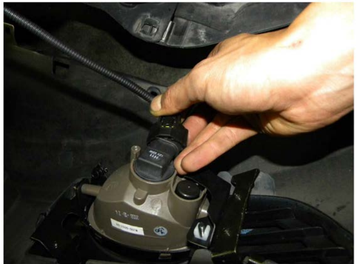
40. Connect the fog lights to the harness
