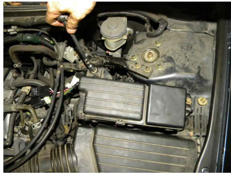
32. Replace the fuse box and tighten the (2) 10mm bolts
