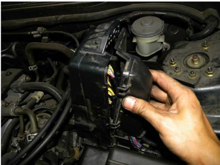
31. Replace the fusebox under cover
