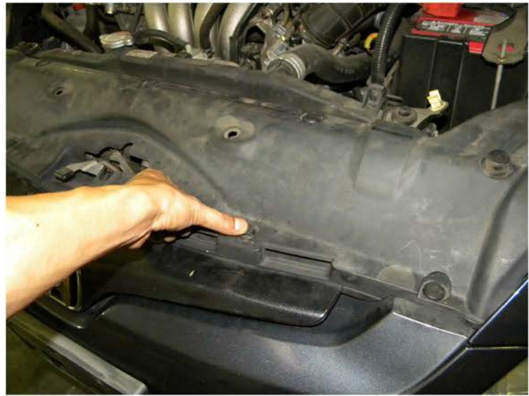
42. Replace the plastic radiator cover
