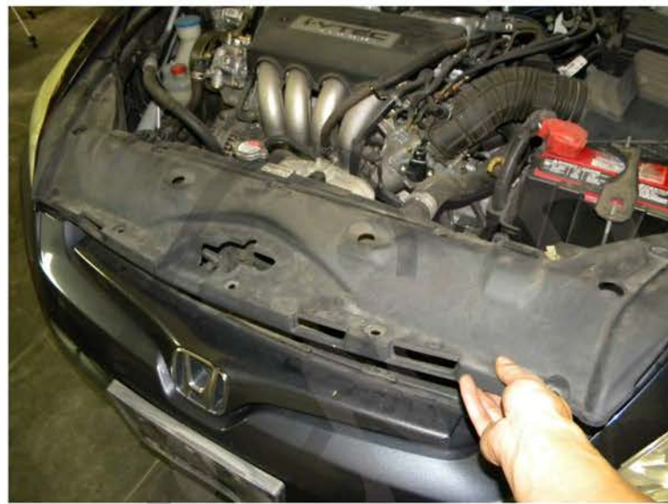
6. Remove the plastic cover
