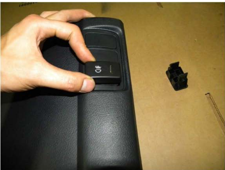
57. Place the fog light switch into the panel
