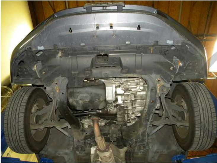
1. (6) clips and (4) 10mm bolt locations
