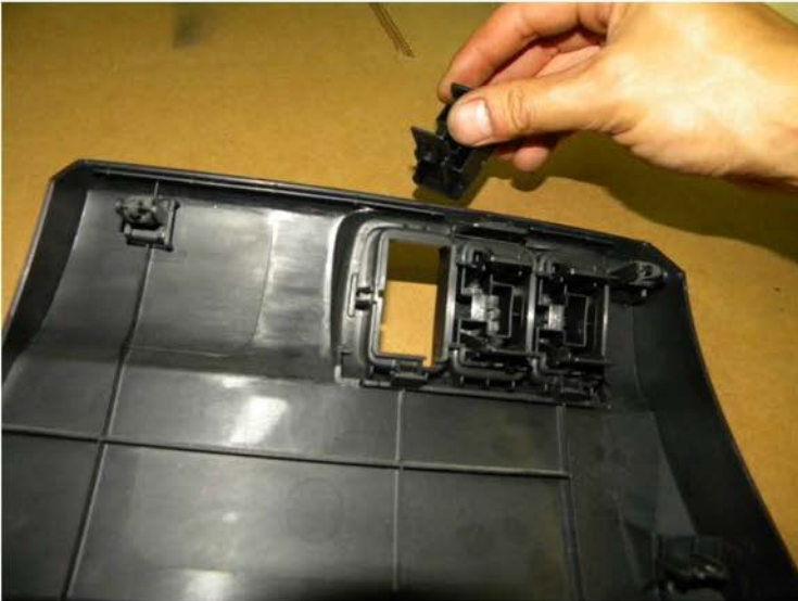
55. Unclip switch hole cover
