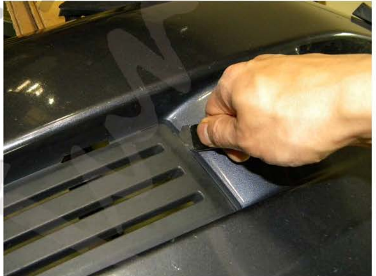
8. Cut out fog light hole
