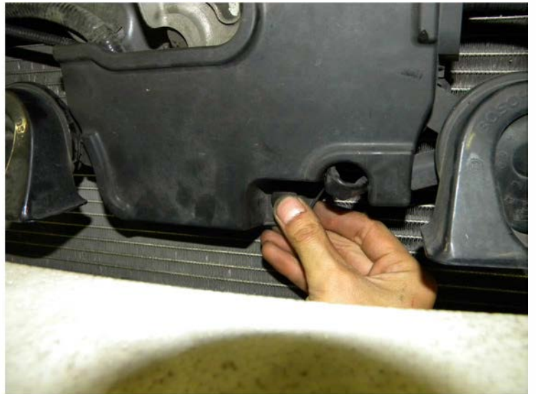
38. Replace the hood latch cover
