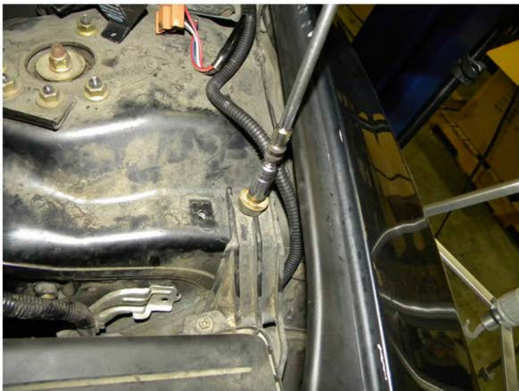
33. Loosen the 10mm bolt from the airbox
