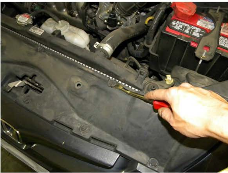
5. Remove the (10) plastic clips
