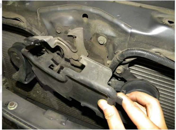
14. Remove the hood latch cover
