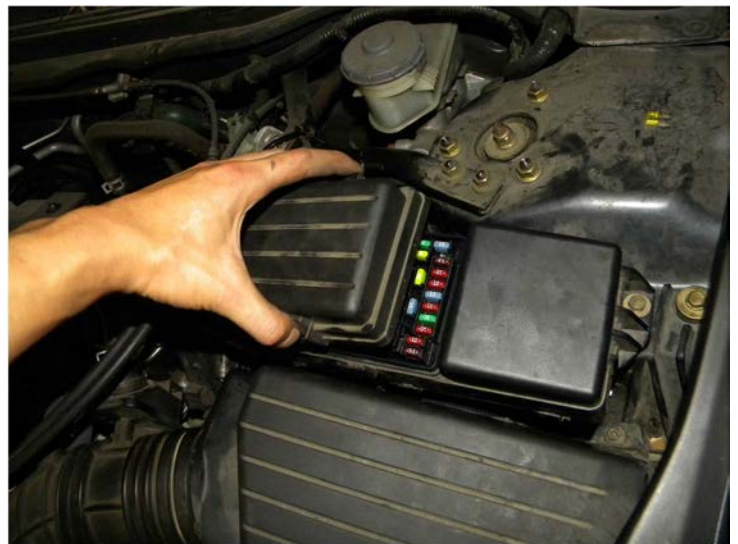
46. Open the fuse box
