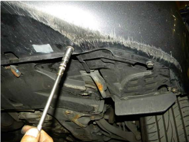
49. Tighten the (4) 10mm bolts
