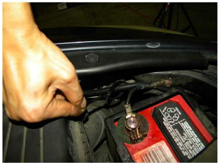
36. Zip tie fog light harness to factory harness
