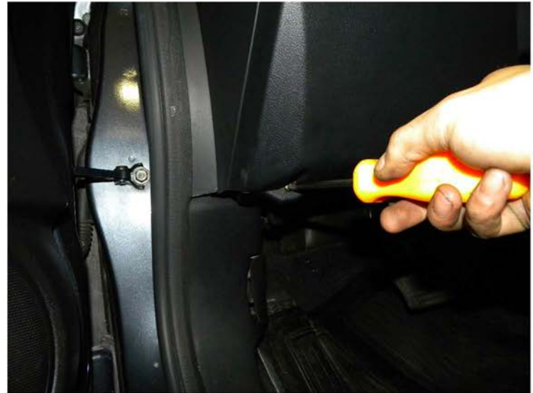
50. Remove the phillips head screw
