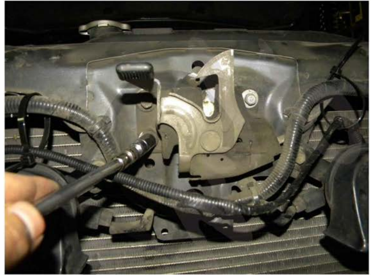
18. Remove the 10mm bolt front hood latch
