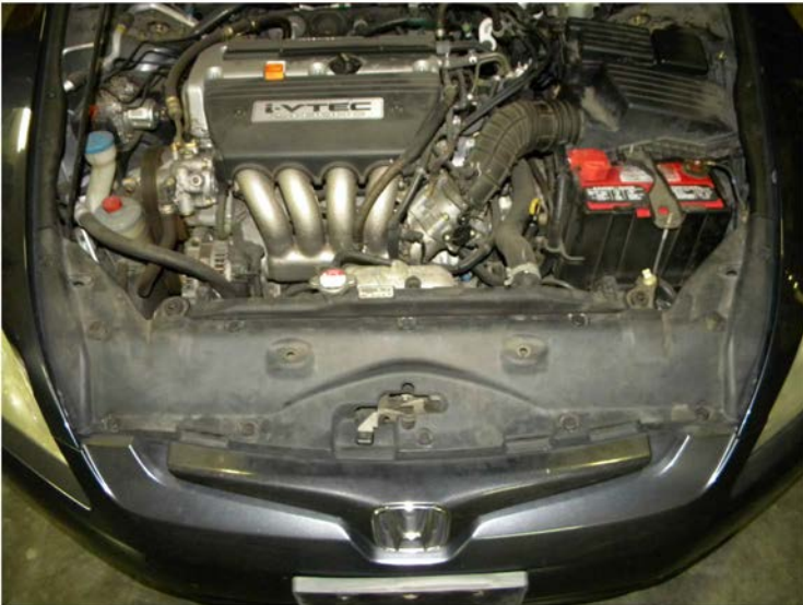
42. Replace the (10) plastic clips
