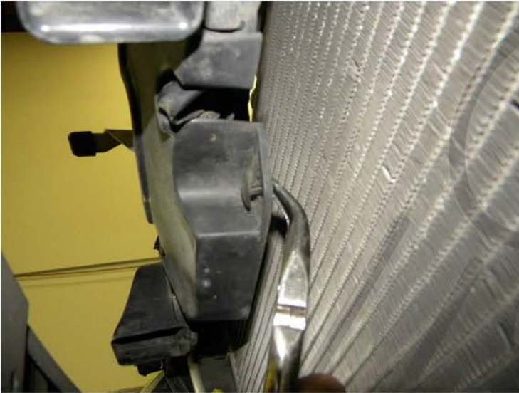
13. Remove the plastic clip from the hood latch cover
