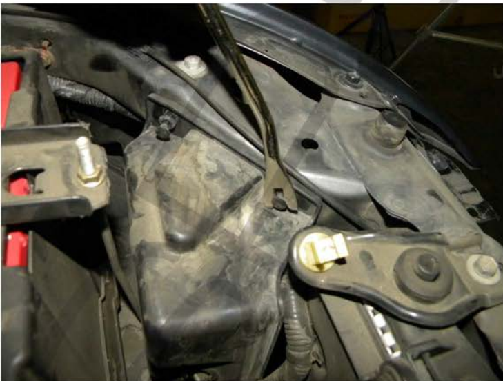
15. Remove the (2) plastic clips from the air duct cover
