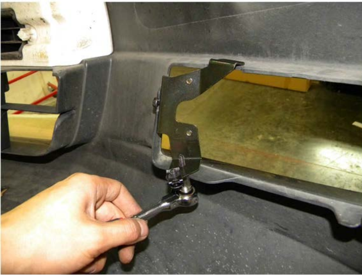
11. Install the fog light outer bracket the (2) 10mm bolts
