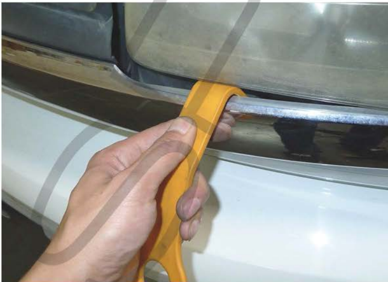
3. Release the front grill retaining clips
