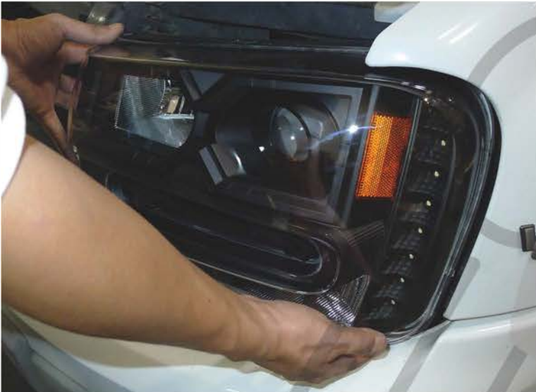
13. Place the new headlight into the position
