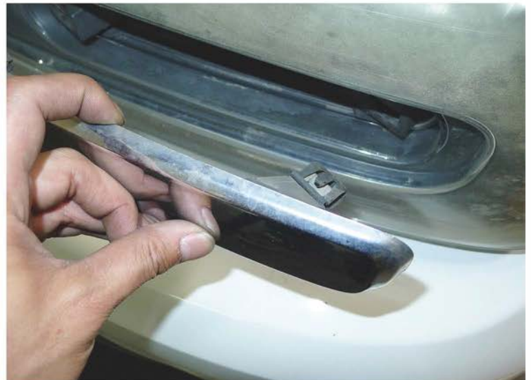
4. Release the front grill retaining clips
