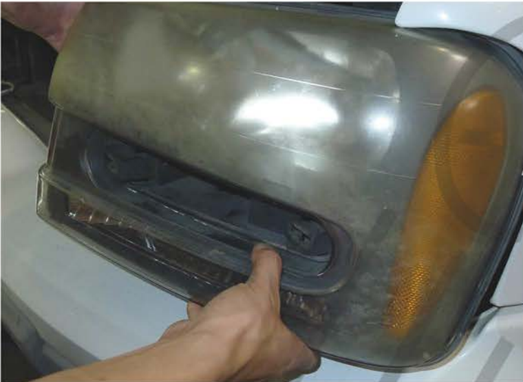
7. Remove the factory headlight
