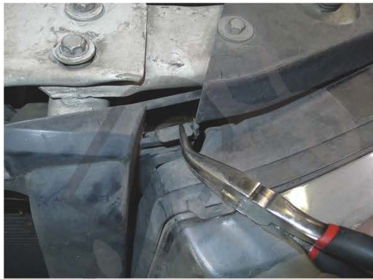
6. Release the (2) headlight retainers by the pulling upwards
