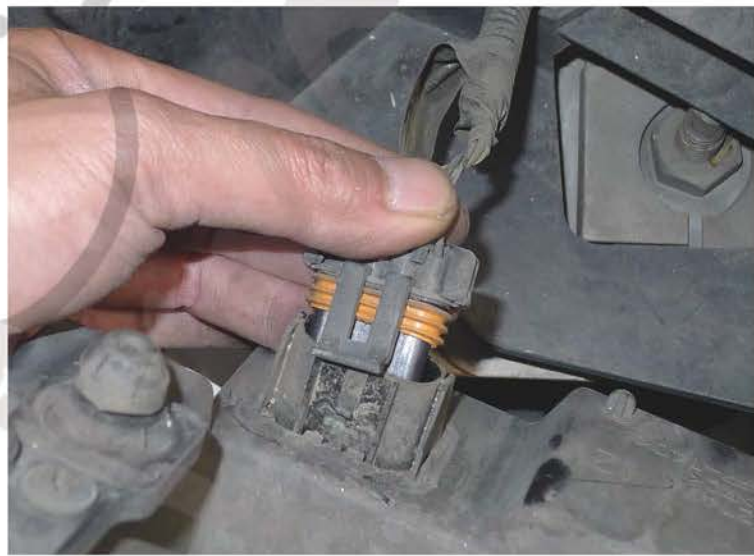
8. Disconnect the headlight harness
