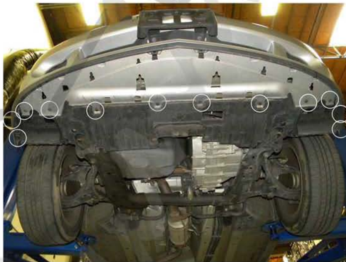
2. Remove eight clips and four screws
