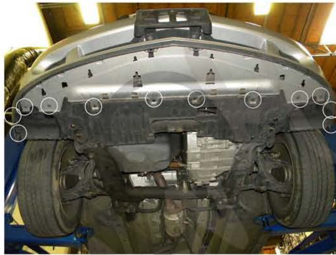
18. Install eight clips and four screws
