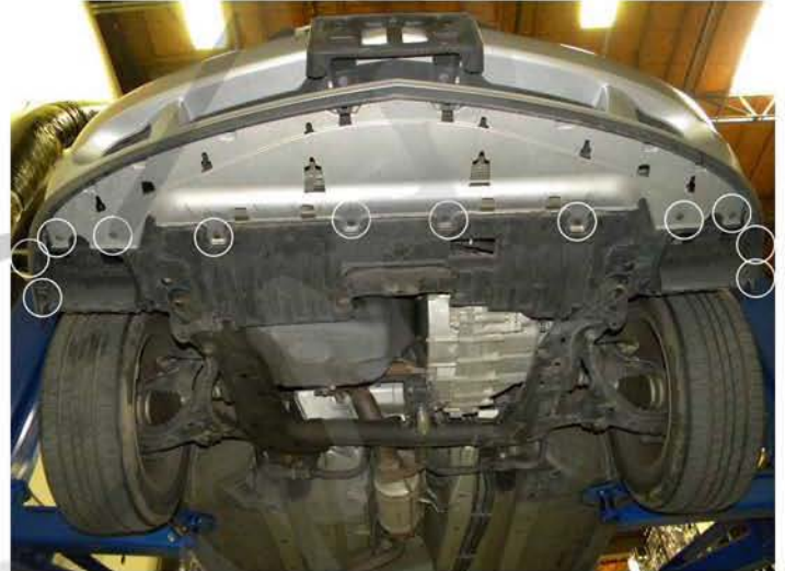
2. Remove eight clips and four screws
