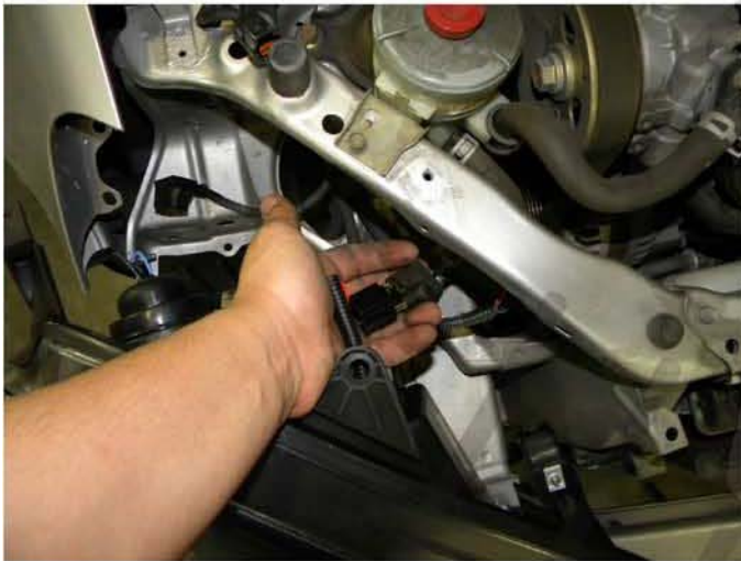
13. Connect all the headlight connectors Please see the "Halo and L.E.D installation instructions" If your headlights don't have HALO or L.E.D. You can skip this step
