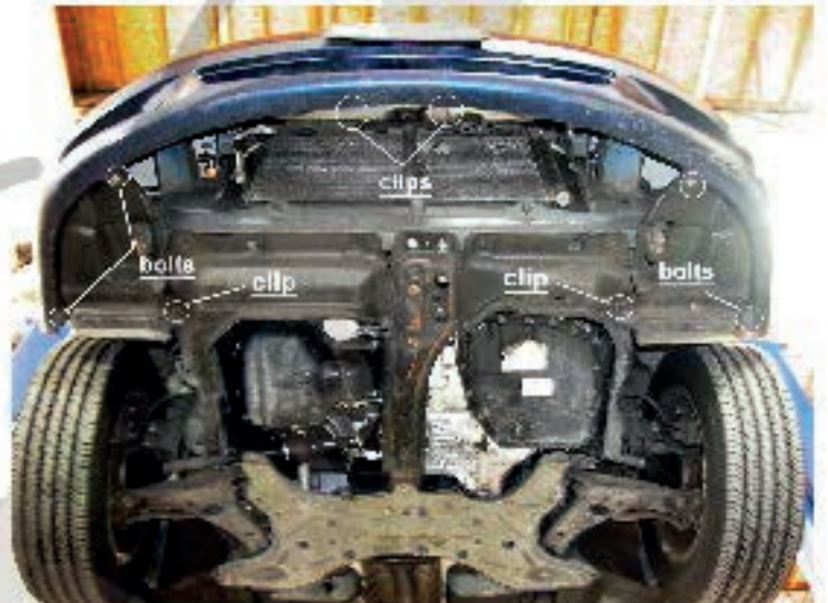
2. Remove the bolts and clips from the front bumper
