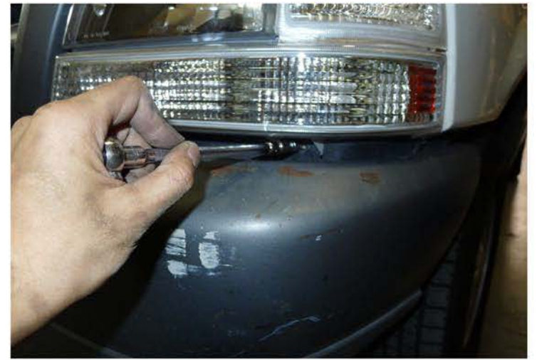
10. Tighten the (2) .25 in. screws
