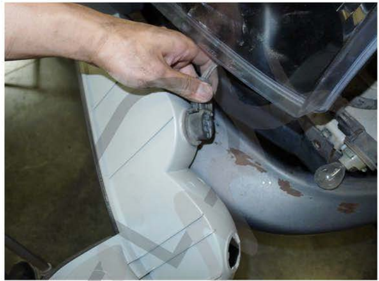
6. Place the light sockets in the new corner-bumper light
