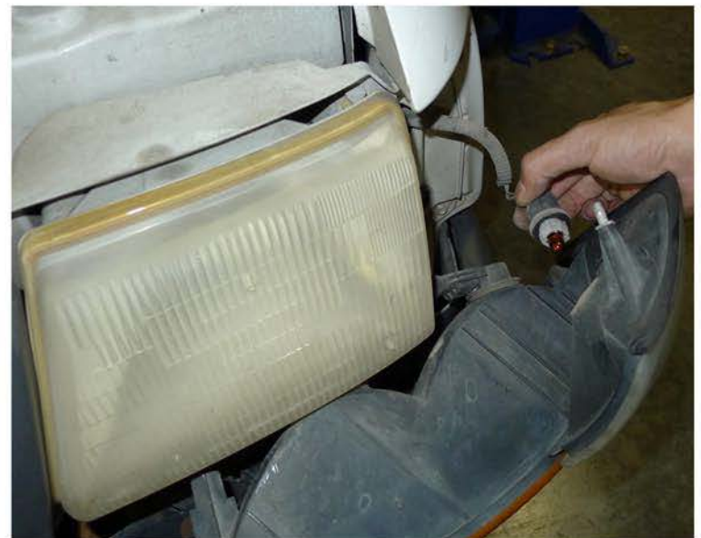
4. Disconnect the light sockets
