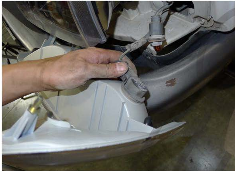
7. Place the light sockets in the new corner-bumper light
