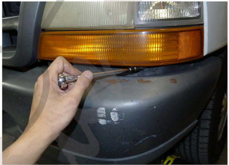
2. Remove the (2) .25 in. screws
