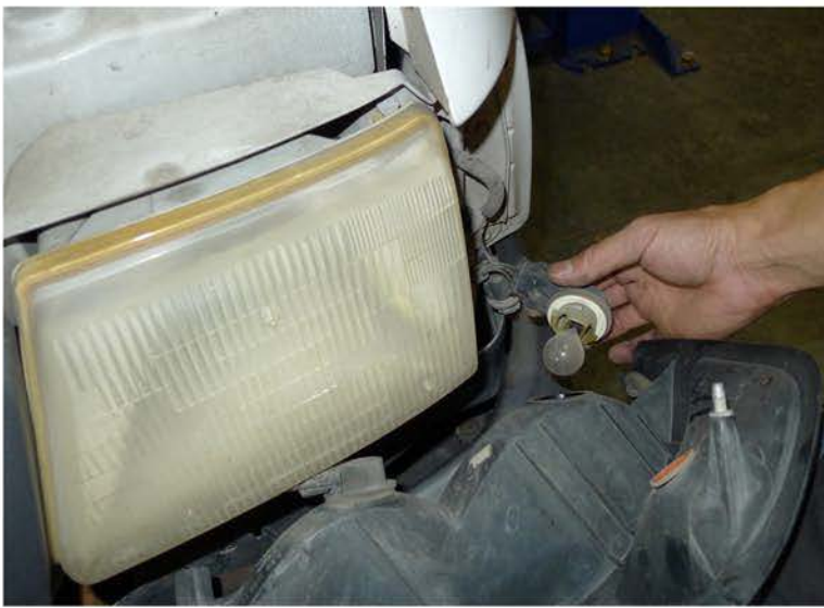
5. Disconnect the light sockets
