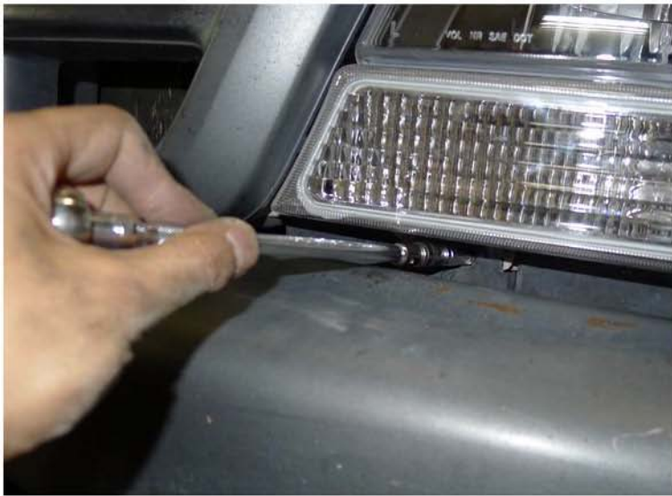
11. Tighten the (2) 1/25 in. screws
