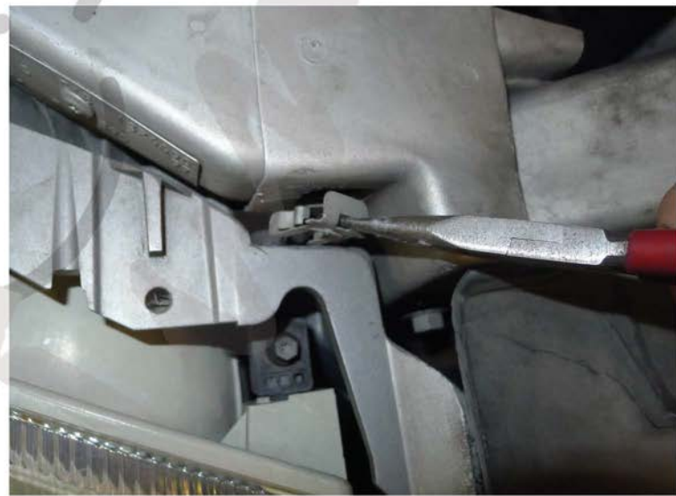
9. Remove the (2) metal clips
