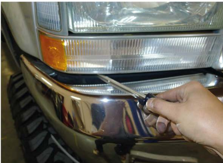
3. Remove the (2) phillips head screws
