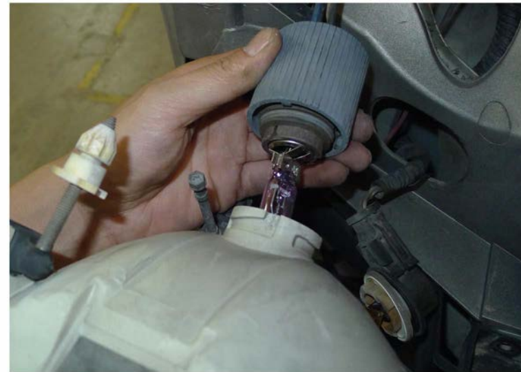
10. Remove the headlight bulb and harness
