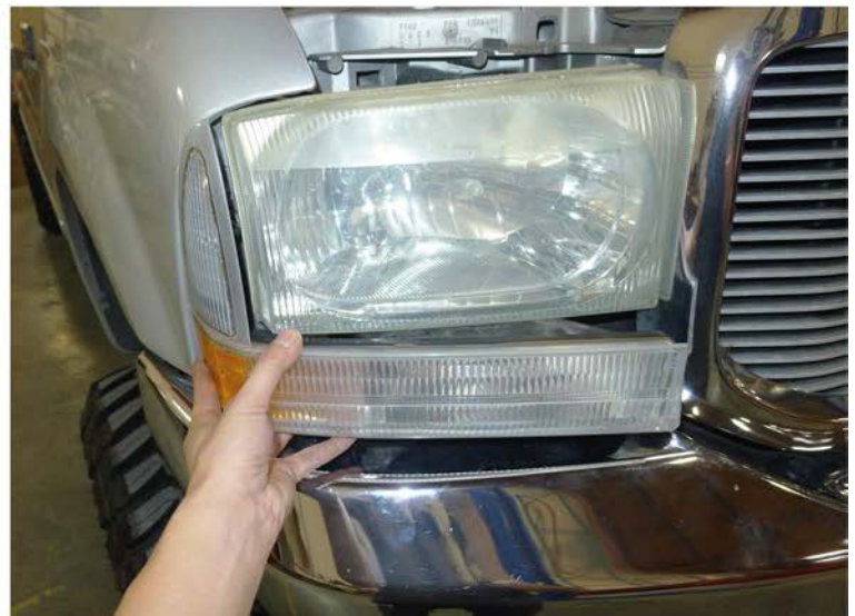
4. Remove the bumper corner light
