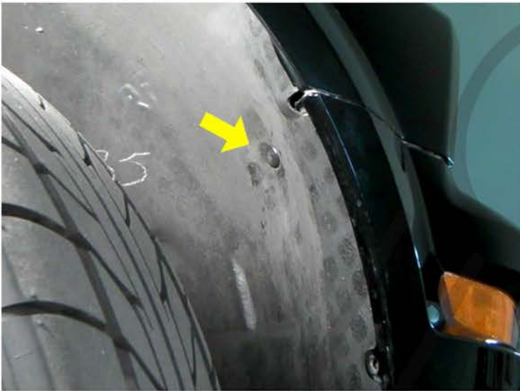
13. Install one clip under the wheel well
