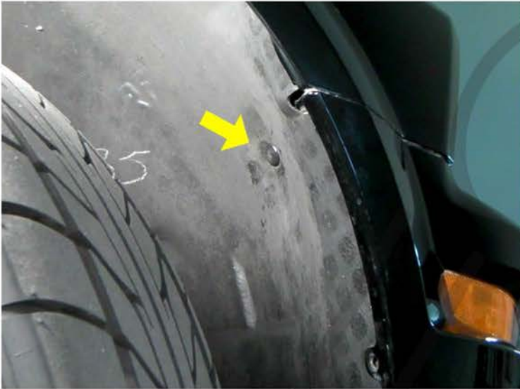
13. Install one clip under the wheel well
