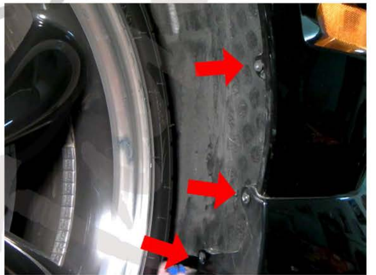
14. Install three bolts under the wheel well
