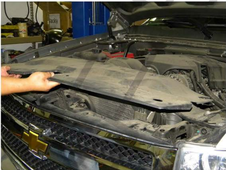
3. Remove the plastic radiator cover
