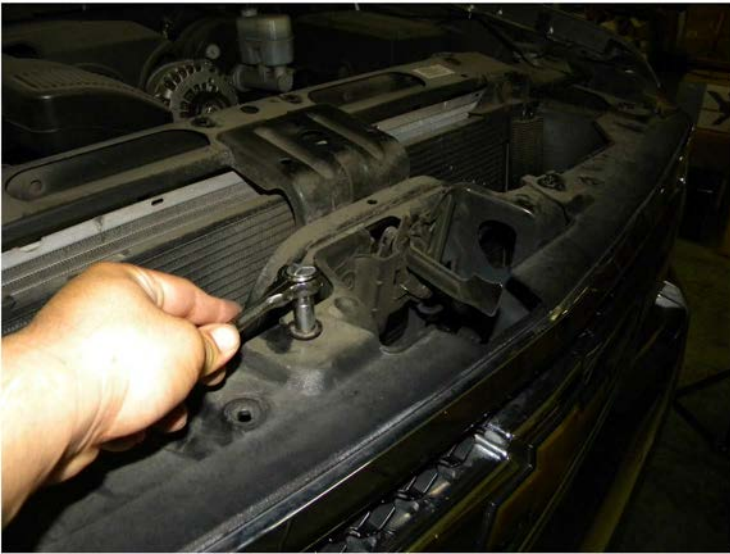
5. Remove the (4) 10mm bolts
