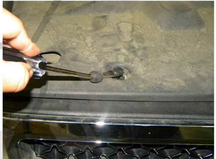
2. Remove the (8) plastic clips
