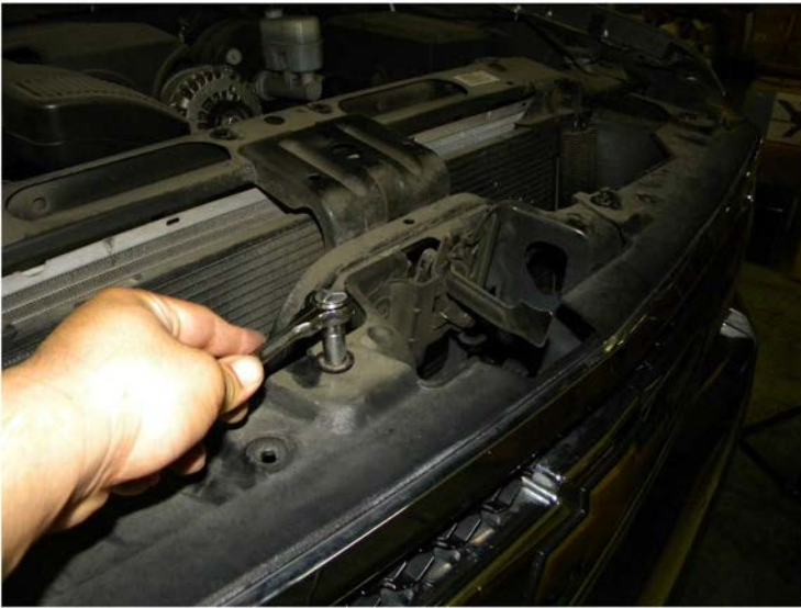
5. Remove the (4) 10mm bolts
