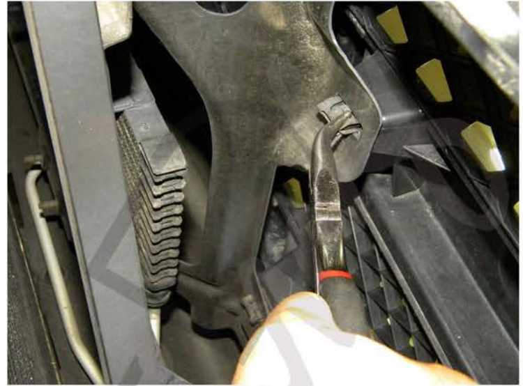
6. Unclip the metal clips from the rear of the front grill
