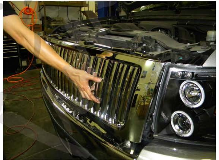
8. Place new grill in the stock location
