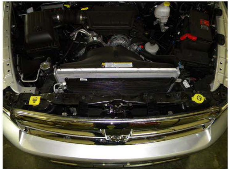
4. 4 10mm bolts location
