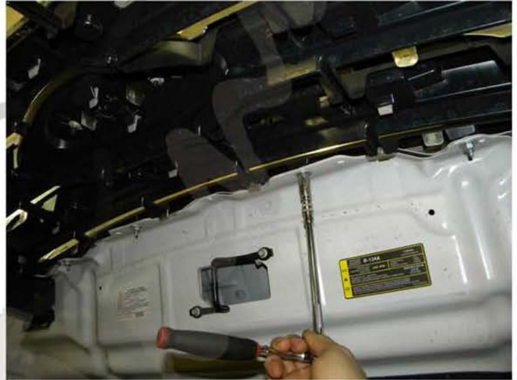
2. Remove the (6) 10mm nuts
