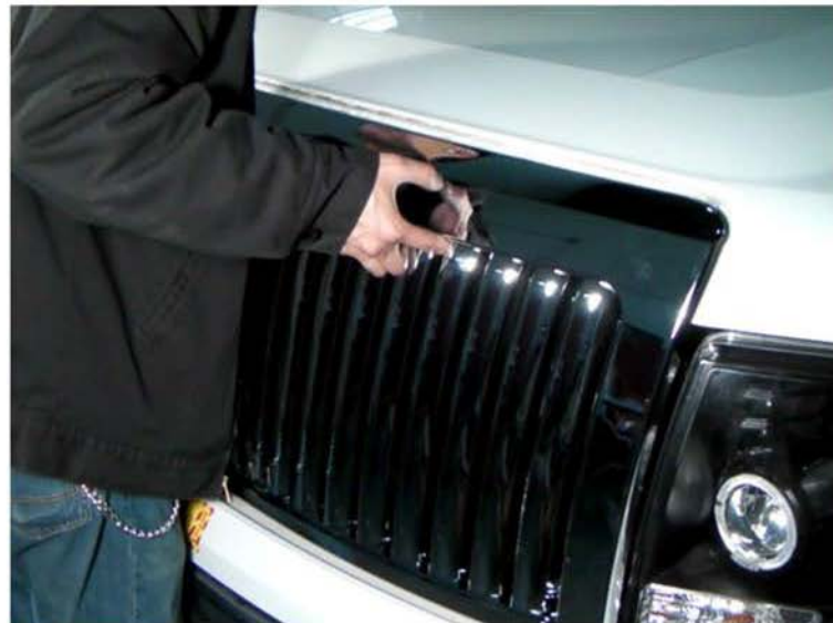
10. Place the new grill in the stock location
