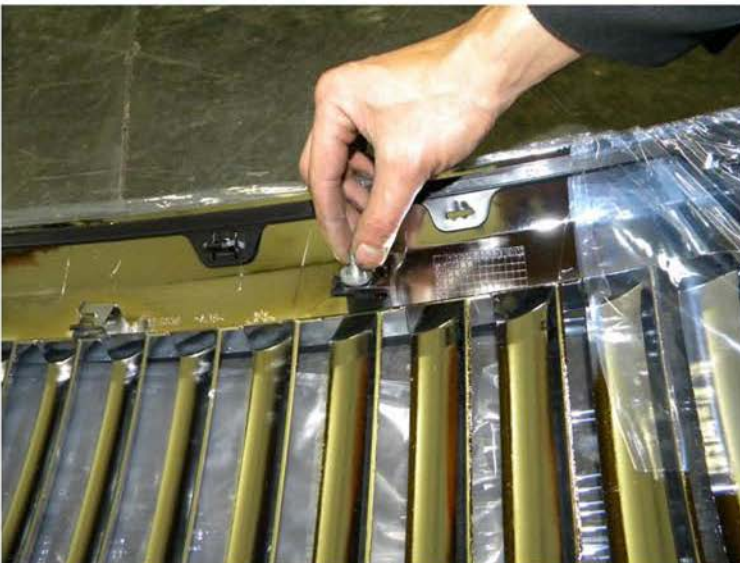
9. Place the (6) bolts in the new grill
