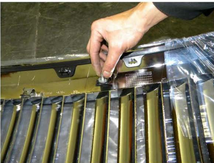
9. Place the (6) bolts in the new grill
