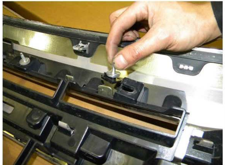
8. Remove the (6) bolts from the stock grill
