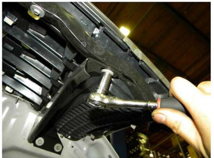
4. Remove the (2) 10mm bolts
