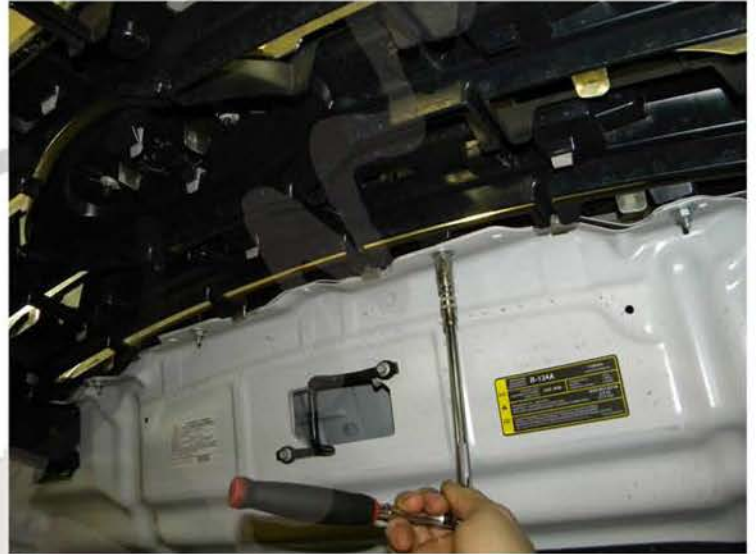
2. Remove the (6) 10mm nuts
