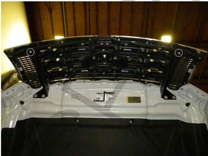
3. (2) 10mm bolts location
