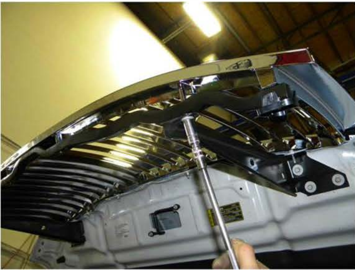
11. Tighten the (2) 10mm bolts
