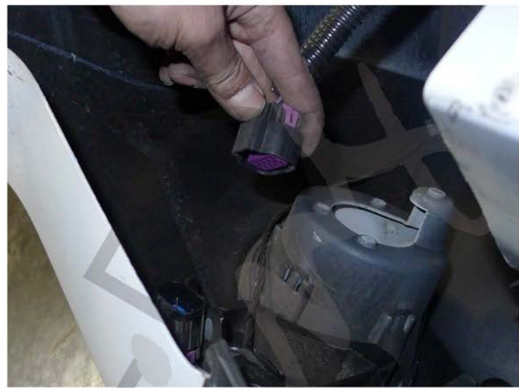
30. Connect the electric harness
