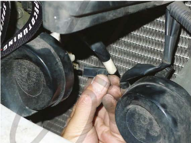
9. Disconnect the stock horns
