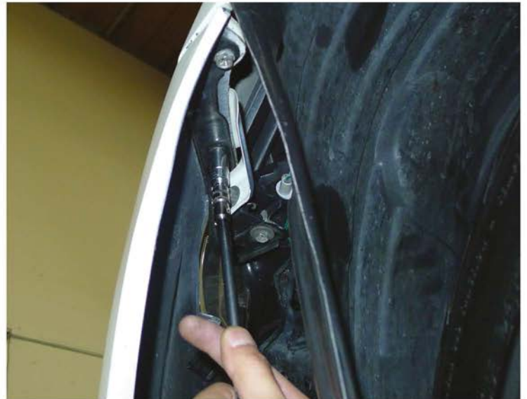
4. Remove the (2) 10mm bolts
