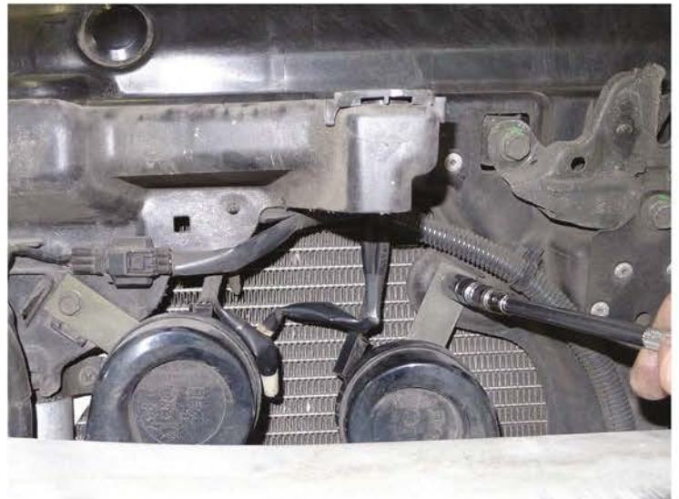
10. Remove the stock horns
