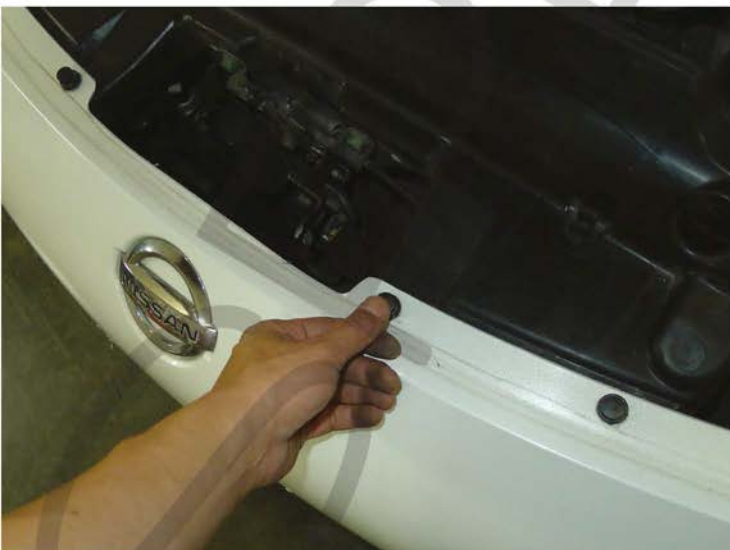
21. Replace the (6) plastic clips
