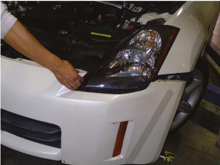
7. Remove the front bumper
