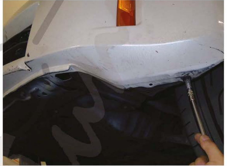
2. Remove the (8) 8mm bolts
