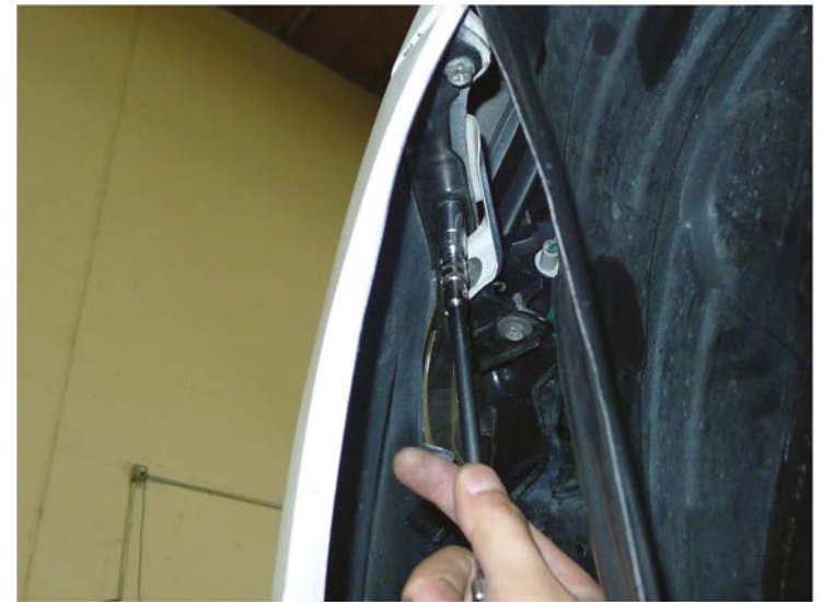
22. Tighten the (2) 10mm bolts
