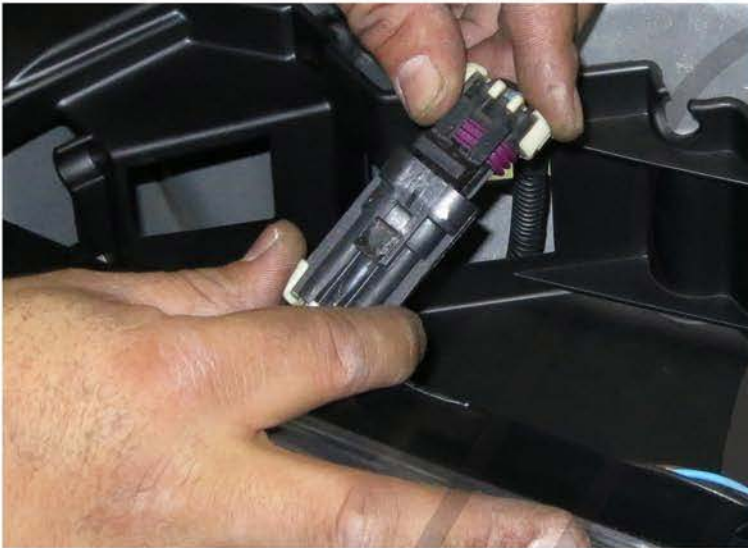
7. Connect the bumper light harness
