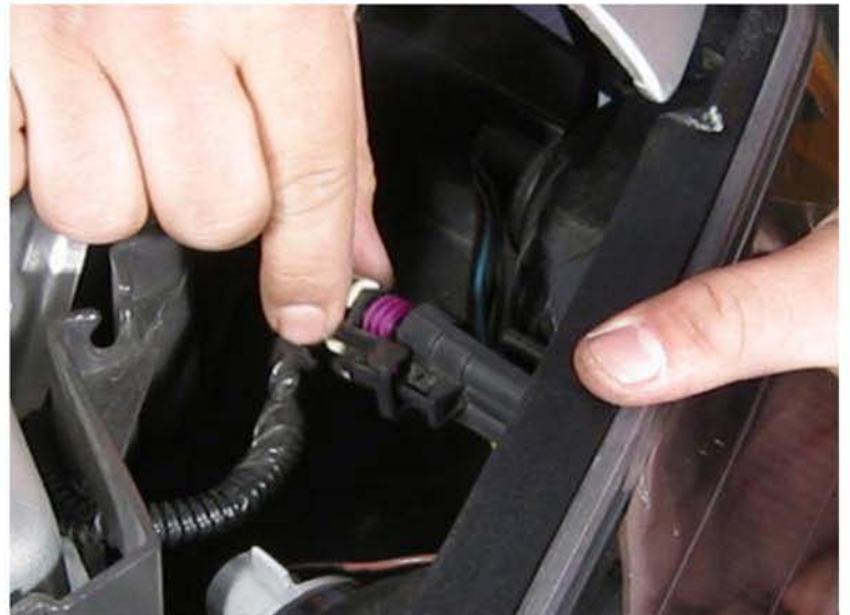
4. Disconnect the bumper light harness
