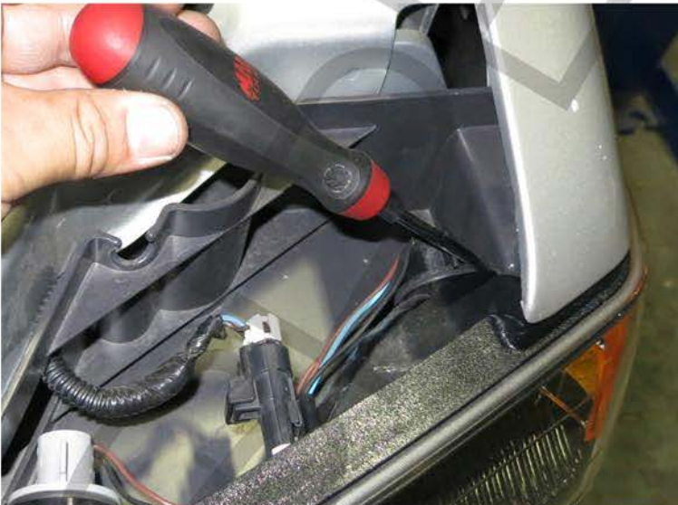
3.. Release the bumper light retaining clip
