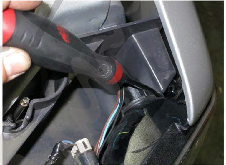
2. Release the retaining clip
