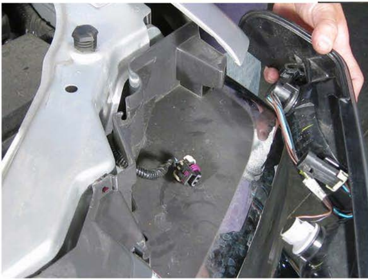
5. Remove the bumper light
