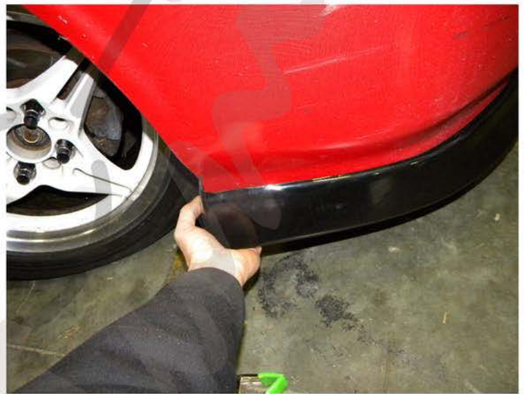
2. Tug firmly and position the chin spoiler on the other side of the front bumper
