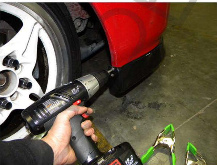
3. Fasten the chin spoiler with the (2) self tapping screws
