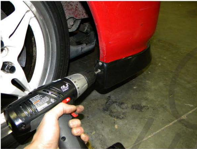
1. Fasten the chin spoiler to the front bumper with (2) self tapping screws
