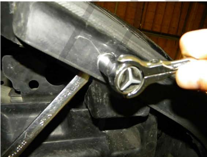
9. Tighten the 14mm nut and the 12mm bolt locate on the bottom end
