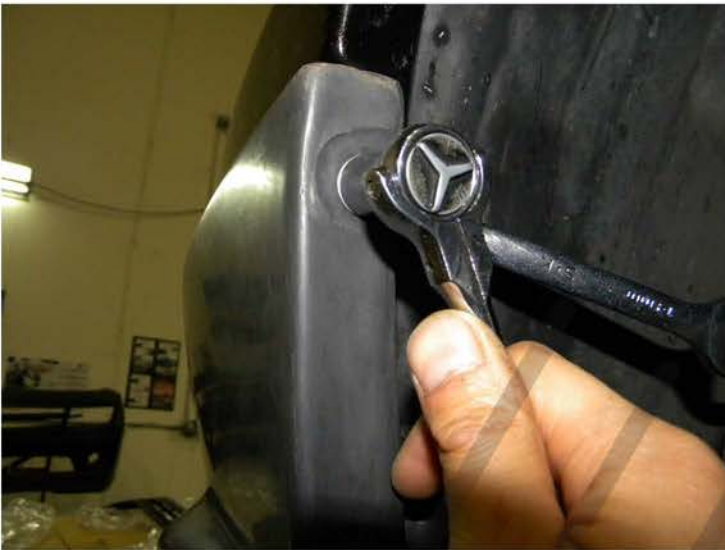
7. Tighten the 14mm nut and the 12mm bolt
